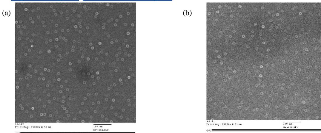
**Figure S1.** TEM image of the wild type TMV-cp in water before (a) and after (b) UV illumination, the dominant species is in disk form.
