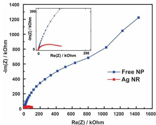
**Figure S6.** Nyquist plot of Ag NR and Free NP recorded at open circuit potential in CO<sub>2</sub> saturated 0.5 M KHCO<sub>3</sub> solution.
