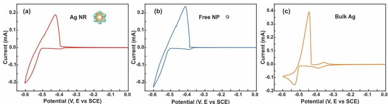
**Figure S2.** Cyclic voltammograms of UPD and bulk deposition of lead in 5 mM Pb(NO<sub>3</sub>)<sub>2</sub>, 10 mM HNO<sub>3</sub> and 10 mM KCl, with a scan rate of 10 mV/s.
