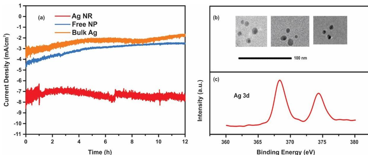
**Figure S8.** Twelve hours durability test at a potential of  $-1.028$  V from Ag NR, Free NP and Bulk Ag (a); post electrolysis characterization of Ag NR by TEM (b) and XPS spectrum (c).
