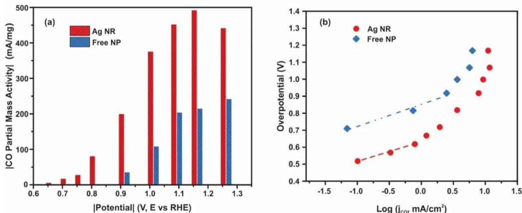
**Figure S4.** CO mass activity of Ag NR and Free NP under different applied potentials (a); Tafel plots of prepared Ag NR and Free N
