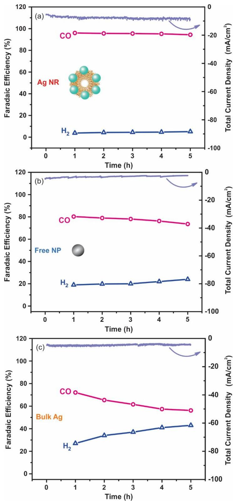
**Figure S7.** Five hours durability test at a potential of -1.028 V from Ag NR (a); Free NP (b); and Bulk Ag (c). FEs of CO and H<sub>2</sub> (left axis) versus time and total current densities (right axis) versus time.
