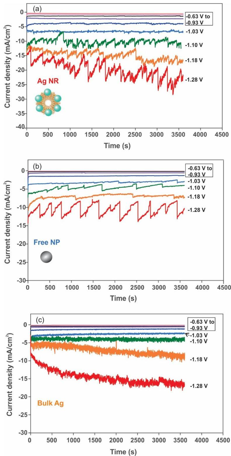
**Figure S3.** Current densities over time at different applied potentials of Ag NR (a); Free NP (b); and bulk Ag (c).
