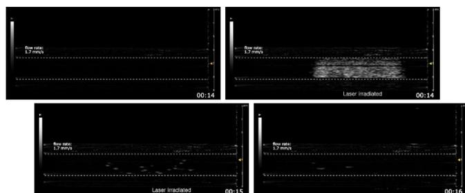
**Movie S4.** B-mode ultrasound imaging of  $N_2$  generation under the laminar flow condition. Laminar flow ( $1.16 \pm 0.17$  mm/s) was created with a syringe pump (200  $\mu$ l/min) in a tube (ID = 1.6 mm). (AVI)
