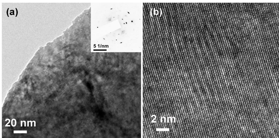
**Figure S3.** (a) The TEM image of  $\text{Cu}_{0.92}\text{Cd}_{0.08}\text{FeS}_2$  with SAED pattern, and (b) the corresponding HRTEM image.
