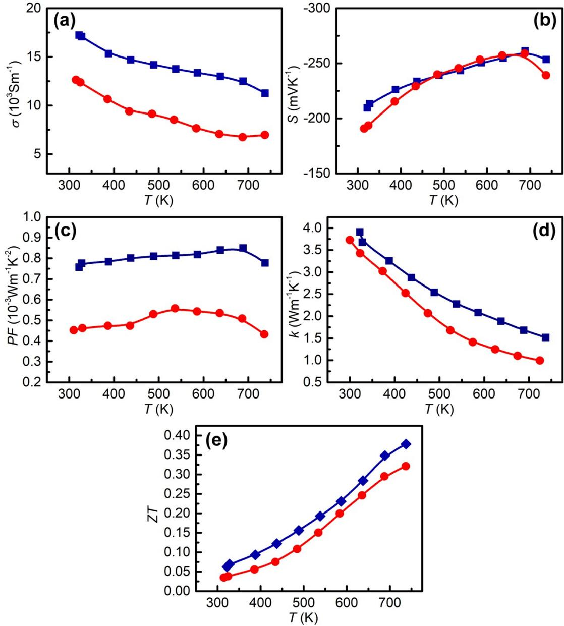
**Figure S8.** The (a) electrical conductivity ( $\sigma$ ), (b) Seebeck coefficient ( $S$ ), (c) power factor ( $PF$ ), (d) electronic thermal conductivity ( $k$ ), and (e) figure of merit ( $ZT$ ) of the  $\text{Cu}_{0.9}\text{Cd}_{0.1}\text{FeS}_2$  (red circulars) and DI- $\text{Cu}_{0.9}\text{Cd}_{0.1}\text{FeS}_2$  (blue squares) samples.
