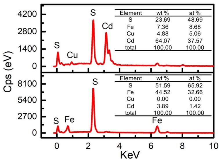
**Figure S1.** EDS results of (a) CdS precipitates (white area) and (b) the  $\text{FeS}_2$  precipitates (gray area) in Figure 2. (d)
