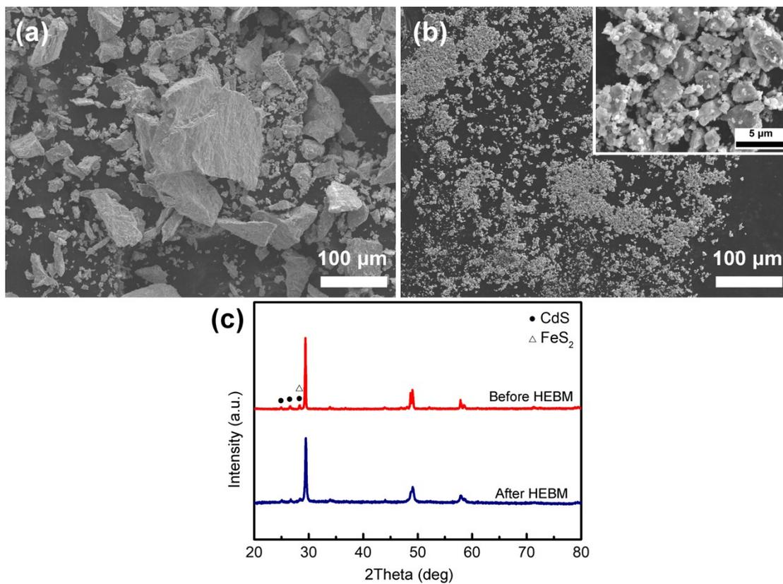
**Figure S2.** The SEM images of the  $\text{Cu}_{0.92}\text{Cd}_{0.08}\text{FeS}_2$  powders (a) before and (b) after HEBM, and (c) the corresponding XRD patterns.
