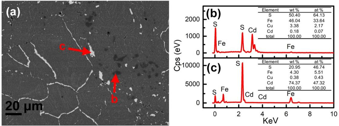
**Figure S4.** The BSE images of  $\text{Cu}_{0.92}\text{Cd}_{0.08}\text{FeS}_2$  sample prepared by quenching and annealing without high-energy ball milling process (a), the EDS result of b point (b) and c point (c).
