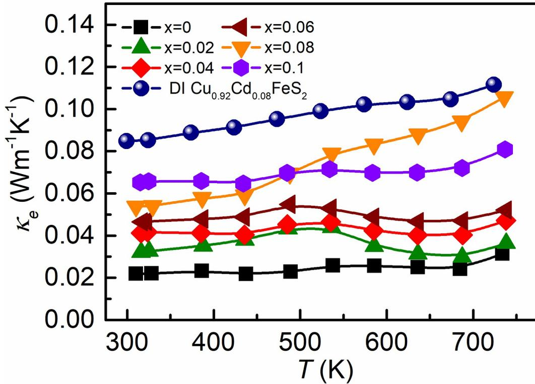
**Figure S5.** The electron thermal conductivity ( $k_e$ ) of  $\text{Cu}_{0.92}\text{Cd}_{0.08}\text{FeS}_2$  (red circles) and defects integrated  $\text{Cu}_{0.92}\text{Cd}_{0.08}\text{FeS}_2$  (blue squares) samples.
