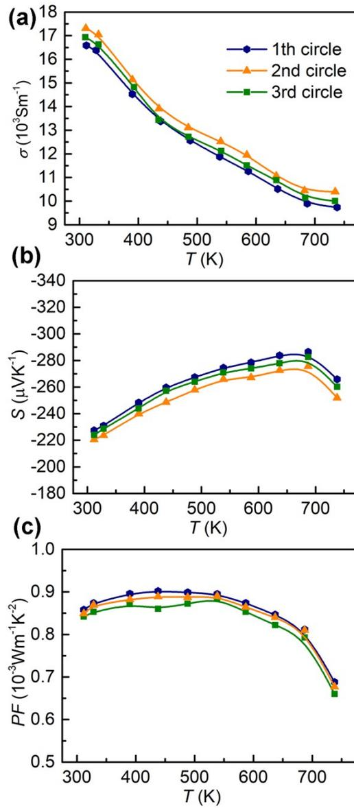
**Figure S7.** The (a) electrical conductivity ( $\sigma$ ), (b) Seebeck coefficient ( $S$ ), (c) power factor ( $PF$ ) of cycle testing
