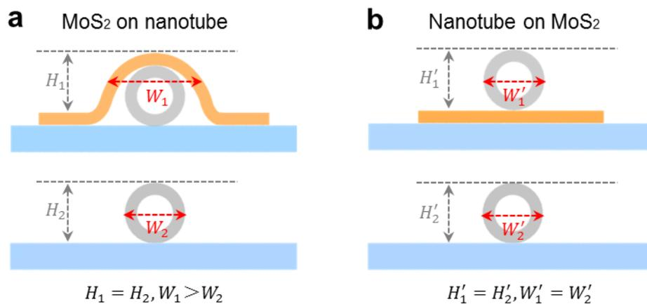
**Supplementary Fig. 3. Schematic diagram of two possible stacking geometries in nanotube-MoS<sub>2</sub> hybrids. (a)** MoS<sub>2</sub> climbing over nanotube geometry. Height and width illustration of the same nanotube hybridized with MoS<sub>2</sub> monolayer (top panel) and on bare substrate (bottom panel). **(b)** Nanotube sitting on MoS<sub>2</sub> geometry. Situations for the same nanotube on MoS<sub>2</sub> (top panel) and on bare substrate (bottom panel) are identical.
