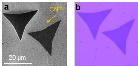
**Supplementary Fig. 2.** (a) Scanning electron microscope (SEM) image and (b) the corresponding optical image of a nanotube-MoS<sub>2</sub> monolayer hybrid structure with clean interface. Nanotube outline cannot be seen in the optical image, but it shows a uniform MoS<sub>2</sub> monolayer contrast on and off nanotube.
