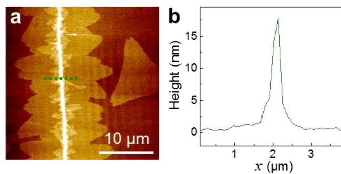
**Supplementary Fig. 1.** (a) Atomic force microscope (AFM) image of nanotube-multilayer MoS<sub>2</sub> hybrids with dirty interface. (b) AFM cross-sectional profile along the green line indicated in (a) shows that the height of MoS<sub>2</sub> along nanotube exceeds 15 nm, and confirms the multi-layer MoS<sub>2</sub> structure.
