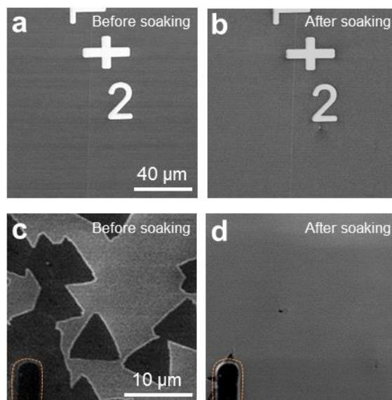
**Supplementary Fig. 4. (a-b)** SEM images of a nanotube on 300 nm SiO<sub>2</sub>/Si substrate before (a) and after (b) soaking in water. **(c-d)** Optical images of MoS<sub>2</sub> samples on 300 nm SiO<sub>2</sub>/Si substrate before (c) and after (d) soaking in water. Pure MoS<sub>2</sub> can be easily washed out by water immersion but nanotube cannot.
