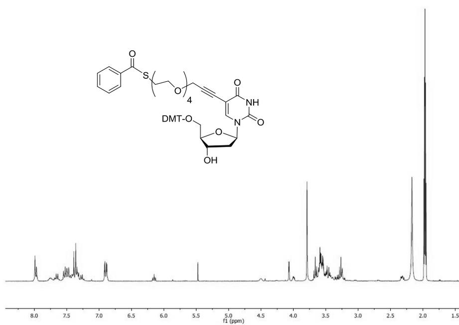
**Figure S7.**  $^1\text{H}$ -NMR spectrum of compound **14** (300 MHz,  $\text{CD}_3\text{CN}$ ).
