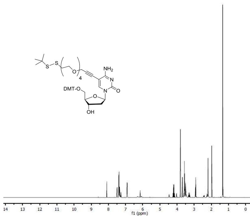
**Figure S4.** <sup>1</sup>H-NMR spectrum of compound **7** (500 MHz, CD<sub>3</sub>CN).
