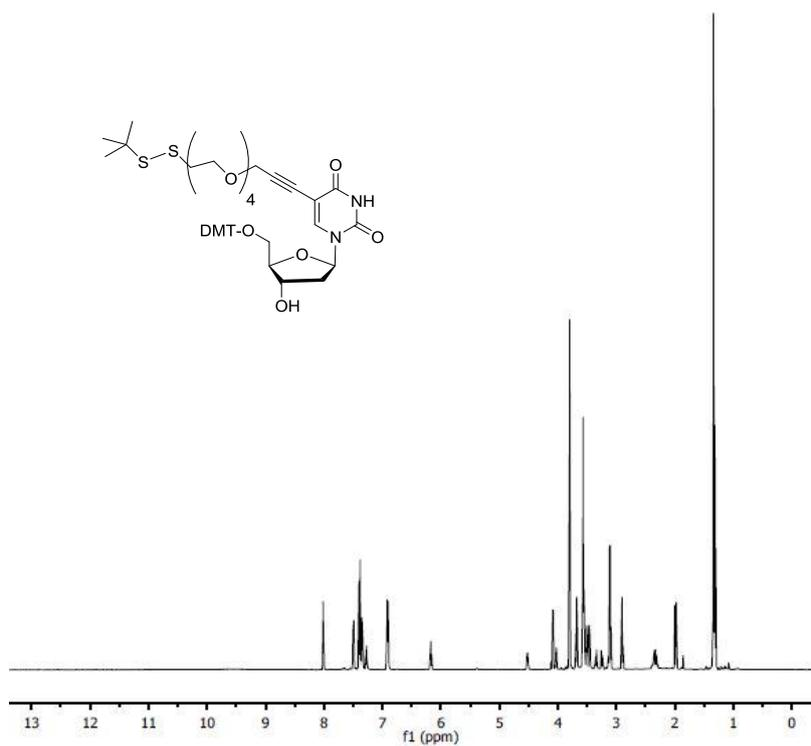
**Figure S8.** <sup>1</sup>H-NMR spectrum of compound **15** (500 MHz, CD<sub>3</sub>CN).
