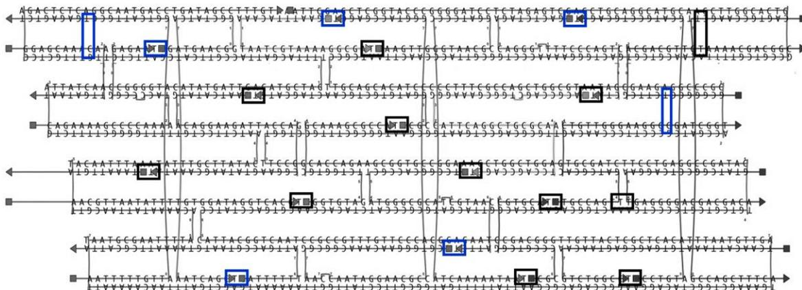
**Figure S13.** The caDNANO-based design of motif IV. Overhangs on both sides of the origami, consisting of stretches of oligo-dT, were used to avoid aggregation of the nanostructures in solution. Highlighted in blue are disulfide links between nucleotide combinations U/C, disulfides between U/U bases (shown as T/T in caDNANO) are highlighted in black.
