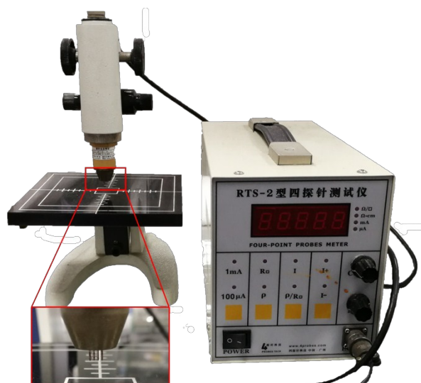
Fig. S4. A photo of the four-point probe station. The inset is the zoomed view of the four points with 1 mm interval space.
