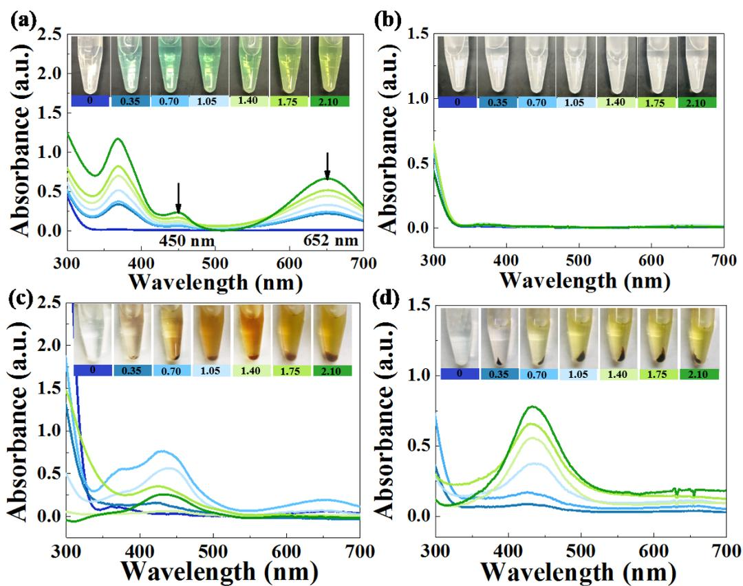
**Figure S3.** (a) UV-Vis spectra of TMB (0.5 mM) oxidation by bare CeO<sub>2</sub> for 12 h. (b) UV-Vis spectra of the supernatant after centrifugation and adding phosphate. (c) UV-Vis spectra of TMB (0.5 mM) oxidation by 5 mM F-/CeO<sub>2</sub> for 12 h. (d) UV-Vis of the supernatant after centrifugation and adding phosphate (500 mM, 15 μL). The concentration of CeO<sub>2</sub> are 0, 0.35, 0.70, 1.05, 1.40, 1.75, 2.1 μM respectively at pH 4 (acetate buffer, 25 mM).
