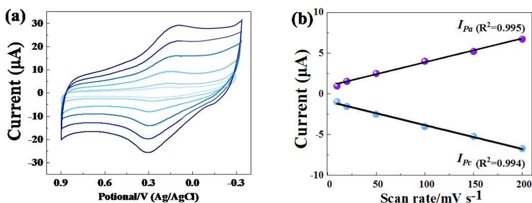
**Figure S4.** (a) The CV curves of the F<sup>-</sup>/CeO<sub>2</sub> GCE in 500 mM acetate buffer (pH 4.0) at different scan rates. Scan rates (from inside out) were 10, 20, 50, 100, 150, 200 mV s<sup>-1</sup>. (b) The anodic and cathodic peak current as function of scan rate. In all these measurements, dissolved oxygen in solution was removed by bubbling in nitrogen for 30 min.
