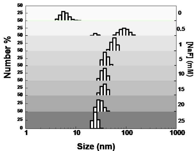
**Figure S1.** The hydrodynamic diameters of the CeO<sub>2</sub> NPs (200 µg mL<sup>-1</sup>) as a function of F<sup>-</sup> concentration at pH 4 (acetate buffer, 25 mM) measured by DLS.
