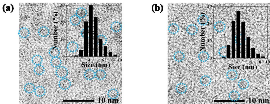
**Figure S2.** The HRTEM micrographs and hydrodynamic diameters of the CeO<sub>2</sub> NPs (200 µg mL<sup>-1</sup>) (a) before and (b) after reaction with 5 mM F<sup>-</sup> and 0.5 mM ABTS at pH 4 (acetate buffer, 25 mM). After reaction, the precipitates were washed 3 times after adding phosphate (500 mM, 5 µL) to desorb the oxidation product of ABTS and F<sup>-</sup> before drying on TEM grids and imaging.
