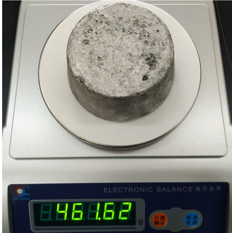
Fig. S6. Photograph showing the \text{Al}_{95}\text{Bi}_x\text{Sn}_y alloy ingot with a mass of more than 460 g. The present strategy could be easily scaled up.
