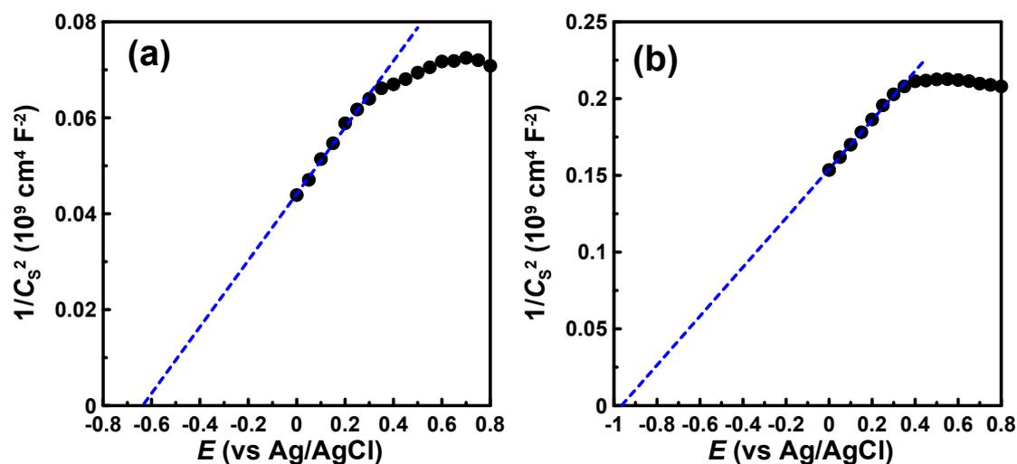
Figure S3. The Mott-Schottky plots of GQD electrodes: (a) NCD-1 and (b) NCD-3, in 1 M Na<sub>2</sub>SO<sub>4</sub> solution.
