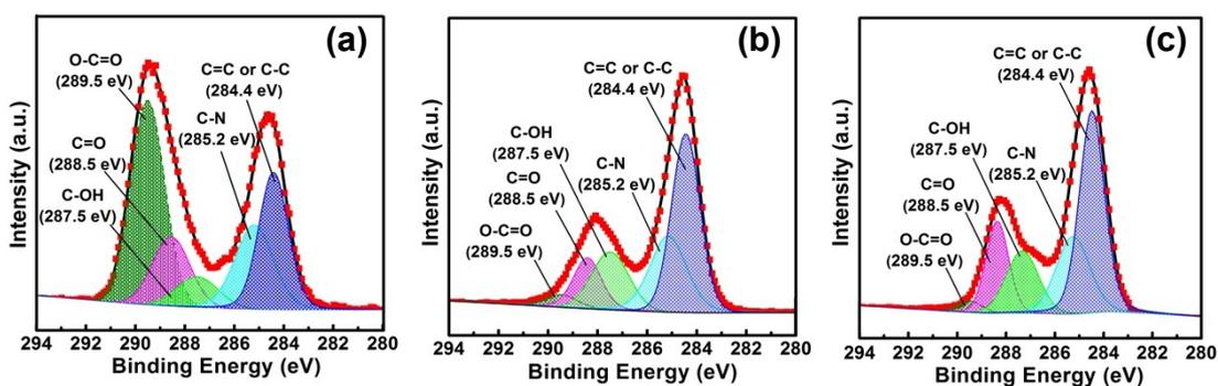
Figure S1. The C 1s peak deconvoluted by a multiple Gaussian function: (a) NCD-1, (b) NCD-2, and (c) NCD-3.
