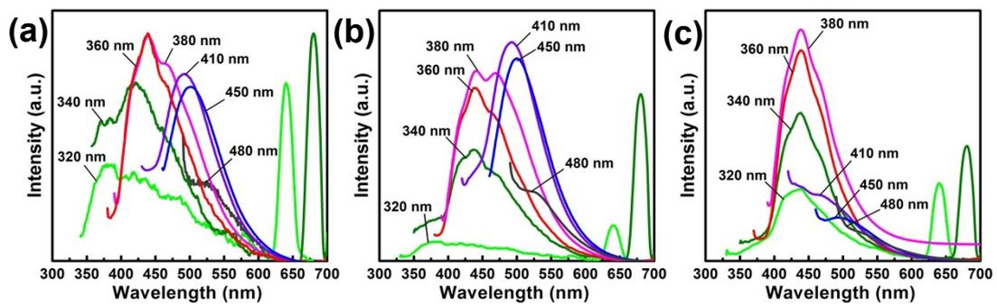
Figure S5. PL emission spectra of different samples in NMP: (a) NCD-1, (b) NCD-2, and (c) NCD-3.
