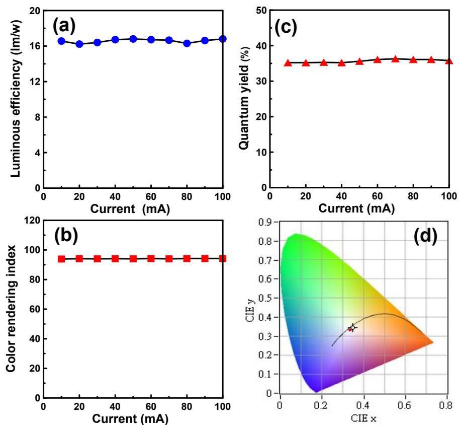
Figure S8. (a) Luminous efficiency, (b) color rendering index, and (c) quantum yield of LED using NCD-1 quantum dots at various working currents. (d) Color coordinates of the white LEDs lamp under 450 nm excitation.
