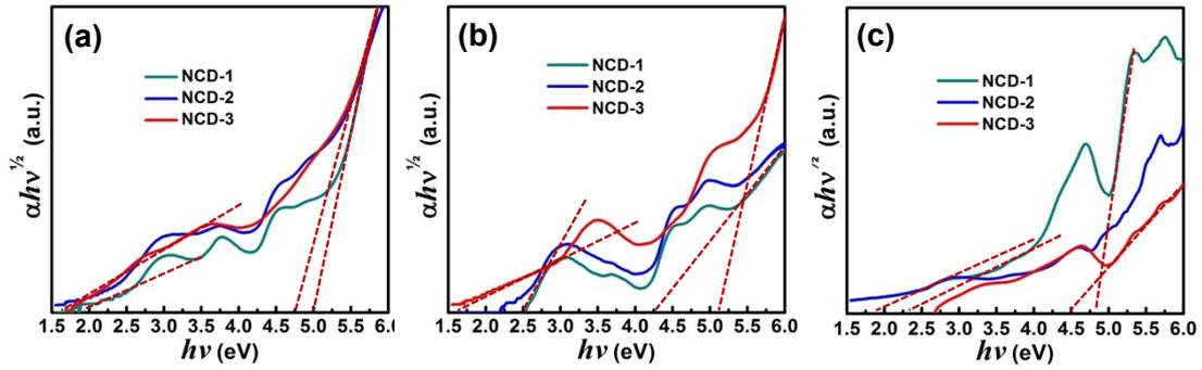
Figure S2. Tauc plots of quantum dots in different solutions: (a) distilled water, (b) ethanol, and (c) NMP.
