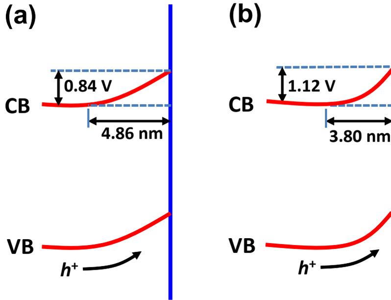
Figure S4. Schematic band structures near surface based on the calculated electronic parameters for (a) NCD-1 and (b) NCD-3 electrodes, based on the flat band potential determined from the intercept of the M-S plots. Here CB and VB represent conduction band and valence band, respectively.
