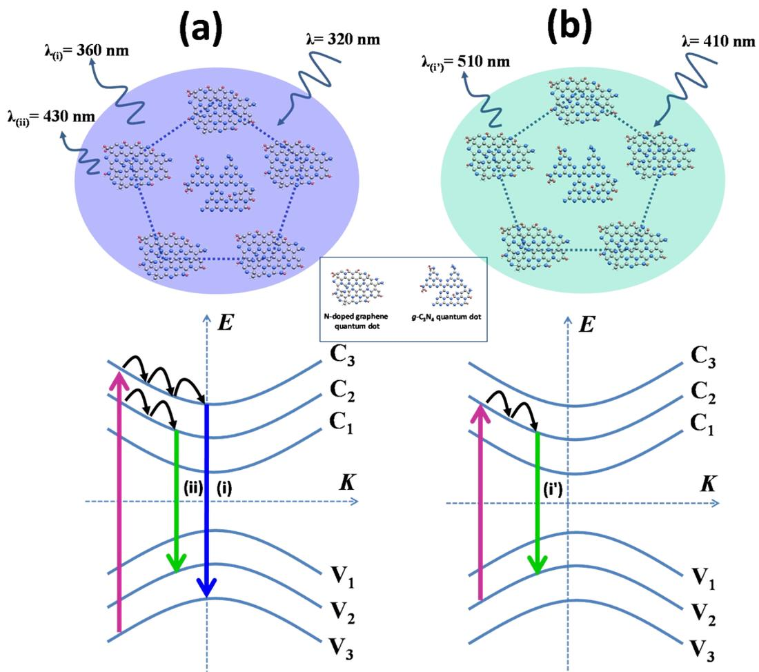
Figure S7. Optical band gap structures on NCD-3 sample under different illuminations: (a) 320 nm UV and (b) 450 nm blue light.
