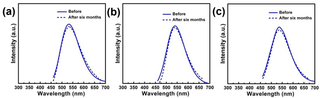
Figure S6. PL emission spectra of different samples in water under 450 nm.
