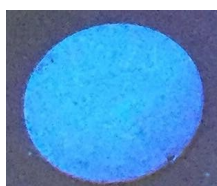
Figure S9: Photo image of a ANMOF-74(Mg) pellet during irradiation with a 365 nm wavelength.
