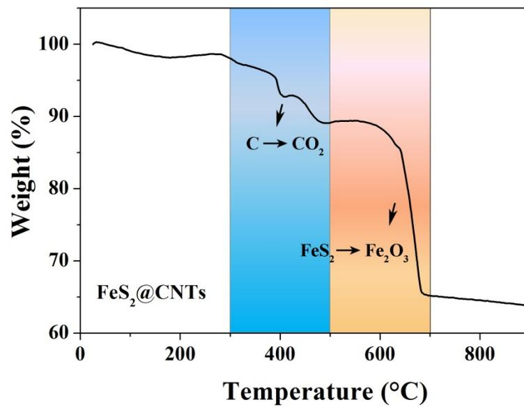
**Figure S5.** TGA curve of FeS<sub>2</sub>@CNTs under air atmosphere.
