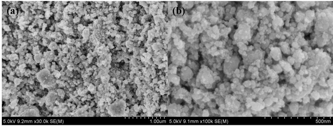
**Figure S6.** SEM images of FeS<sub>2</sub> under low (a) and high magnifications (b).
