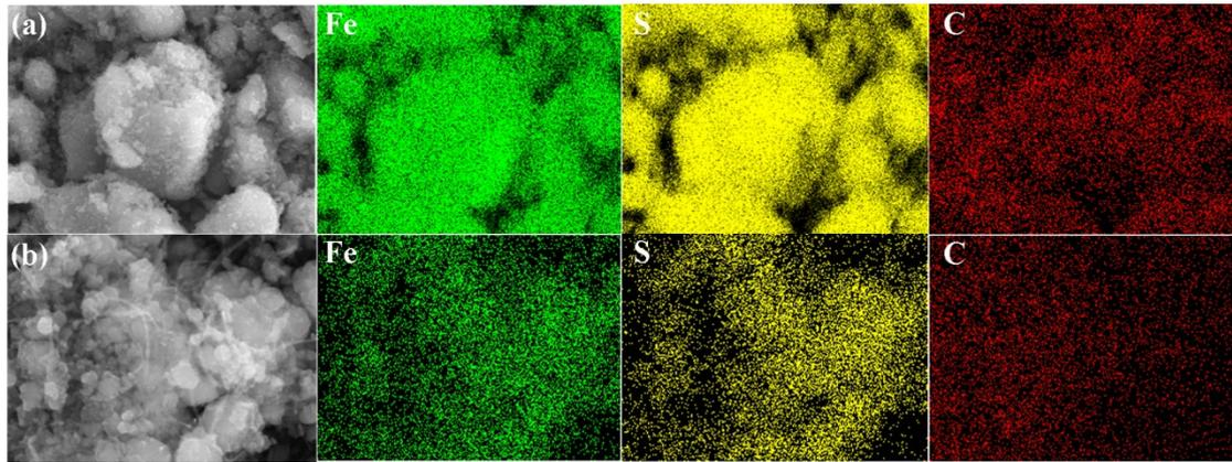
**Figure S7.** Element mapping of FeS<sub>2</sub>@CNTs (a) and FeS<sub>2</sub>+CNTs (b).
