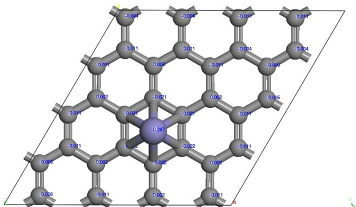
**Figure S3.** Charge transfer between Fe and C atoms.
