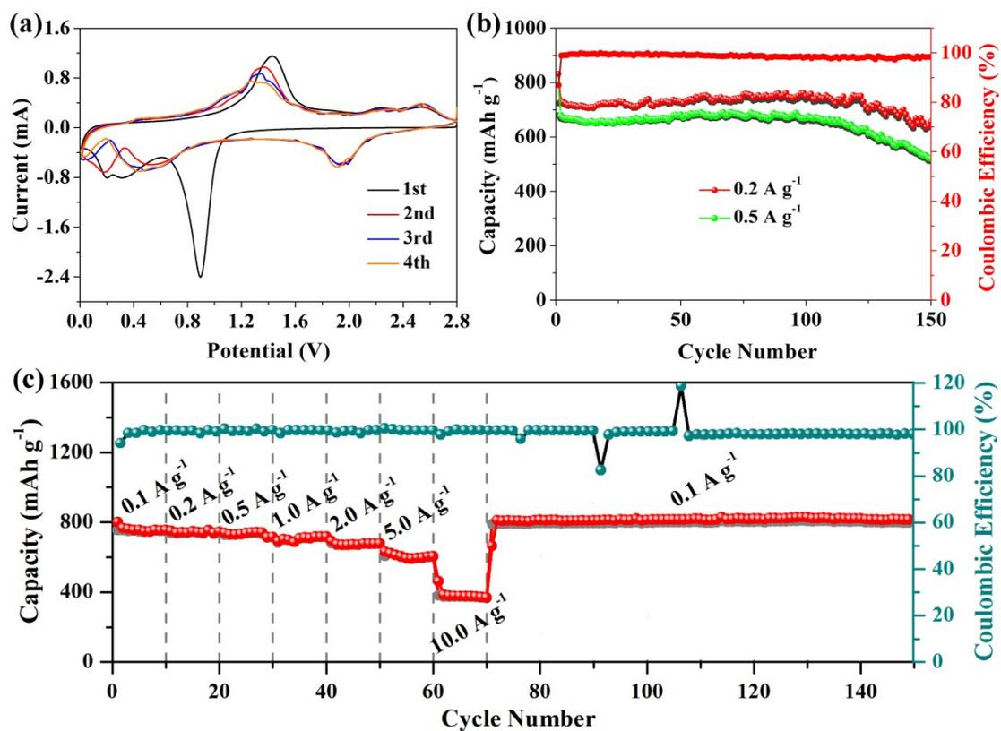
**Figure S8.** The electrochemical performance of FeS<sub>2</sub>@CNTs at a cut off voltage of 0.01–2.8 V. (a) CV curves for the first four cycles at a scan rate of 0.2 mV s<sup>-1</sup>. (b) Cycling performance at current density of 0.2 A g<sup>-1</sup> and 0.5 A g<sup>-1</sup>. (c) Rate performance at various current densities.
