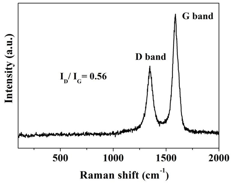
**Figure S2.** Raman spectrum of the pristine CNTs.
