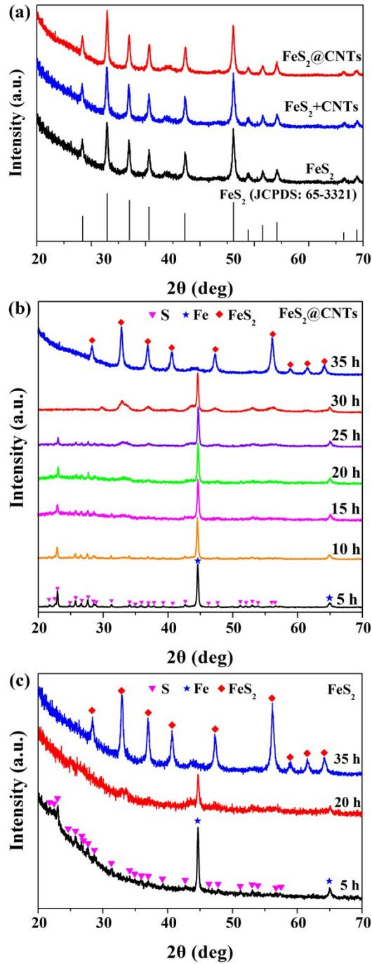
**Figure S1.** (a) XRD patterns of FeS<sub>2</sub>@CNTs and FeS<sub>2</sub> after mechanical milling for 35 h and FeS<sub>2</sub>+CNTs ball milling for 5 h. The Bragg positions of the pyrite FeS<sub>2</sub> with Pa-3 symmetry are indexed accordingly. XRD patterns of FeS<sub>2</sub>@CNTs (b) and FeS<sub>2</sub> (c) for various mechanical alloying times.
