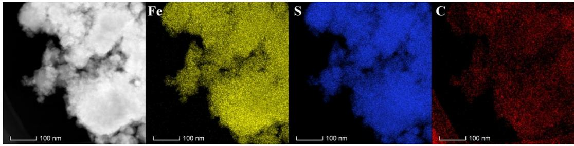
**Figure S4.** Elemental mapping of the as-prepared FeS<sub>2</sub>@CNTs.
