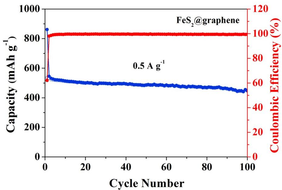
**Figure S9.** Cycling performance and coulombic efficiency of a FeS<sub>2</sub>@graphene composite at a current density of 0.5 A g<sup>-1</sup>.
