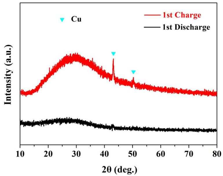
**Figure S10.** *Ex situ* XRD patterns of FeS<sub>2</sub>@CNTs after fully discharging and charging.
