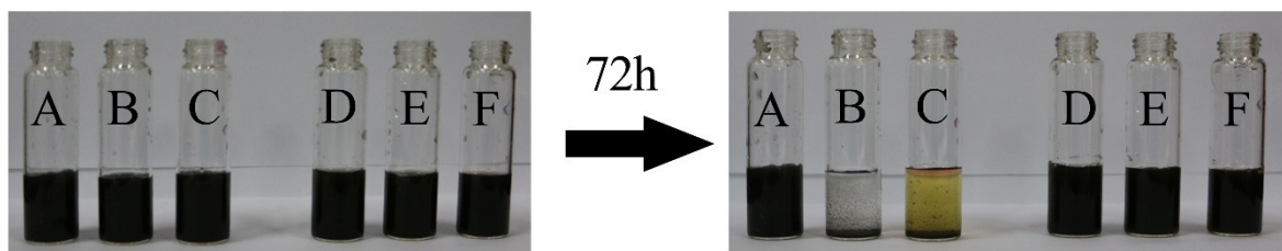
Figure S3. Stabilities of the as-prepared FePt/MoS 2 were dissolved in H 2 O (A), PBS (B), and DMED medium (C) or FPMF NCs were dissolved in H 2 O (D), PBS (E), and DMED medium (F) for 72 h, respectively
