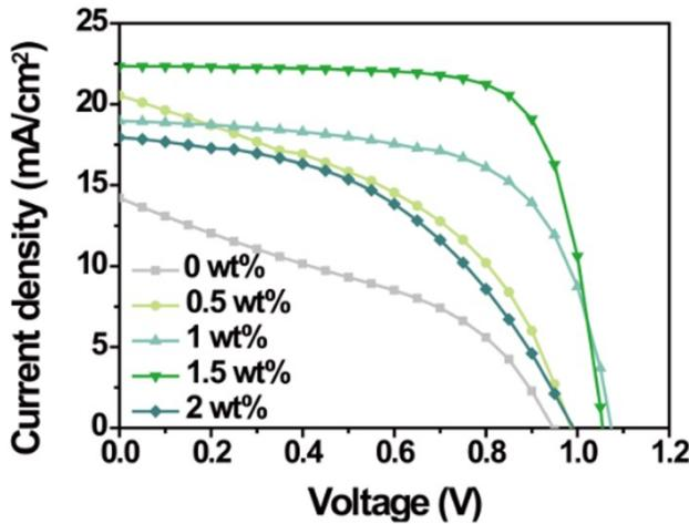
**Figure S3.** Photovoltaic performance of PCSSs based on TFB with increasing F4-TCNQ dopant concentration under AM 1.5 G illumination.
