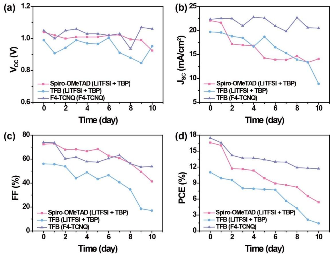
**Figure S7.** Photovoltaic decay curve for the perovskite solar cells in air atmosphere with humidity of about 45%.
