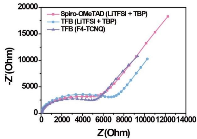
**Figure S5.** Nyquist plots of the PSC devices with different HTLs in whole region.
