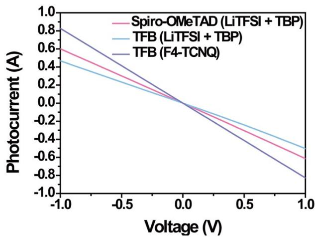
**Figure S6.** I-V curves of the three different hole transport layer only devices.
