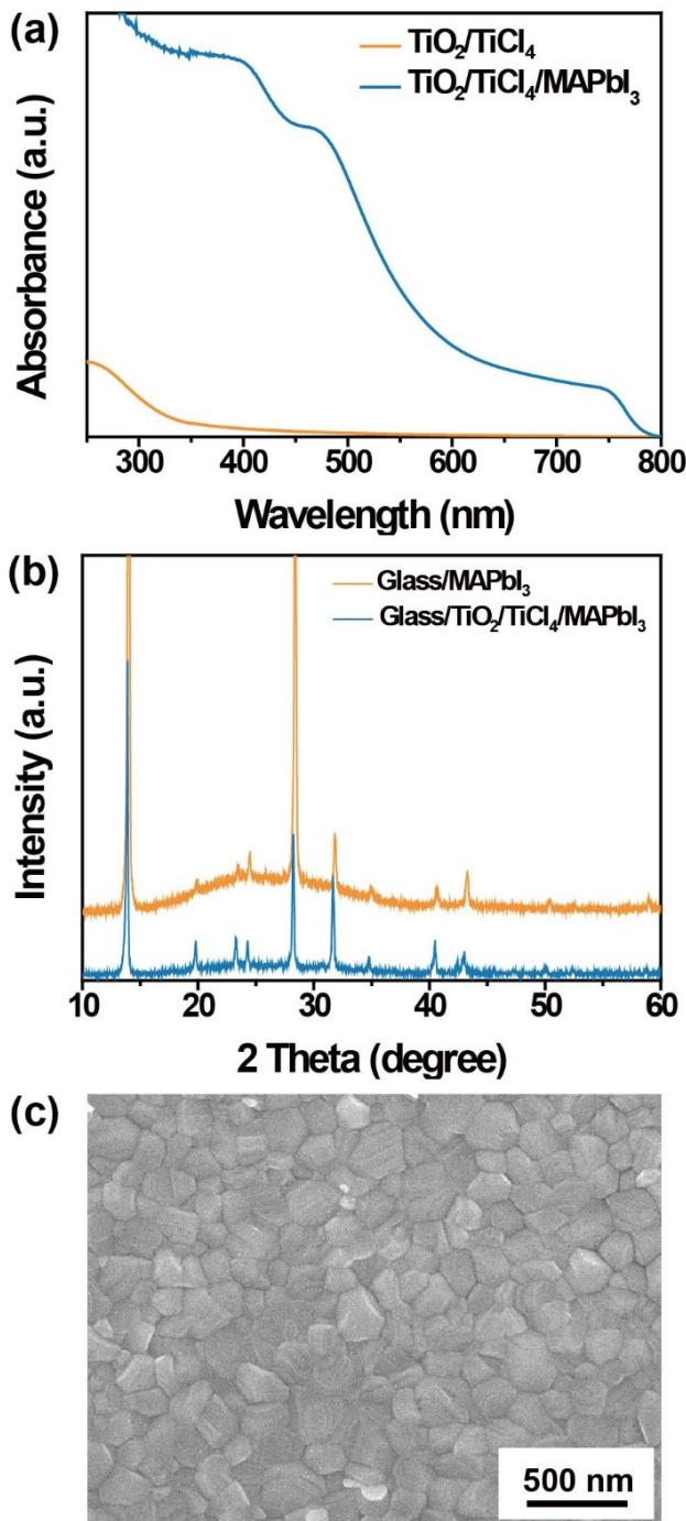
**Figure S2.** (a) UV-vis absorbance spectra of  $\text{TiO}_2/\text{TiCl}_4$  layer and  $\text{TiO}_2/\text{TiCl}_4/\text{Perovskite}$  layer. (b) XRD spectrum of the perovskite and  $\text{TiO}_2/\text{TiCl}_4/\text{Perovskite}$  surface coated on the glass substrate. (c) SEM image of perovskite surface.
