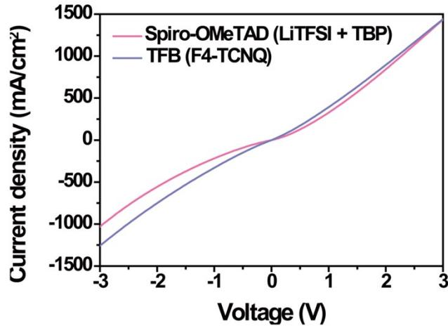
**Figure S11.** Current density versus applied voltage measured by hole-only devices at room temperature.
