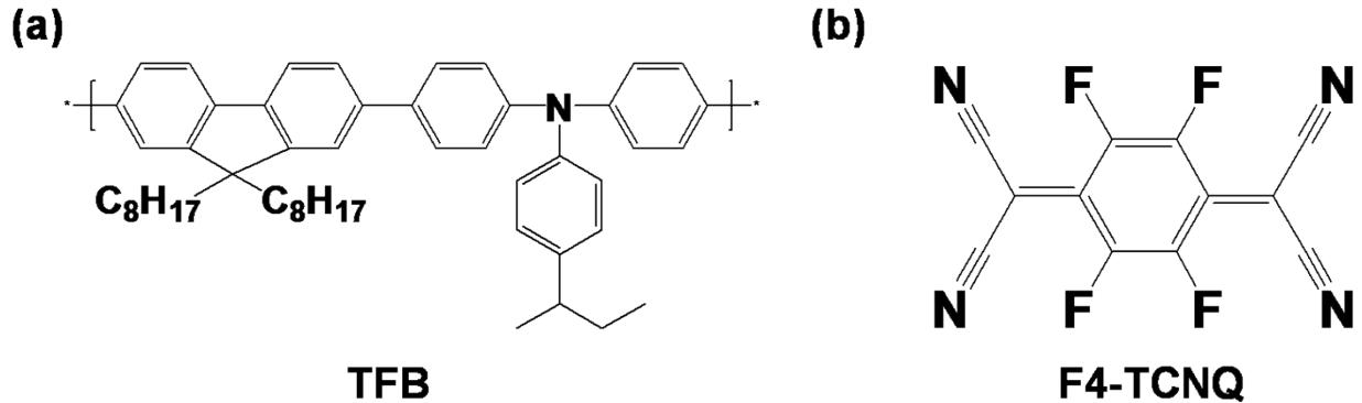
**Figure S1.** Chemical structure of (a) TFB and (b) dopant F4-TCNQ.
