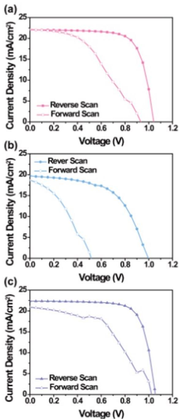
**Figure S4.** Hysteresis of the (a)  $\text{MAPbI}_3/\text{Spiro-OMeTAD}$  ( $\text{LiTFSI} + \text{TBP}$ ), (b)  $\text{MAPbI}_3/\text{TFB}$  ( $\text{LiTFSI} + \text{TBP}$ ), (c)  $\text{MAPbI}_3/\text{TFB}$  ( $\text{F4-TCNQ}$ ) films.
