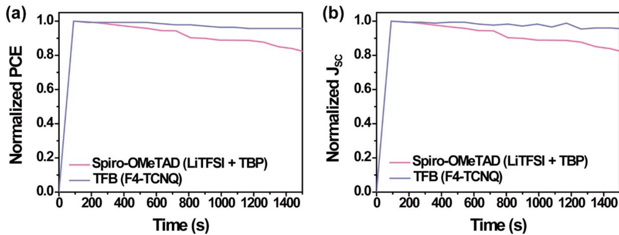
**Figure S9.** The steady state power output of a representative PSC devices based on Spiro-OMeTAD (LiTFSI + TBP) and TFB (F4-TCNQ) was measured at a constant bias of 0.75 and 0.8 V, respectively.
