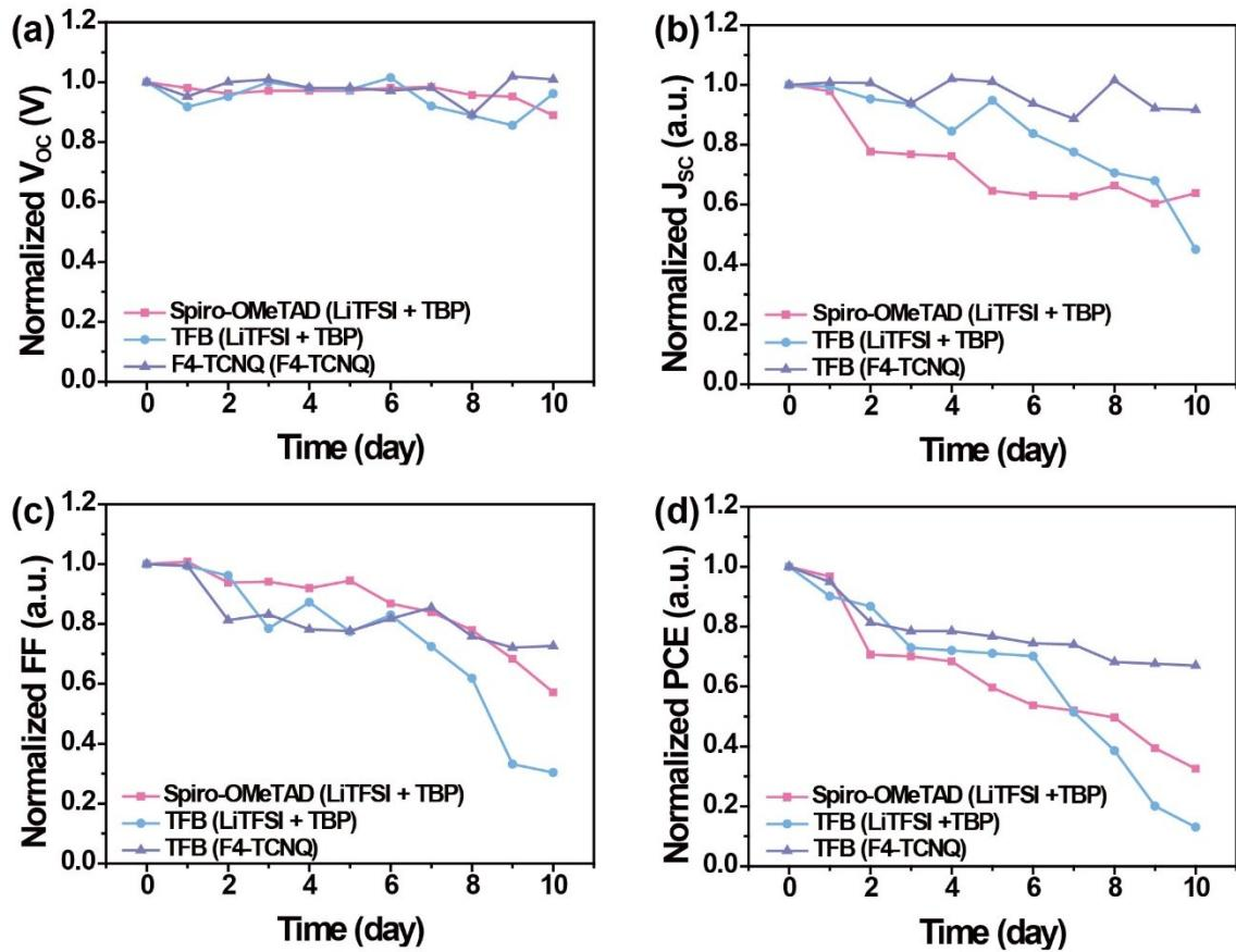
**Figure S8.** Normalized photovoltaic decay curve for the perovskite solar cells in air atmosphere with humidity of about 45%.
