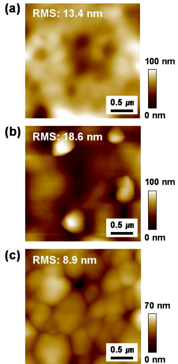
**Figure S10.** AFM images of the (a)  $\text{MAPbI}_3$ /Spiro-OMeTAD (LiTFSI + TBP), (b)  $\text{MAPbI}_3$ /TFB (LiTFSI + TBP), (c)  $\text{MAPbI}_3$ /TFB (F4-TCNQ) films.
