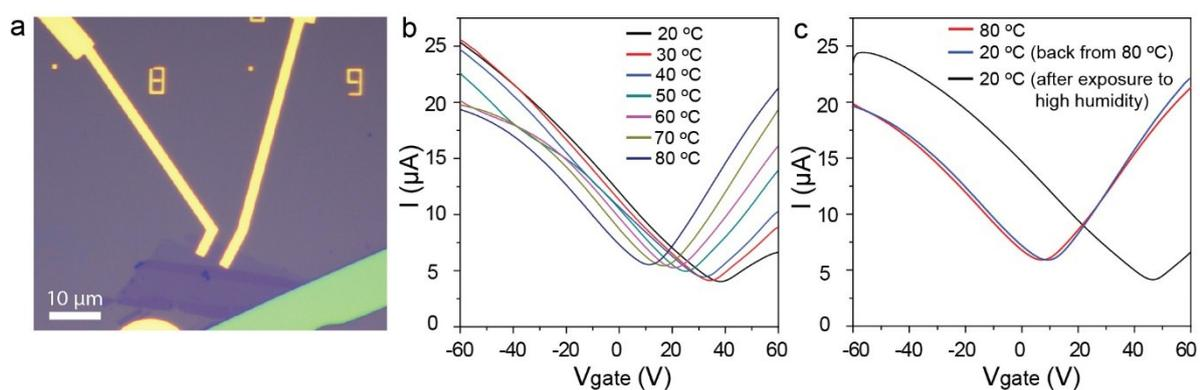
Figure S3. Graphene FET transport measurement under different temperatures. (a) Optical image of the as-fabricated graphene FET devices. (b) Source-drain current ( $I$ ) as a function of back gate voltage ( $V_{\text{gate}}$ ) of monolayer graphene supported on SiO<sub>2</sub>/Si substrate measured at different temperatures under vacuum. (c)  $I$ -  $V_{\text{gate}}$  curves of monolayer graphene measured at 80 °C, 20°C (back from 80 °C) and 20 °C (after exposure to high humidity).
