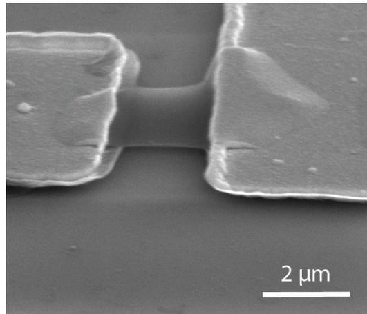
Figure S4. SEM image of suspended monolayer graphene device.
