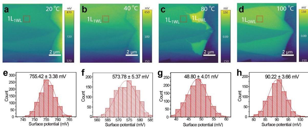
Figure S2. The surface potential of graphene supported on SiO<sub>2</sub>/Si at different temperature. (a-d) *In situ* surface potential mapping corresponding to Figure 2 measured by SKPM. (e-h) The statistical distribution of surface potential of red dashed box area in (a-d).
