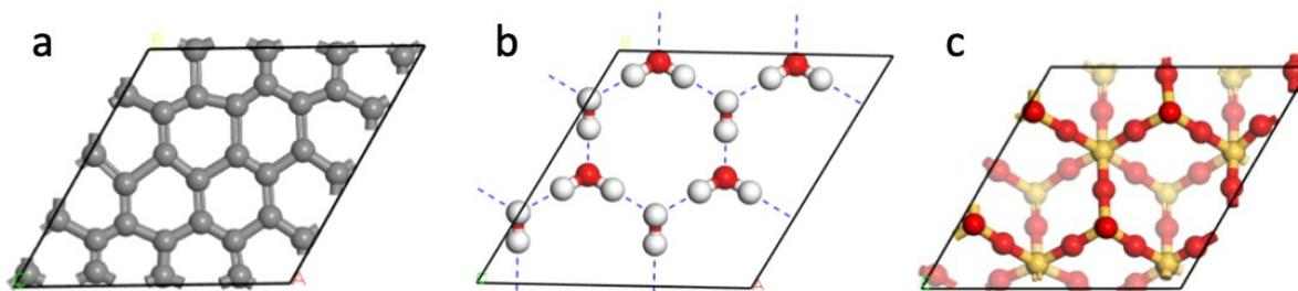
Figure S7. Top-view of the supercells of (a) monolayer graphene ( $4\times 4$ ), (b) monolayer water ( $2\times 2$ ), and (c) three-layer  $\text{SiO}_2$  substrate ( $2\times 2$ ).
