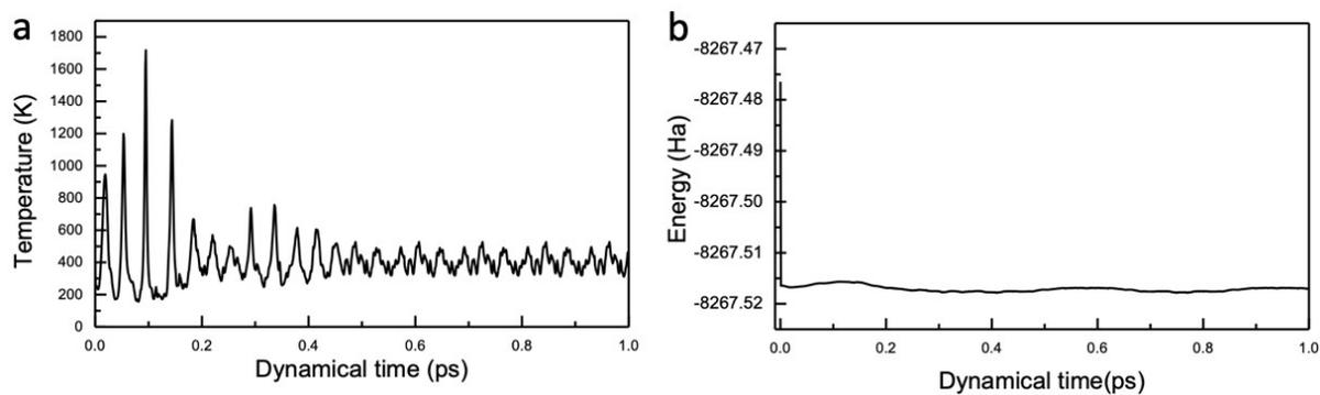
Figure S5. Ab initio molecular dynamics of  $1L_{0WL}$  by Dmol<sup>3</sup>, in the NVT ensemble and Massive GGM thermostat. The step is 0.5fs and 2000 steps totally. The temperature (a) and energy (b) reach to stability after 1ps relaxation. At the end of calculation, we found the work function at 400K is close to 4.56eV as measured by SKPM at 80 °C.
