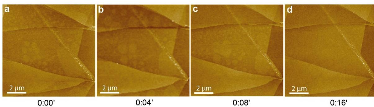
Figure S1. (a-d) *In situ* AFM height images of the interfacial water layer growth during the scanning. It can be clearly seen that the isolated interfacial water layers coalesced into a continuous water layer takes ~16 mins.
