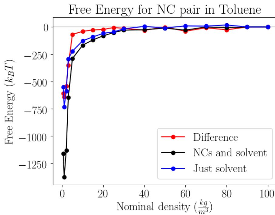
Figure S12: The Free energy of the NC pair and solvent system (black), compared with that of a system composed of just solvent (blue), and the difference between the two (red).
