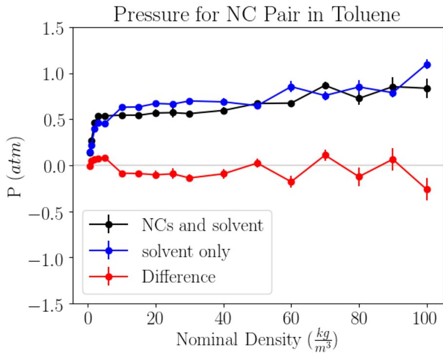
Figure S11: Pressure taken directly from the simulations for a pair of NCs in solvent (black), just solvent (blue), and the difference between the two (red). Error bars quoted are for a one standard deviation error.
