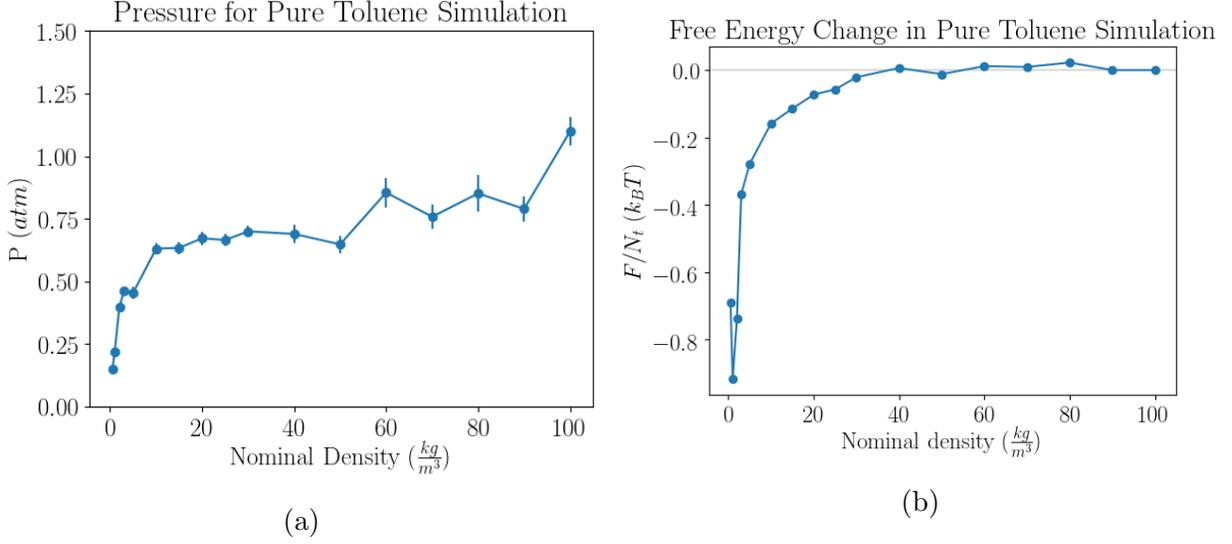
Figure S10: (Left) Pressure data for pure toluene, using the peaks of the distributions similar to Fig. 1b and then applying Eq. 5, as a function of nominal density. (Right) Calculated free energy change (from Eq. S12) per solvent molecule throughout the simulation.
