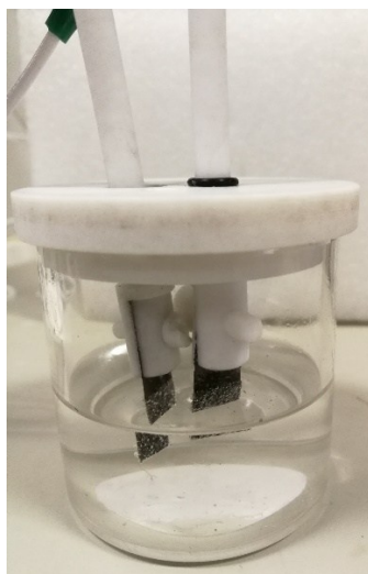
Figure S20. The photograph of electrochemical overall water splitting cell ( \text{Ni}_{0.8}\text{Fe}_{0.2}\text{-m/t-Se}_{0.02}\text{-LDH//Pt/C} ).
