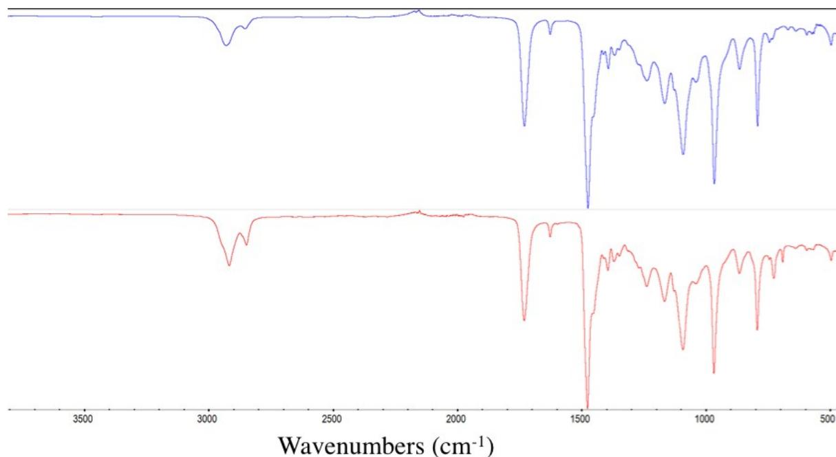
**Figure S.12.** Comparison FTIR spectra of pure ligand **I2** (Top, blue) and the exchanged AuNP-**I2** (Bottom, red). The particles in toluene were drop-casted on diamond and spectrum was recorded after solvent evaporation.
