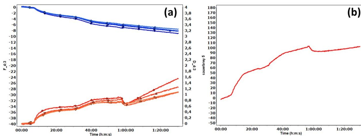
**Figure S.18.** Deposition of AuNP-I2 on the surface of QCM-D sensors functionalized with DT ligands. (a) Change in frequency and dissipation with time. (b) Mass gain as a function of time.
