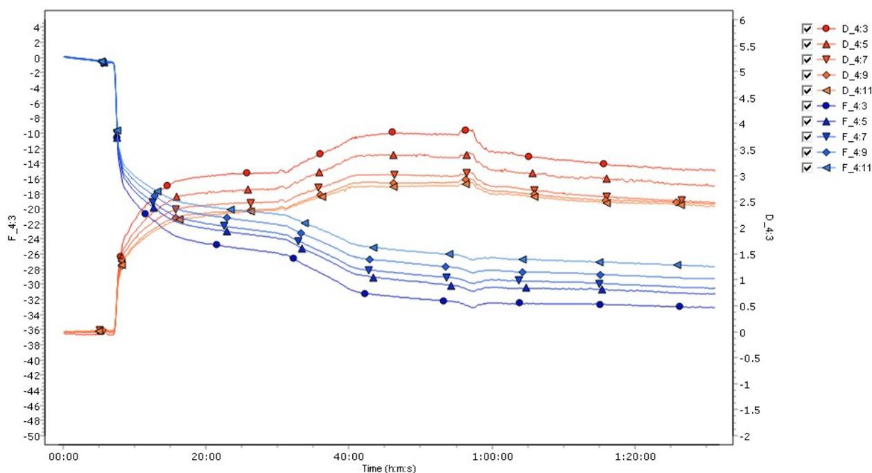
**Figure S.17.** QCM-D measurement of change in frequency change and the change in dissipation plotted against time upon the adsorption of AuNP-I2 on the QCM-D sensor coated with Py1 ligand.
