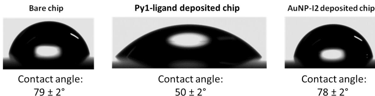
**Figure S.19.** Static water contact angles of the bare gold sensor (left), functionalized with the XB acceptor ligand (middle) and sensor deposited with AuNP-I2 on top of the XB acceptor ligand (right).
