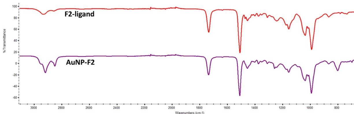
**Figure S.10.** Comparison FTIR spectra of pure ligand **F2** (Top, red) and the exchanged AuNP-**F2** (Bottom, magenta). The particles in toluene were drop casted on diamond and spectra was recorded after solvent evaporation.
