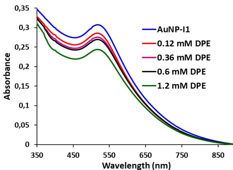
**Figure S.9.** UV-Vis spectra of AuNP-**II** compared upon incremental addition of 1,2-Di(4-pyridyl)ethylene. Obtained data show no changes in the SPR bands even when an excess of the XB acceptor system is present. AuNP-**II** were not used to prepare XB driven AuNPs assemblies as they
