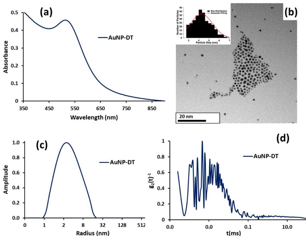
**Figure S.6.** (a) UV-Vis spectra of AuNP-DT. (b) TEM image of AuNP-DT showing the NPs size distribution (inset) resulting in NPs averaged diameter of about 4 nm. (c) Intensity weighted NP size distributions obtained by DLS for AuNP-DT dispersion in toluene at 90° obtained through CONTIN analysis. (d) Scattered intensity auto-correlation functions of AuNP-DT dispersion in toluene.
