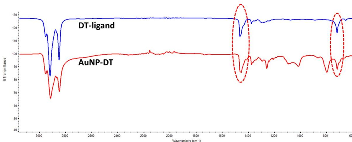
**Figure S.5.** FTIR spectra of pure **DT** (Top, blue) and **AuNP-DT** (Bottom, red), the particles in toluene were drop casted on diamond and the spectrum was recorded after solvent evaporation.
