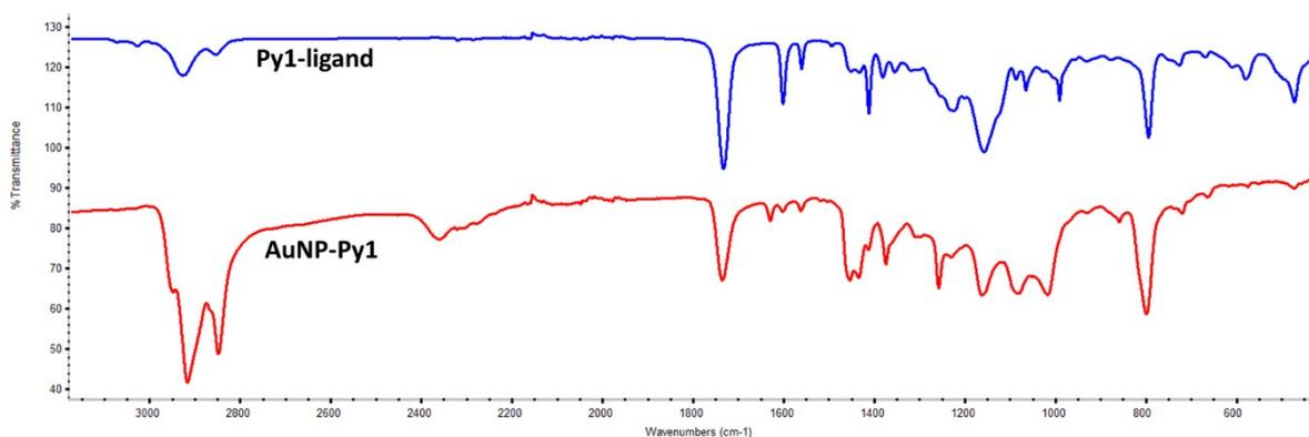
**Figure S.2.** Comparison between FTIR spectra of the pure ligand **Py1** (Top, blue) and the synthesized AuNP-Py1 (Bottom, red).
