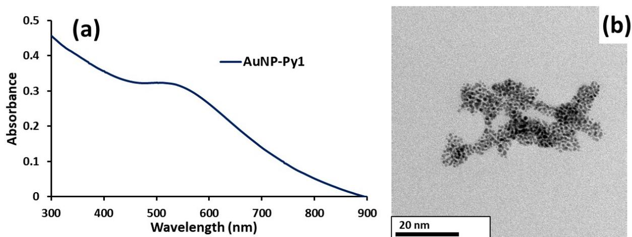
**Figure S.3.** (a) UV-Vis spectra of AuNP-Py1 dispersion showing a broadening of the surface plasmon peak. (b) Representative TEM image of AuNP-Py1 showing aggregation of particles.
