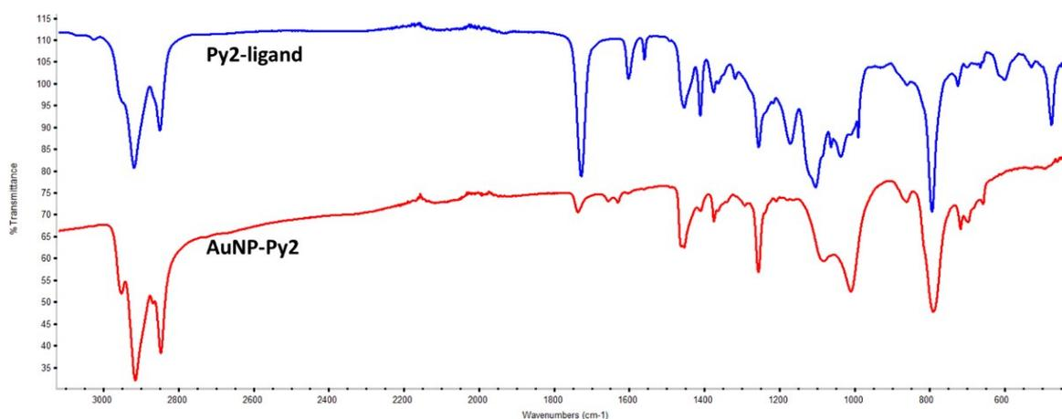
**Figure S.11.** Comparison FTIR spectra of pure ligand **Py2** (Top, blue) and the exchanged AuNP-**Py2** (Bottom, red). The particles in toluene were drop-casted on diamond and spectrum was recorded after solvent evaporation.
