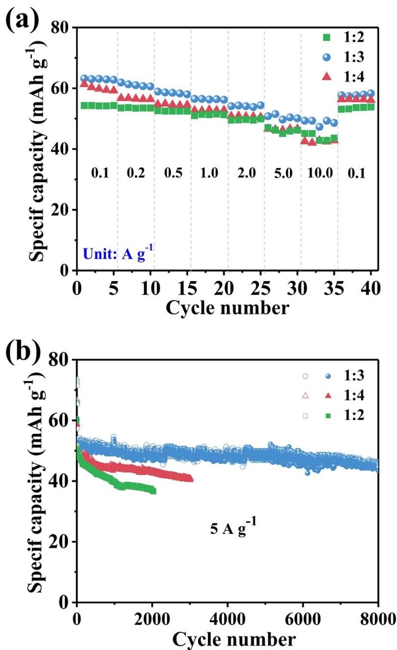
**Fig. S7.** (a) Rate capability and (b) cycling performance of the HNCNB//PHNCNB hybrid capacitors with different anode to cathode mass ratios.
