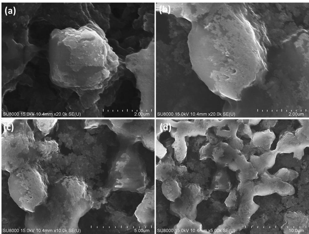
**Fig. S5** SEM images of the HNCNB anode after 2000 cycles at  $5.0 \text{ A g}^{-1}$ .
