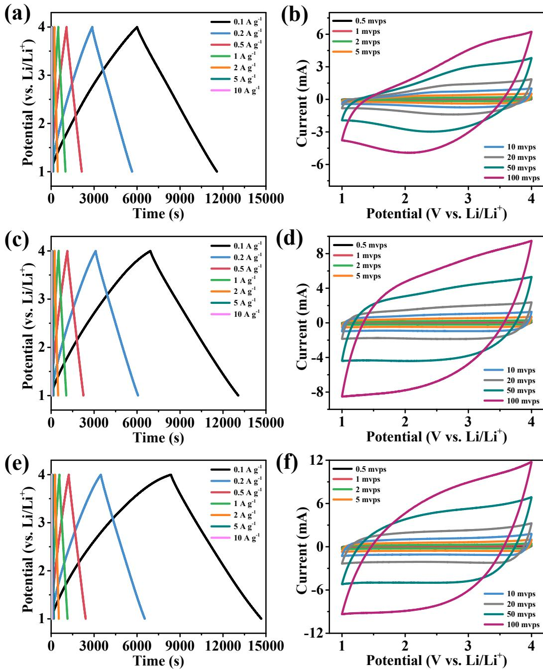
**Fig. S8.** GCD and CV curves of LIHC measured at (a, b) 0 °C, (c, d) 25 °C, (e, f) 60 °C.
