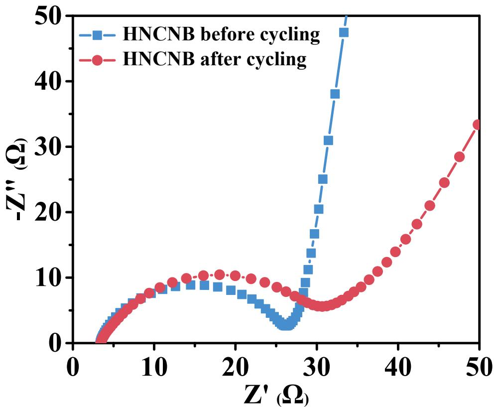
**Fig. S4.** EIS spectra of HNCNB before and after cycling.
