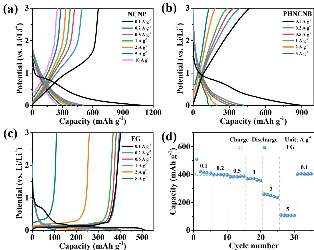
**Fig. S3.** GCD curves of (a) NCNP, (b) PHNCNB and (c) FG, (d) rate performance of FG.
