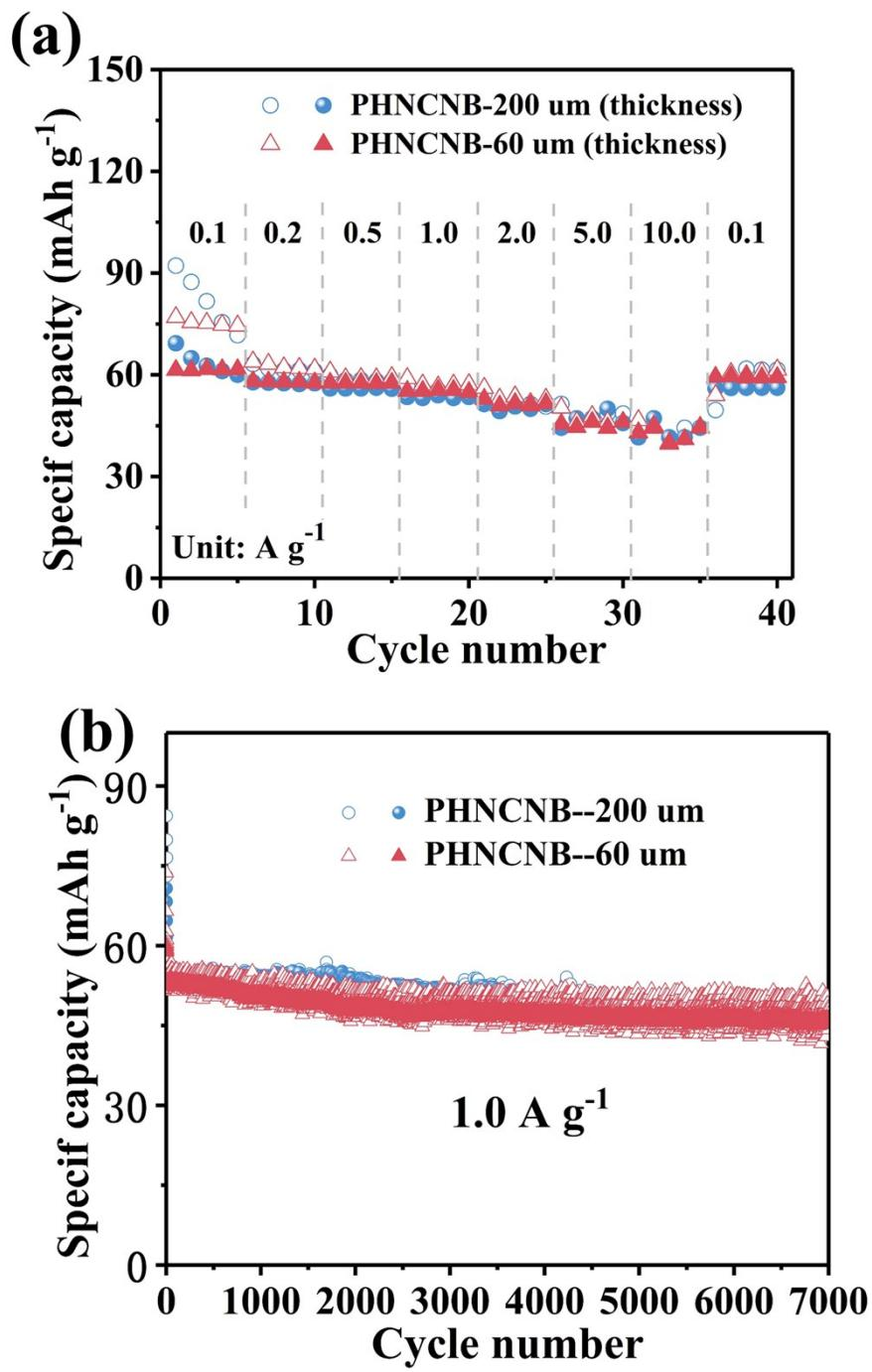
**Fig. S6.** (a) Rate capability and (b) cycling performance of the PHNCNB cathode with two different electrode thicknesses (60 and 200  $\mu\text{m}$ ) in half-cells.
