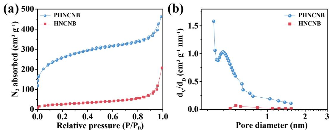
**Fig. S2** (a) Nitrogen adsorption/desorption isotherms and (b) pore-size distribution curve of HNCNB and PHNCNB.
