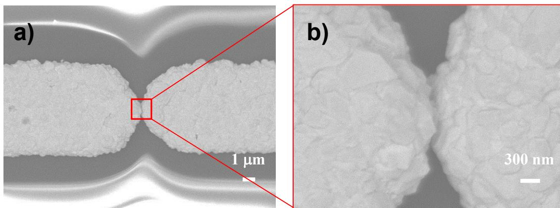
**Figure S5.** SEM images of the electrodes after electroplating. a) Gold electrodes after electroplating. b) Enlarged view of the area framed by the red rectangle in a).
