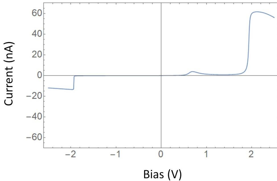
**Figure S10.** Current-voltage ( $IV$ ) characteristic using the three-site model ( $z=0$ ).
