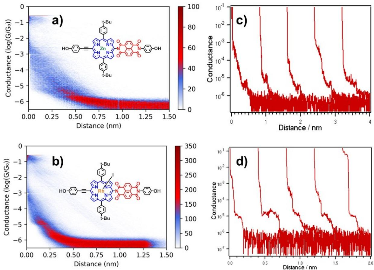
**Figure S2.** (a) 2D Conductance histograms for ZPI constructed obtained from 1767 measurements of individual traces. (b) 2D Conductance histograms for RPI constructed from 4070 measurements of individual traces. Insets: structure of ZPI and RPI. (c-d) Selected individual traces of ZPI and RPI respectively
