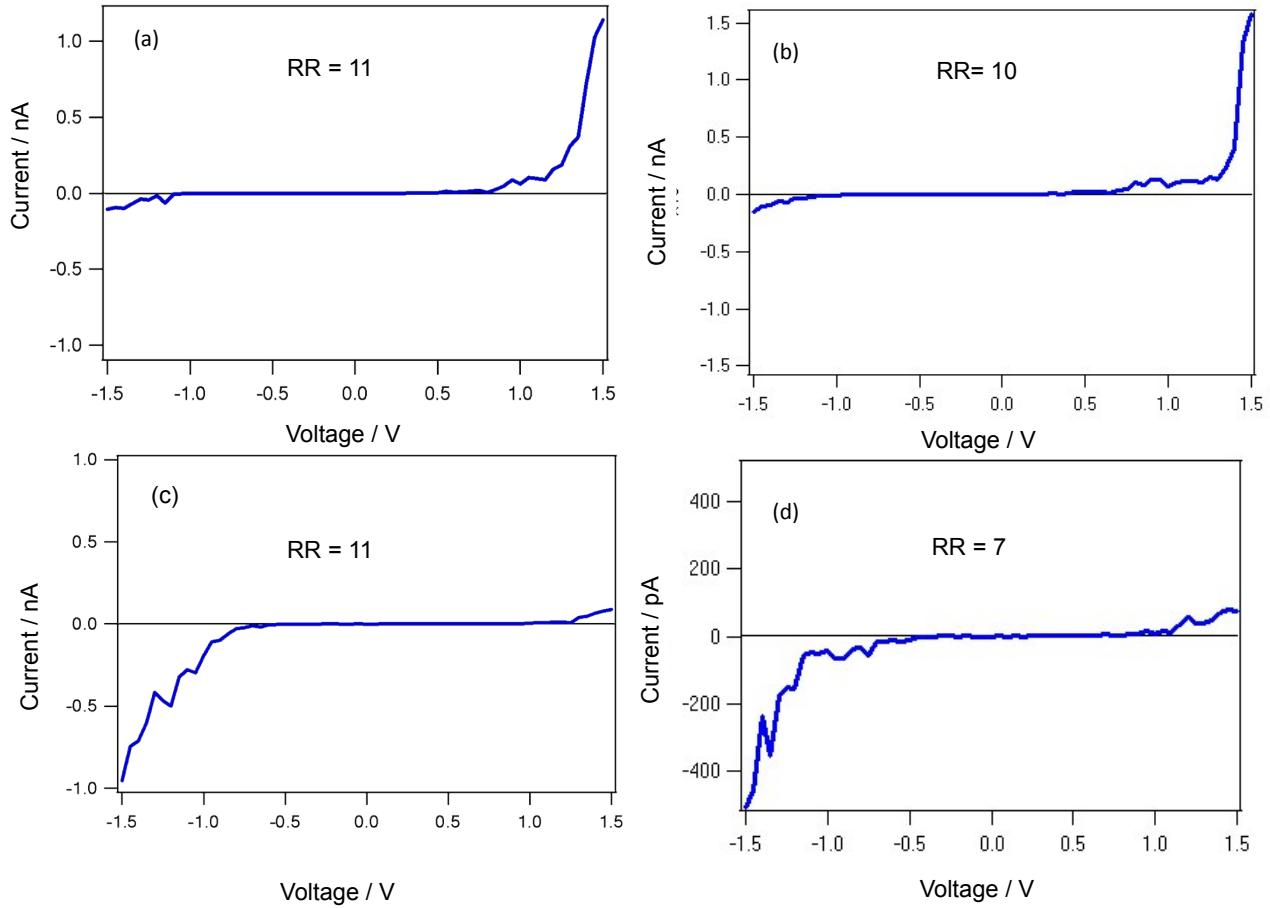
**Figure S1.** Typical individual  $I$ - $V$  curves of ZPI (I) and RPI (II).
