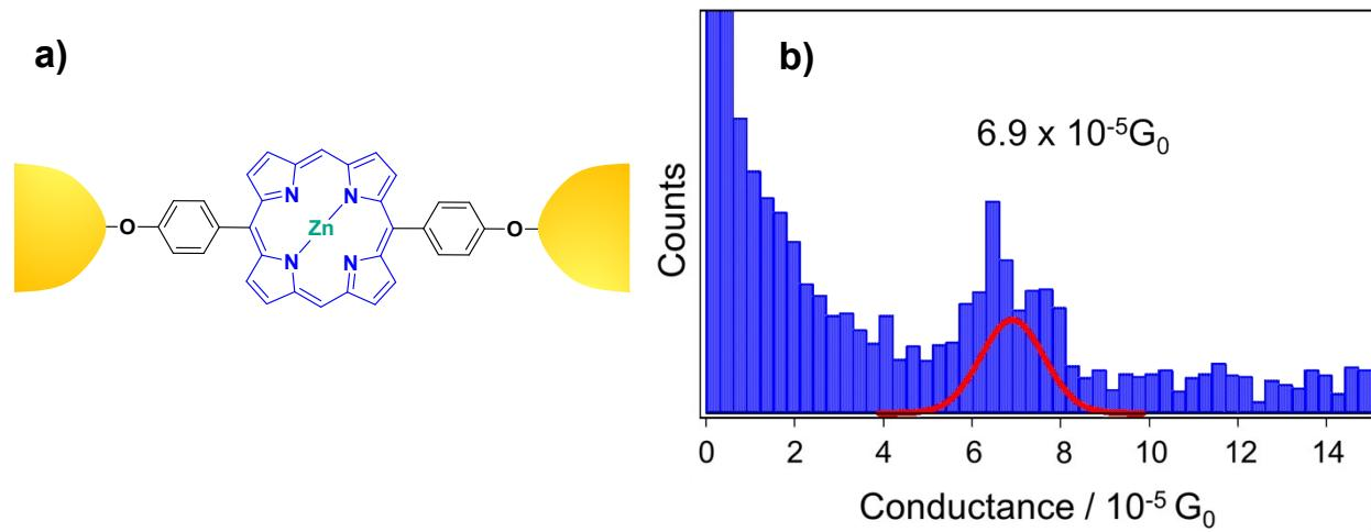
**Figure S4.** Molecular structure and conductance histogram of the symmetric porphyrin molecule Zn<sup>II</sup>-5,15-bis(4-hydorxyphenyl)porphyrin (ZHPP).
