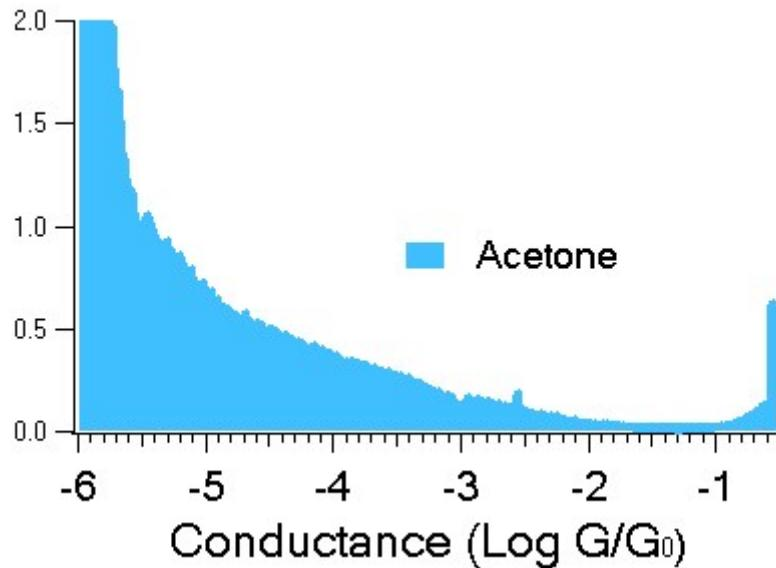
**Figure S3.** Conductance histogram of acetone solvent. It is seen that there is no peak observed in the conductance histogram
