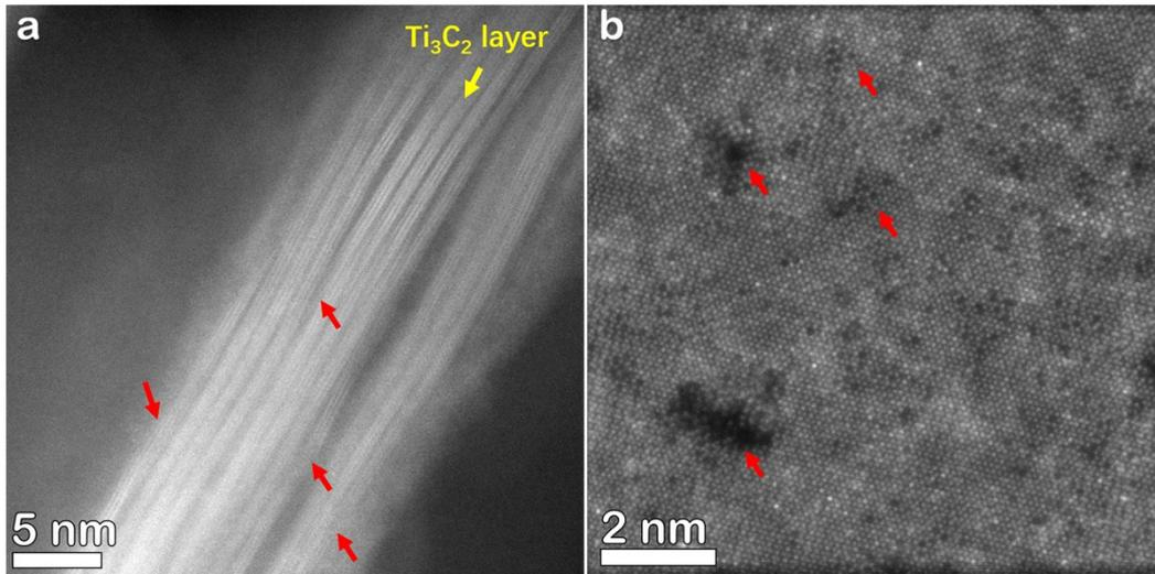
**Figure S6** (a) A cross-sectional STEM image of an incomplete exfoliated  $\text{Ti}_3\text{AlC}_2$  MAX phase, showing the generation of large amount of defects. (b) A plan-view STEM image showing the defects in the  $\text{Ti}_3\text{C}_2$  MXene layer. The only defect found at atomic scale is the Ti-vacancy (or accumulation of many Ti-vacancies) as shown by the red arrowheads.
