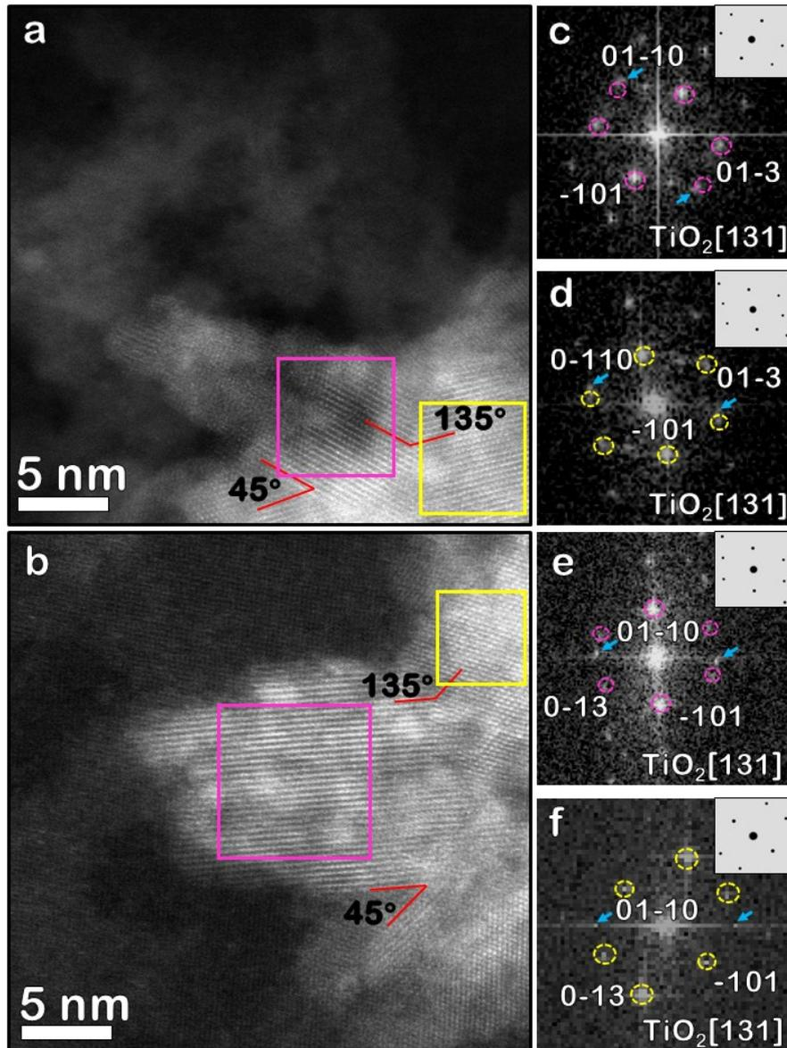
**Figure S4. Phase identification of anatase  $\text{TiO}_2$ :** (a-b) HAADF STEM images showing the formation of  $\text{TiO}_2$  nanoparticles on the substrate of  $\text{Ti}_3\text{C}_2$  MXene. (c-f) The FFT patterns of the area marked by (c) and (e) pink, (d) and (f) yellow box in (a) and (b), compared to the simulated diffractions as insets. The  $\text{TiO}_2$  is identified as anatase phase. Additionally, the  $\text{Ti}_3\text{C}_2$  diffraction spots marked by the blue arrows.
