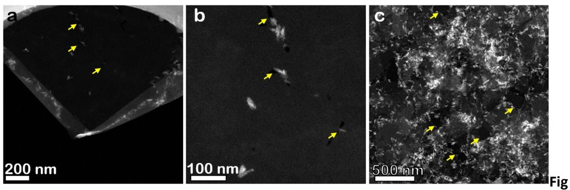
**Figure S8** (a) A HAADF-STEM image showing the formation of TiO<sub>2</sub> nanoparticles (white contrast) along the edges and vertex of the Ti<sub>3</sub>C<sub>2</sub> flake. (b) Inside the Ti<sub>3</sub>C<sub>2</sub> layer, almost every nanoparticle is accompanied with a 'hole' nearby, which is a Ti-vacancy rich area. (c) With more and more TiO<sub>2</sub> nanoparticles appeared, there are more holes while the size of holes become large.
