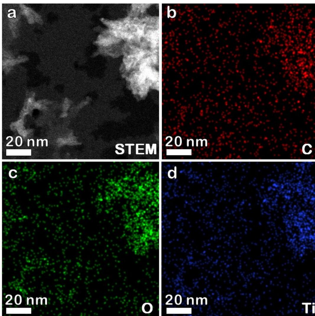
**Figure S3.** (a) HAADF-STEM image at low magnification, (b-d) Corresponding EDS elemental maps of the whole area in (c), C shown in red, O in green and Ti in blue.
