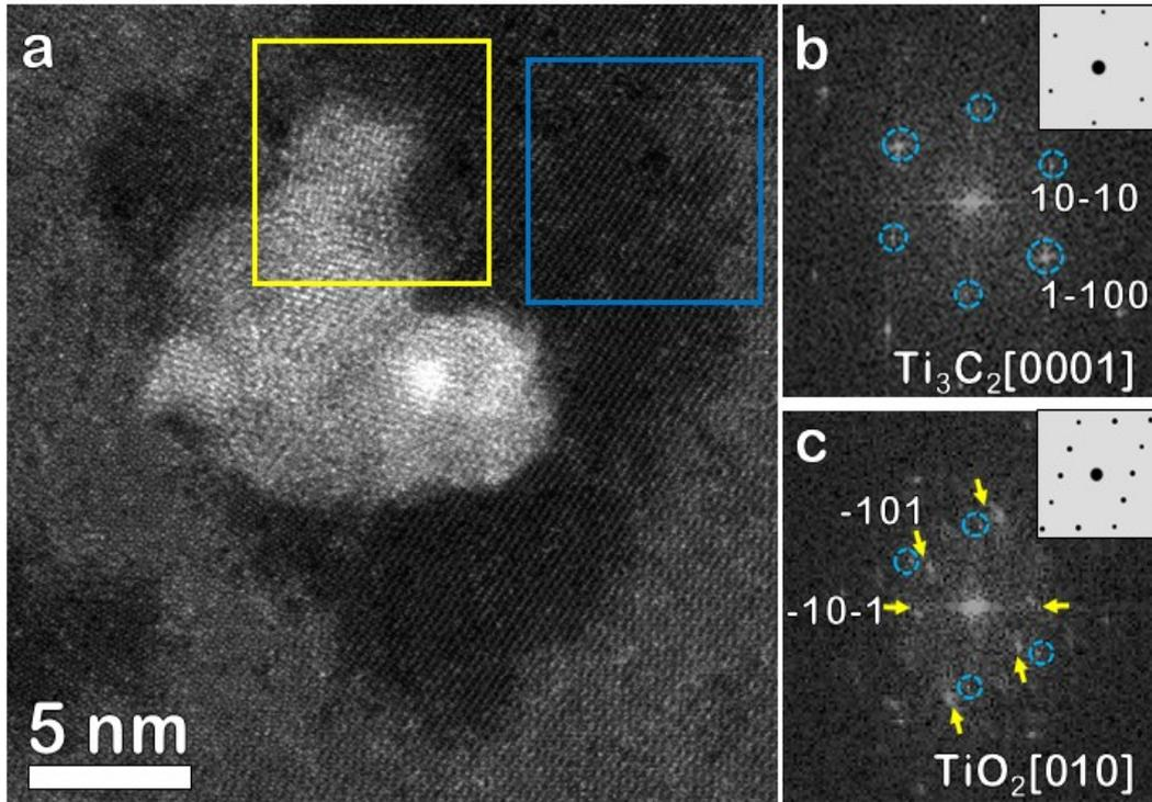
**Figure S5. Other orientation relationship between anatase  $\text{TiO}_2$  and  $\text{Ti}_3\text{C}_2$  MXene.** (a-b) HAADF STEM images showing the formation of  $\text{TiO}_2$  nanoparticles on the substrate of  $\text{Ti}_3\text{C}_2$  MXene. (b-c) The FFT patterns of the area marked by (b) blue, (c) pink box in (a), compared to the simulated diffractions as insets. The  $\text{TiO}_2$  is identified as anatase phase along the [010] axis.
