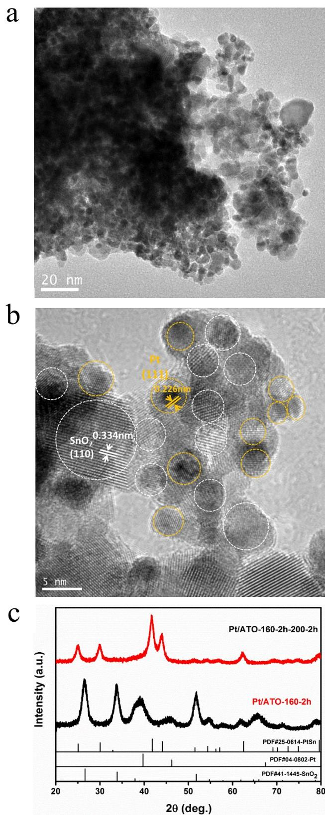
**Figure S4.** (a) and (b)TEM of Pt/ATO-160-2h. (C) XRD of Pt/ATO-160-2h and Pt/ATO-160-2h heated up to 200 °C for 2 h in EG solution.
