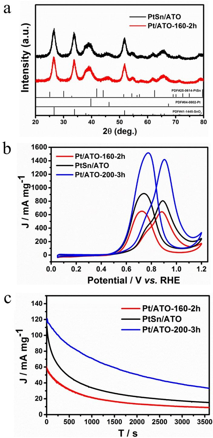
**Figure S7.** (a) XRD of Pt/ATO-160-2h, PtSn/ATO catalysts. (b) CV curves of Pt/ATO-160-2h, PtSn/ATO and Pt/ATO-200-3h catalysts in 0.5 M H<sub>2</sub>SO<sub>4</sub> + 1 M CH<sub>3</sub>OH solution with a sweep rate of 50 mV s<sup>-1</sup>. (c) Chronoamperometric curves of Pt/ATO-160-2h, PtSn/ATO and Pt/ATO-200-3h catalysts in N<sub>2</sub>-saturated 0.5 M H<sub>2</sub>SO<sub>4</sub> + 1 M CH<sub>3</sub>OH solution at constant voltage 0.6 V for 60 mins.
