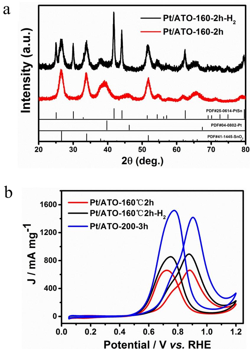
**Figure S6.** (a) XRD of Pt/ATO-160-2h and Pt/ATO-160-2h annealing at 300°C in H<sub>2</sub>/N<sub>2</sub> (denoted as Pt/ATO-160-2h-H<sub>2</sub>) for 2h. (b) CV curves of Pt/ATO-160-2h, Pt/ATO-160-2h-H<sub>2</sub> and Pt/ATO-200-3h catalysts in 0.5 M H<sub>2</sub>SO<sub>4</sub> + 1 M CH<sub>3</sub>OH solution with a sweep rate of 50 mV s<sup>-1</sup>.
