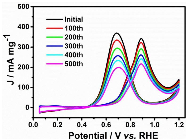
**Figure S8.** Cyclic voltammogram of Pt/C catalyst in  $\text{N}_2$ -saturated 0.5 M  $\text{H}_2\text{SO}_4$  + 1 M  $\text{CH}_3\text{OH}$  solution at scan rate of  $50 \text{ mV s}^{-1}$  during the durability tests.
