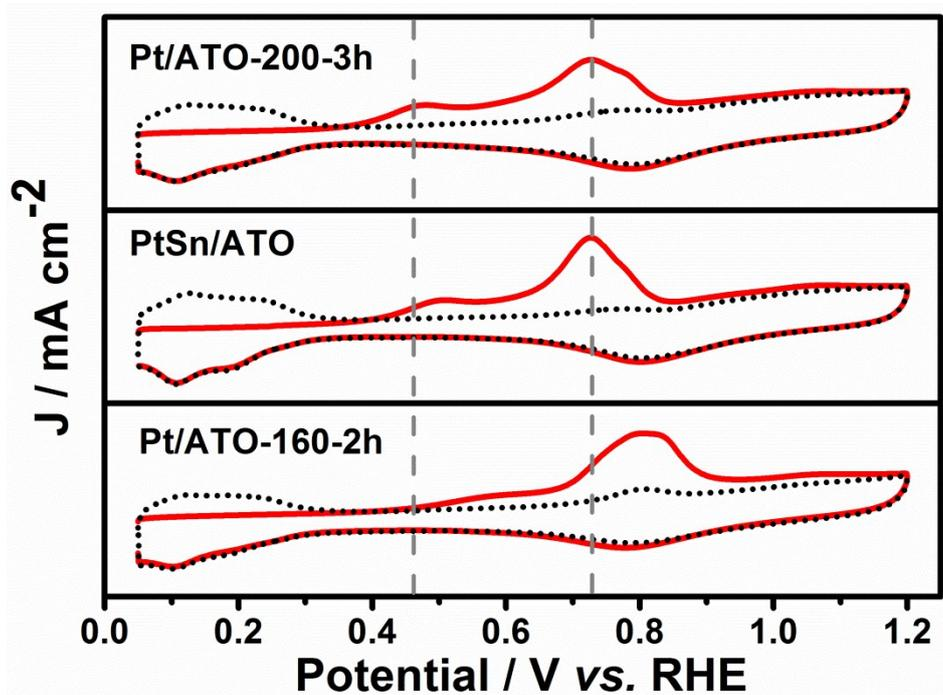
**Figure S9.** CO stripping patterns of Pt/ATO-160-2h, PtSn/ATO and Pt/ATO-200-3h catalysts in 0.5 M of H<sub>2</sub>SO<sub>4</sub>.
