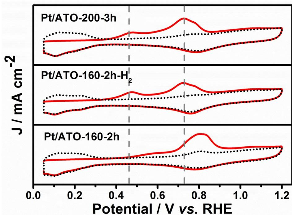
**Figure S10.** CO stripping patterns of Pt/ATO-160-2h, Pt/ATO-160-2h-H<sub>2</sub> and Pt/ATO-200-3h catalysts in 0.5 M of H<sub>2</sub>SO<sub>4</sub>.
