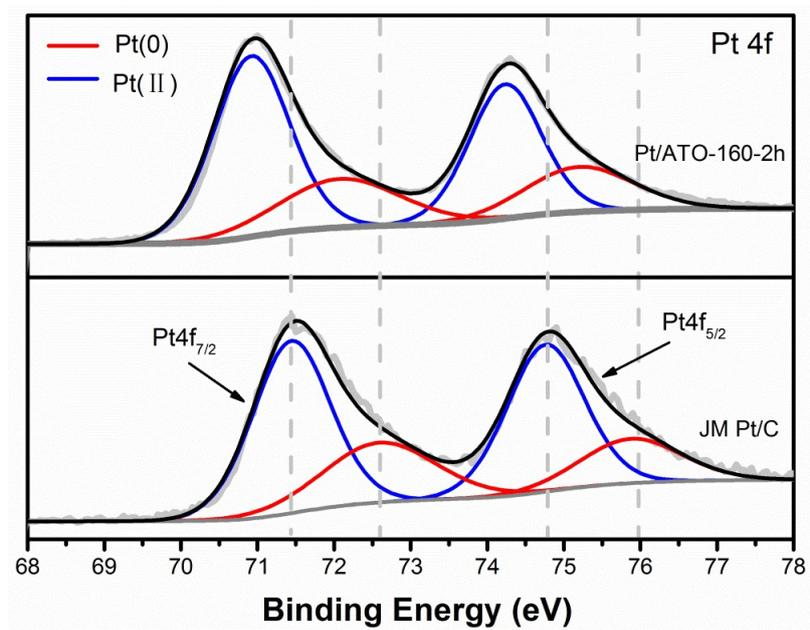
**Figure S5.** XPS spectra of Pt 4f for JM Pt/C and Pt/ATO-160-2h catalysts.
