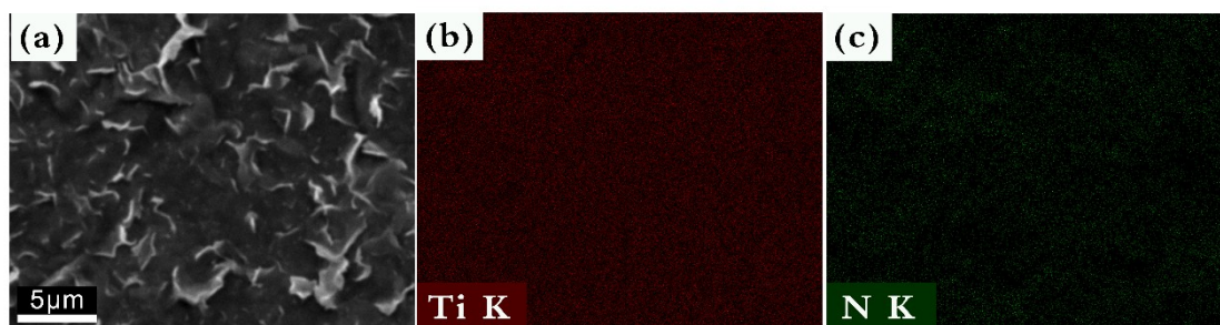
Figure S5. (a) Surface image of d-Ti 3 C 2 T x /ANFs composite paper (b) EDS mapping of d-Ti 3 C 2 T x /ANFs composite paper (element Ti) indicating the evenly dispersion of d-Ti 3 C 2 T x . (c) EDS mapping of d-Ti 3 C 2 T x /ANFs composite paper (element N) indicating the evenly dispersion of ANFs.
