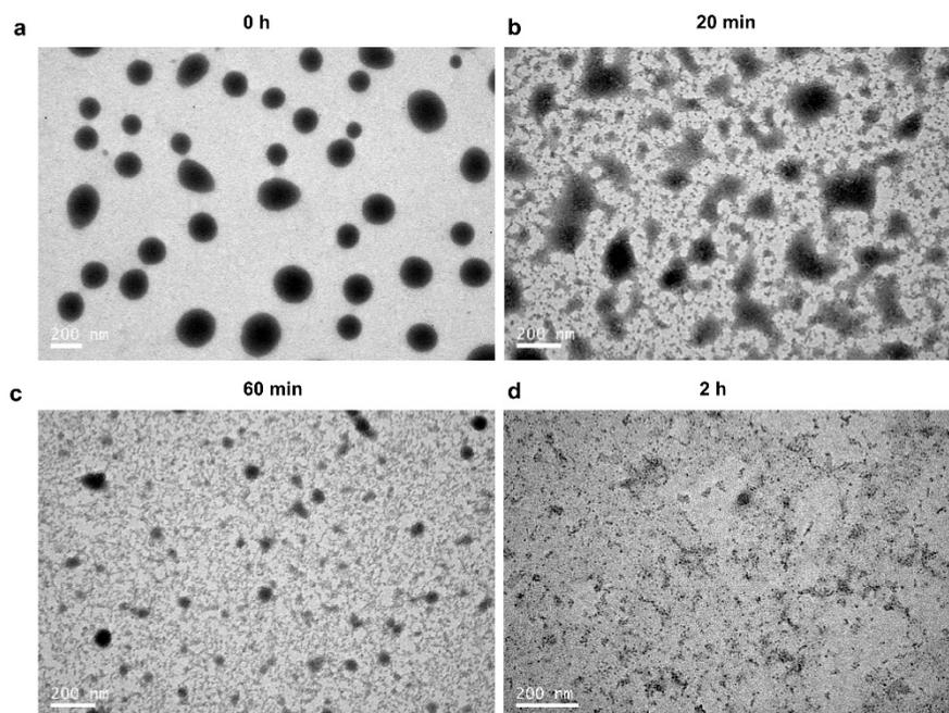
**Fig. S12** . TEM images of Ca<sup>2+</sup>-GNCs-BSA nanoparticles dispersed in acidic solution (pH ~5) for different time. a) 0 h, b) 20 min, c) 60 min and d) 2 h.
