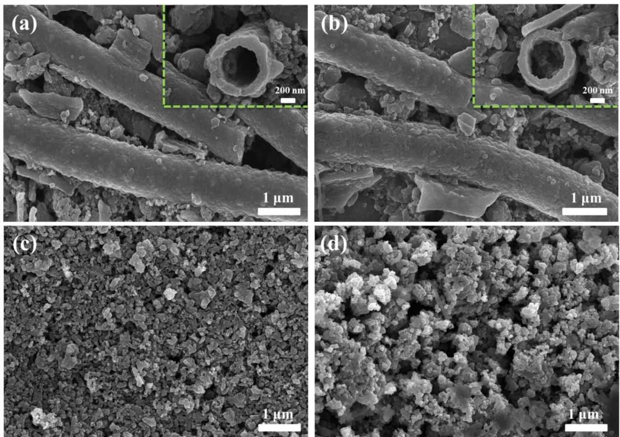
**Fig. S2.** FESEM images of HCNFs electrode (a) before and (b) after cycles for 450 cycles; FESEM images of CNPs electrode (c) before and (d) after cycles.
