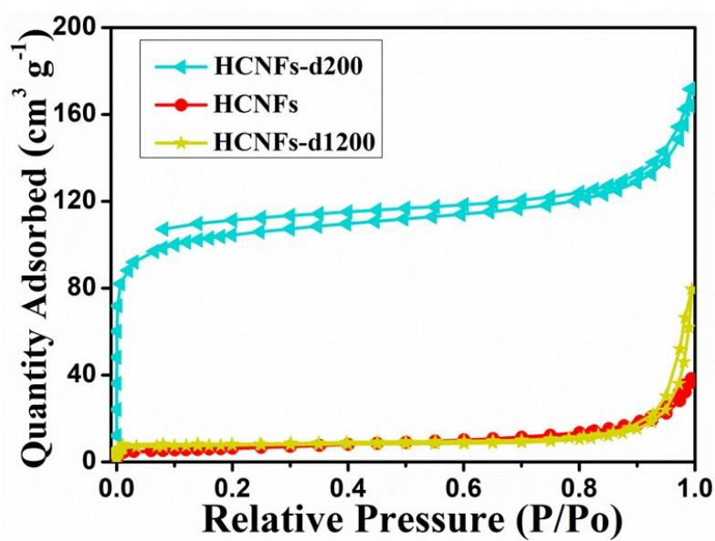
**Fig.S3.**  $\text{N}_2$  adsorption–desorption isotherms of HCNFs-d200, HCNFs and HCNFs-d1200.
