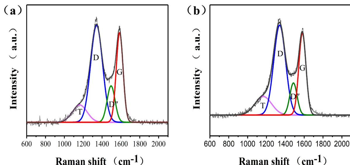
**Fig. S1.** Fitted of Raman spectra of (a) HCNFs, (b) CNPs.
