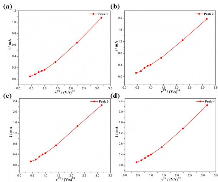
Fig. S13.  $i$  vs.  $v^{1/2}$  plots at each redox peak of CV curves for Li storage (peak current:  $i$ , scan rate:  $v$ ).
