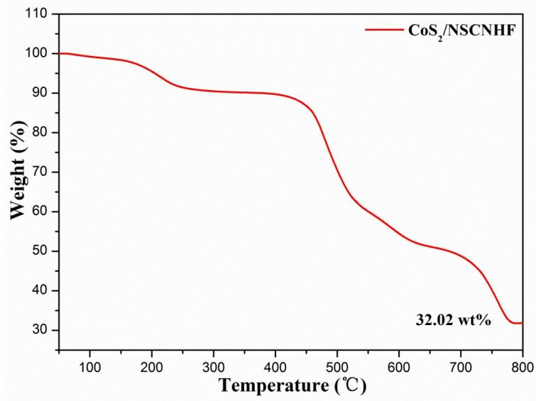
Fig. S3. TGA curve under air atmosphere.
