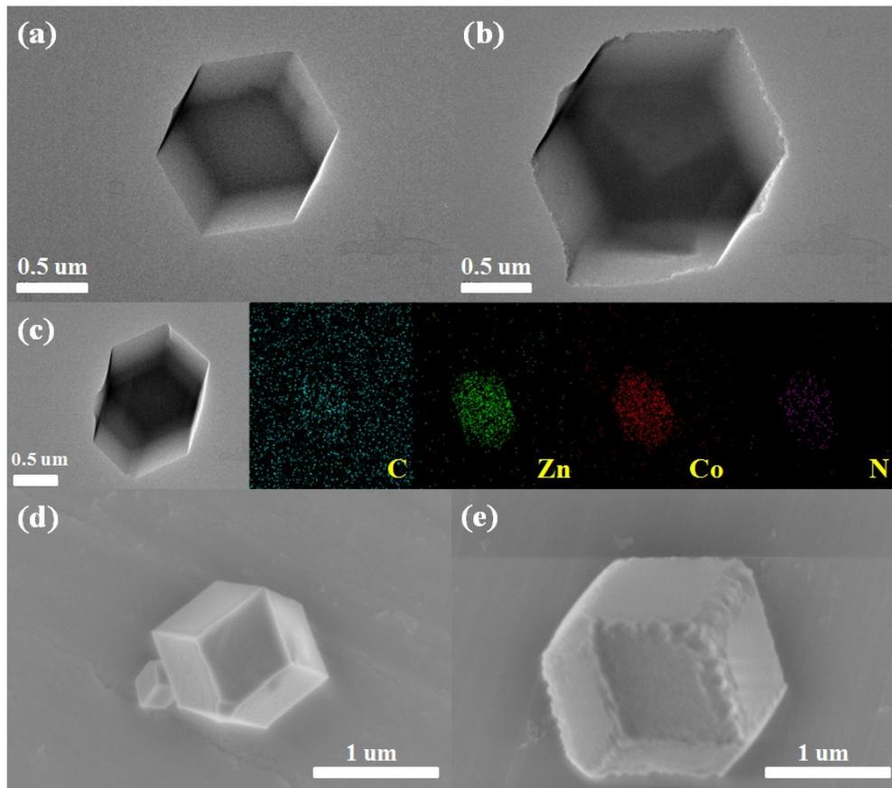
Fig. S4. (a and b) TEM images of ZIF8 and ZIF8@ZIF67; (c) TEM elemental mapping of ZIF8@ZIF67; (d and e) SEM images of ZIF8 and ZIF8@ZIF67.
