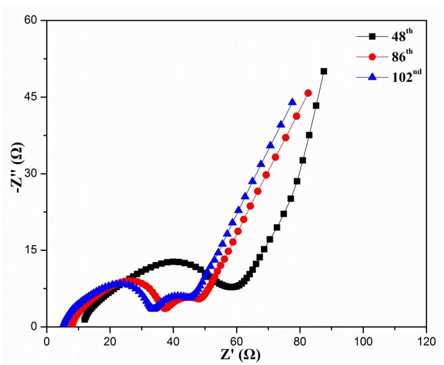
Fig. S12. Electrochemical impedance spectra (EIS) of  $\text{CoS}_2/\text{NSCNHF}$  electrode at different cycle.
