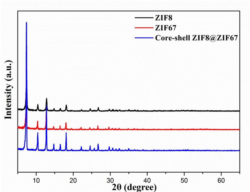
Fig. S1. XRD results of ZIF8, ZIF67 and core-shell ZIF8@ZIF67.
