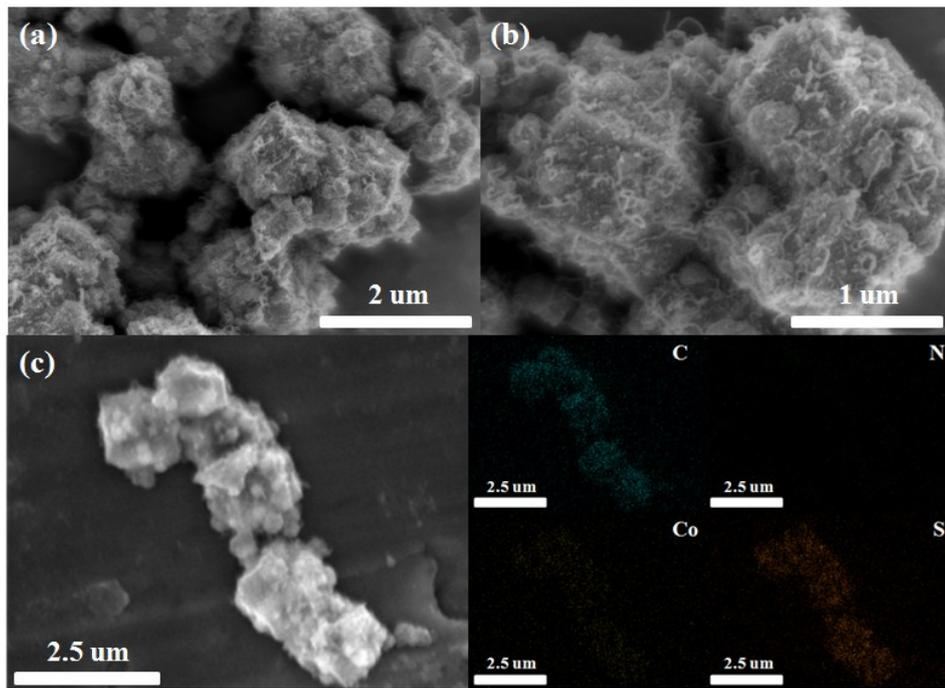
Fig. S6. (a and b) SEM images under different magnification and (c) elemental mapping results of CoS<sub>2</sub>/NSCNHF.
