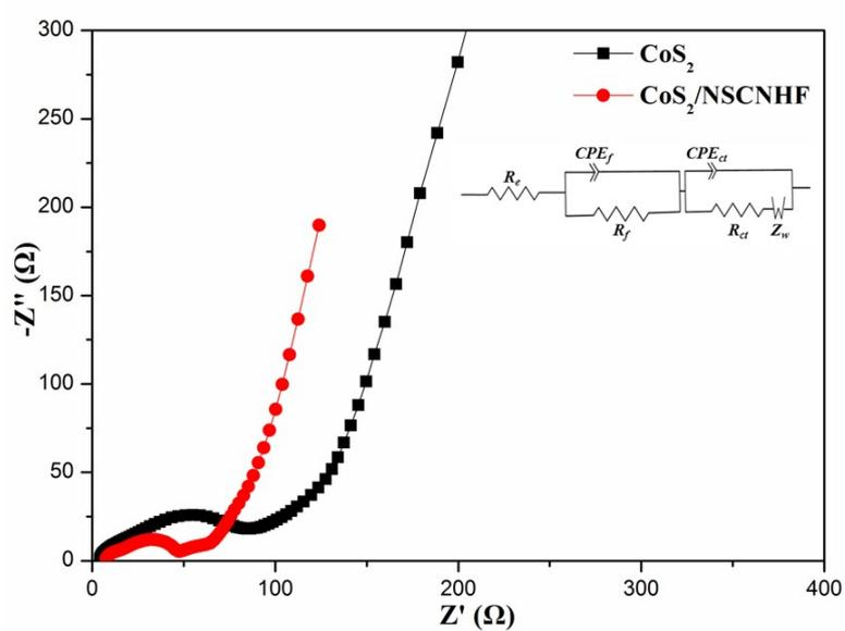
Fig. S11. Electrochemical impedance spectra (EIS) of bare  $\text{CoS}_2$  and  $\text{CoS}_2/\text{NSCNHF}$  electrode after 21 cycles.
