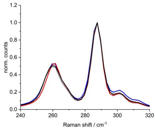
Figure S12: Radial breathing modes of SWCNT drop casted from DMF (black) or ethanol (grey) and **1**/SWCNT drop casted from DMF (red) or ethanol (blue) on a Si/SiO<sub>2</sub> surface.
