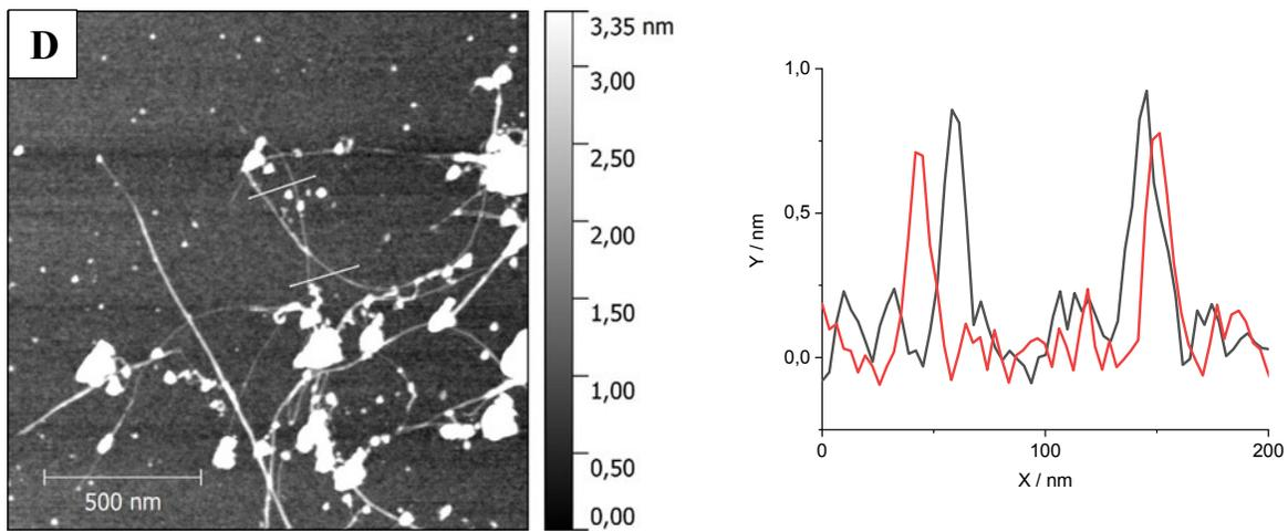
Figure S7: Tapping mode AFM images (left) and corresponding height profiles (right) of SWCNT (A) and 1/SWCNT (B) drop-casted from DMF and SWCNT (C) and 1/SWCNT (D) drop-casted from ethanol on a Si/SiO<sub>2</sub> surface.
