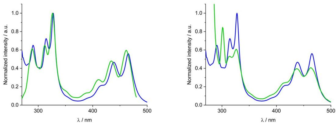
Figure S1: Absorption spectra (blue) and excitation spectra (green) of **1** recorded in DMF at 490 nm (left) and 600 nm (right).
