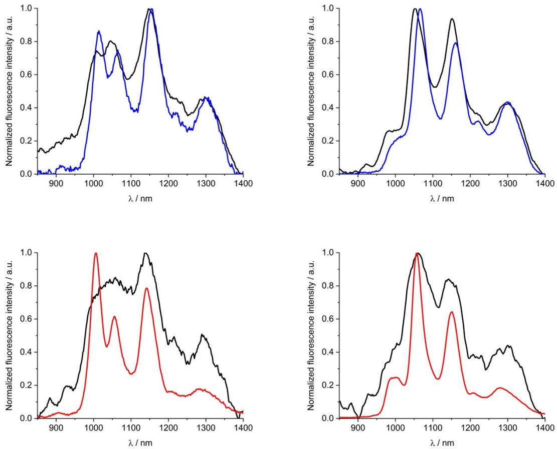
Figure S9: Normalized nIR fluorescence spectra of SWCNT (black) and 1/SWCNT in DMF (top/blue) and ethanol (bottom/red) at 585 (left) and 657nm (right) excitation.
