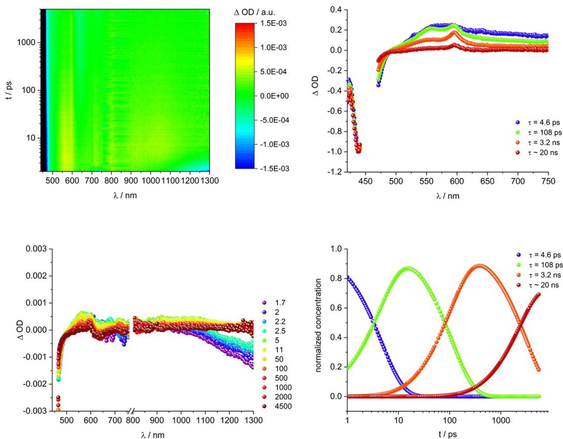
Figure S19: Differential absorption changes obtained upon femtosecond pump-probe experiments (460 nm) of 1/NG in DMF at room temperature with time delays between 2 and 5000 ps (upper left). Exemplary time evolution spectra of 1/NG in DMF at room temperature with time delays between 1.7 and 4500 ps (lower left) Corresponding evolution associated spectra of 1/NG in DMF obtained by global analysis (upper right). Corresponding concentration profiles (lower right).
