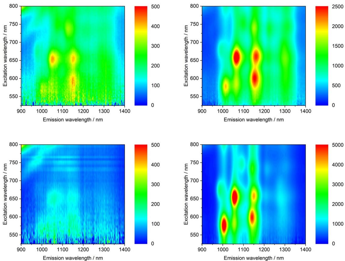
Figure S8: 3D nIR fluorescence spectra of a SWCNT reference (left) and 1/SWCNT (right) in DMF (top) and ethanol (bottom).
