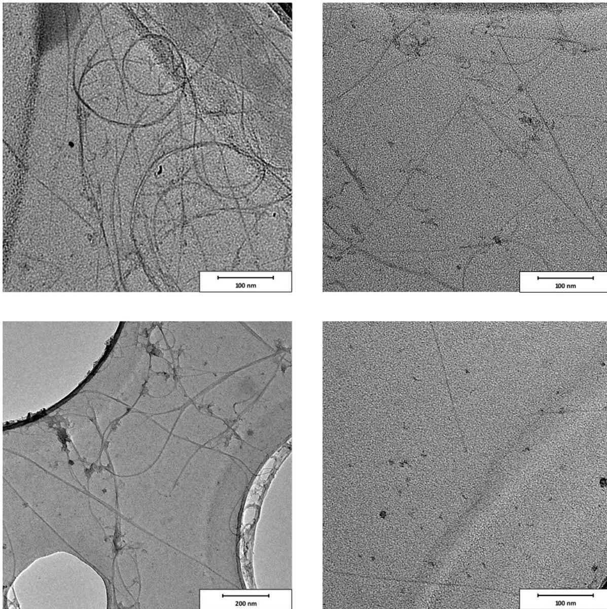
Figure S6: TEM images of a SWCNT reference (left) and 1/SWCNT (right), drop-casted on a lacey carbon grid from DMF (top) and ethanol (bottom).
