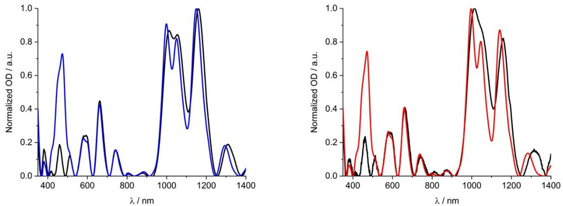
Figure S5: Normalized absorption spectra of the SWCNT reference (black) and 1/SWCNT in DMF (left/blue) and ethanol (right/red) after subtraction of the scattering background.
