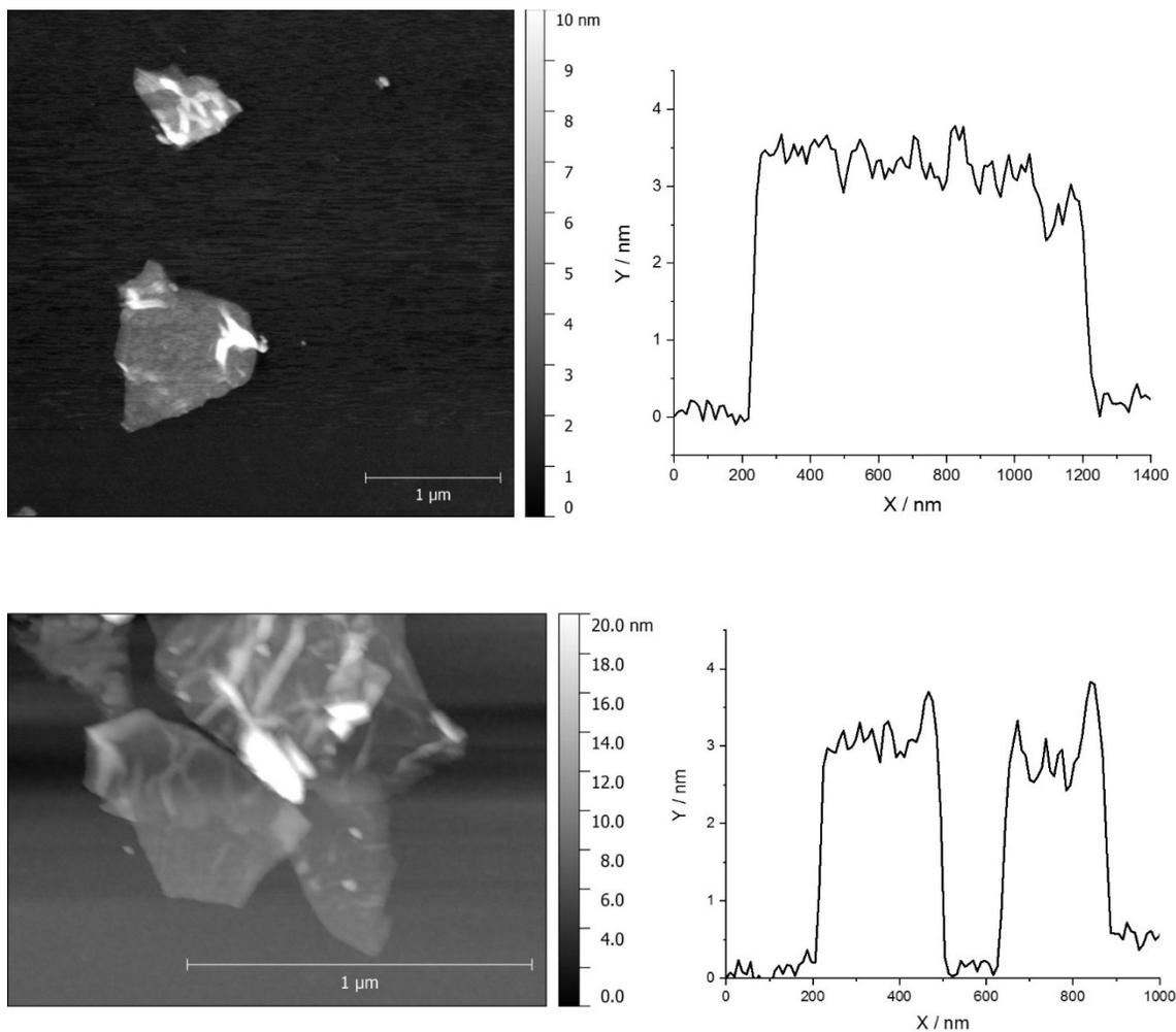
Figure S17: Tapping mode AFM images (left) and the corresponding height profiles (right) of **1/NG** (A) drop casted from DMF and **1/NG** (B) drop casted from ethanol on a Si/SiO<sub>2</sub> surface.
