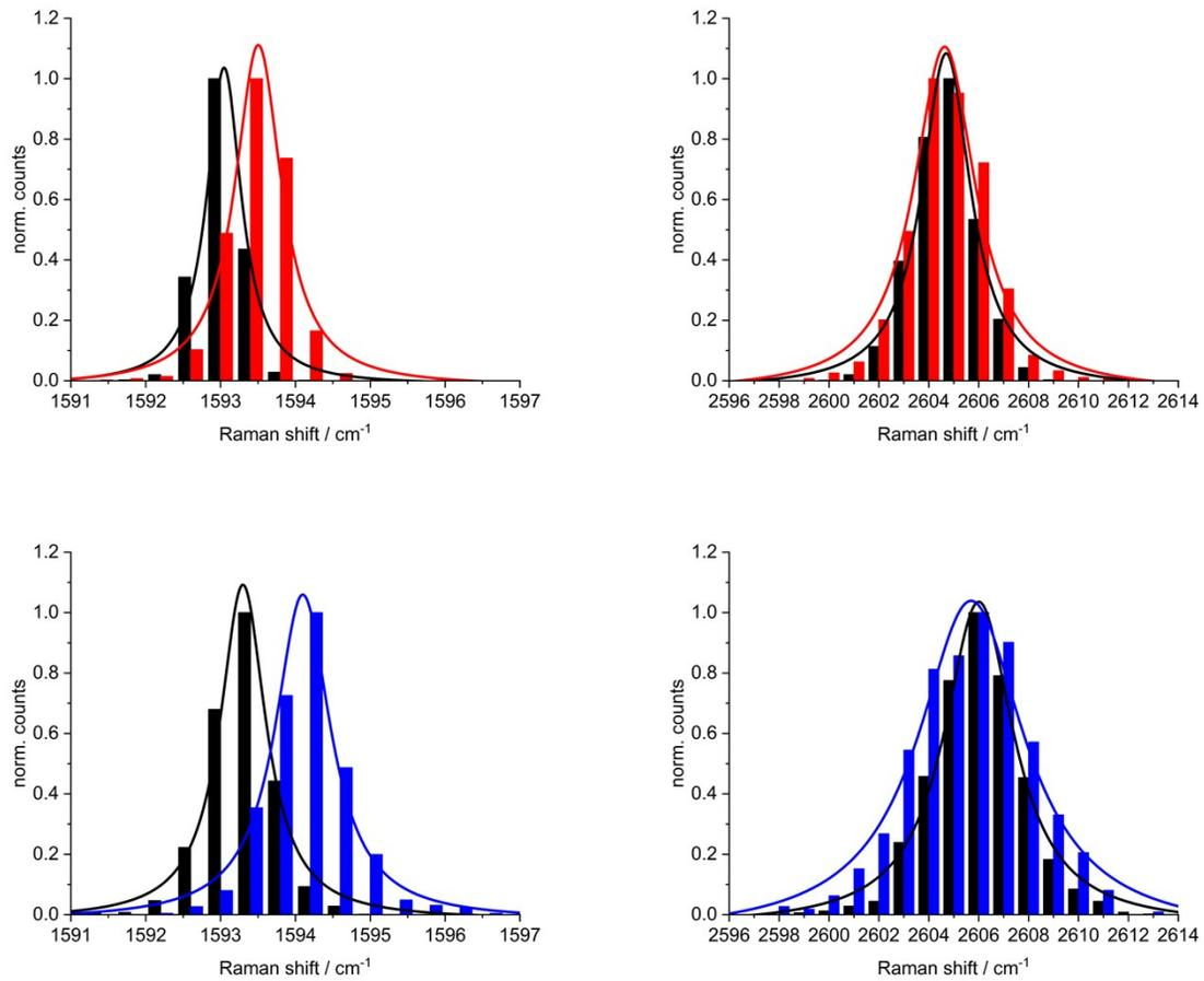
Figure S11: Histograms of Raman spectra for the G-band (left) and 2D-band (right) of the SWCNT reference (black) and 1/SWCNT (red/blue) drop casted from DMF (top) or ethanol (bottom) on a Si/SiO<sub>2</sub> surface.
