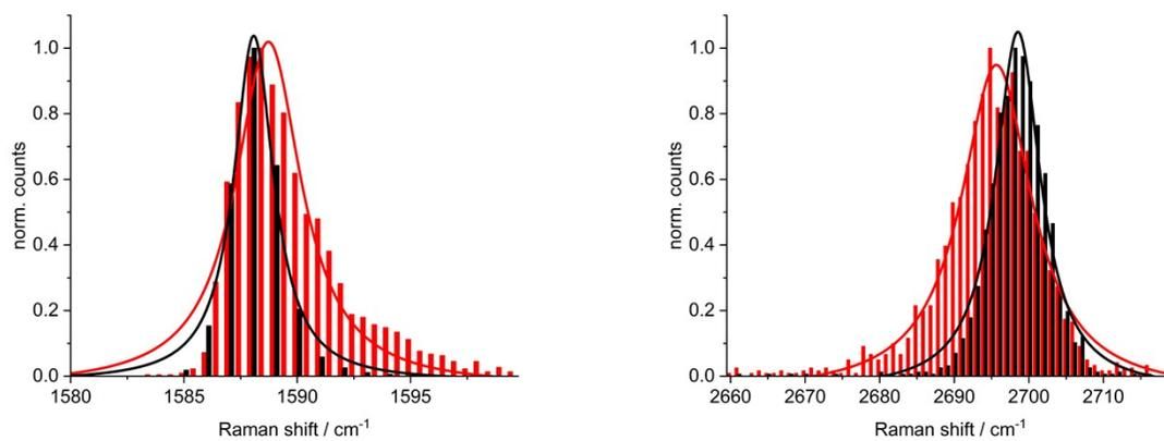
Figure S18: Histograms of Raman spectra for the G- band (left) and 2 D band (right) of the graphene reference (black) and 1/NG (red) drop casted from DMF on a Si/SiO<sub>2</sub> surface.
