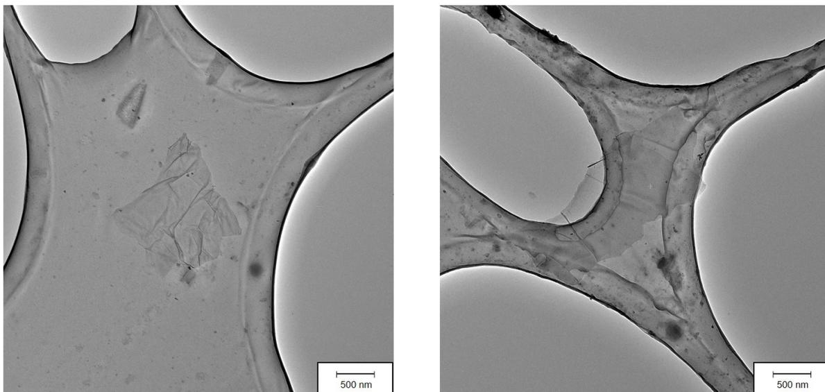
Figure S16: TEM image of 1/NG in DMF (Left) and 1/NG in ethanol (right) drop casted on a lacey carbon grid.
