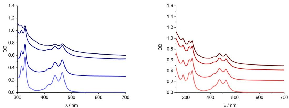
Figure S14: Absorption spectra of **1** in DMF (left) and ethanol (right) with increasing number of graphene enrichment cycles from blue/red to dark blue/dark red.
