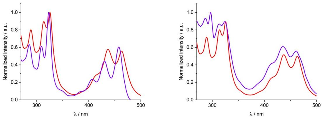
Figure S2: Absorption spectra (red) and excitation spectra (blue) of **1** recorded in ethanol at 490 nm (left) and 600 nm (right).
