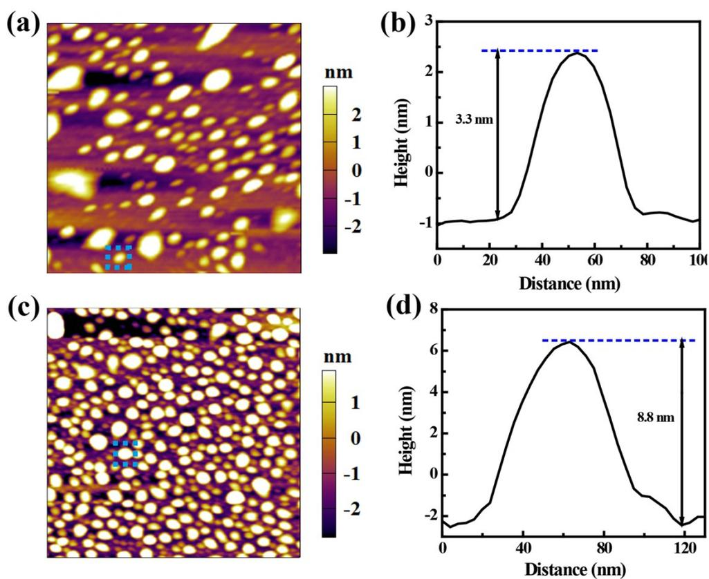
**Figure S4.** AFM images of G3.NHAc-Ad (a) and G5.NHAc-CD/Ad-G3.NHAc (c) dendrimers. Corresponding height profiles of G3.NHAc-Ad (b) and G5.NHAc-CD/Ad-G3.NHAc (d) dendrimers.
