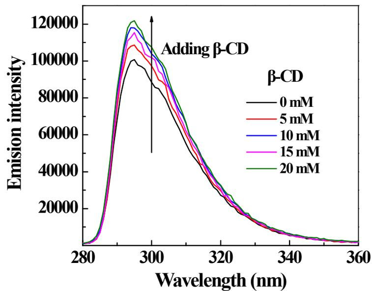
**Figure S2.** Fluorescence emission spectra of  $\beta$ -CD/BM mixture (the concentration of BM was fixed at 10 mM).
