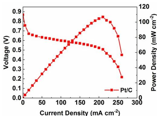
**Figure S13.** Polarization and power density curves of commercial Pt/C. Test conditions: cathode loading 2 mg<sub>Pt</sub> cm<sup>-2</sup> for commercial 60% Pt/C, anode loading 6 mg cm<sup>-2</sup> for PtRu black, Nafion® 212 membrane, 4 cm<sup>2</sup> electrode, 80 °C, 0.5 M methanol at a flow rate of 1 ml min<sup>-1</sup>, O<sub>2</sub> at a flow rate of 100 ml min<sup>-1</sup>.
