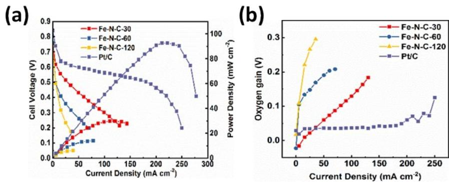
**Figure S14.** (a) DMFC single cell performance of different cathode catalysts in air and (b) oxygen gain results.
