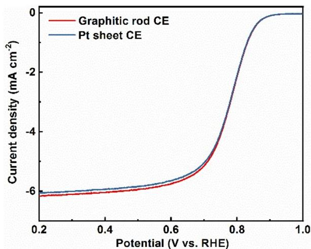
**Figure S1.** Comparison of LSV curves tested with Pt and graphite counter electrodes.
