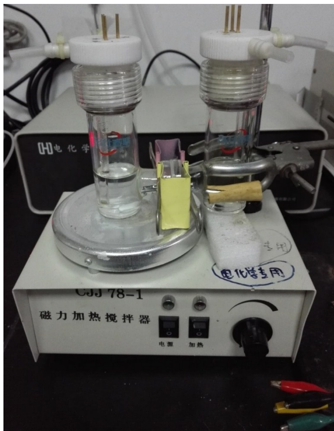
Figure S26. Photograph of the custom-designed gas-tight H-type cell for CO 2 RR.
