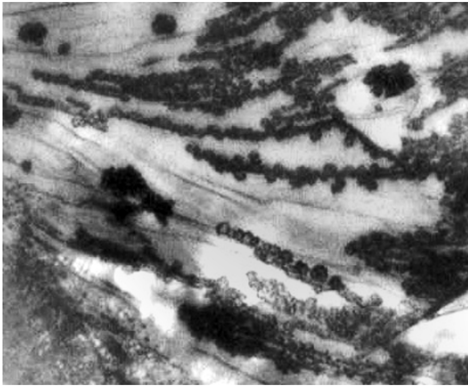
Fig. S4. Ice bands on the (010) face of feldspar. The image shows an optical frame from an experiment performed on the (010) face at -25^{\circ}\text{C} under AH_{\text{in}} = 1.18 \text{ g/m}^3 . As in the case of the (001) face, dark bands extending across the image are ice, which abruptly appeared and immediately started consuming the small droplets of liquid water that had initially covered the entire surface.
