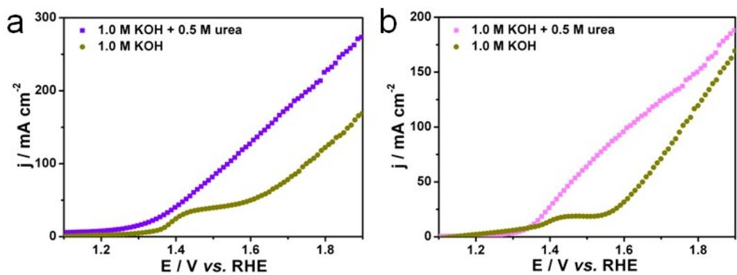
**Fig. S9** Polarization curves for UOR and OER of the as-prepared (a) a-MoS<sub>2</sub>/CoS HNSs and (b) Co<sub>0.85</sub>Se NRs.
