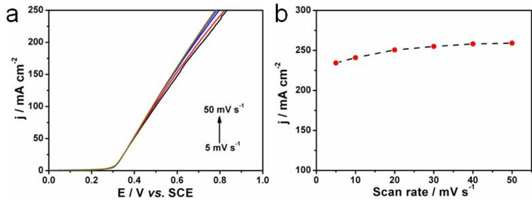
**Fig. S14** (a) UOR polarization curves of the a-MoS<sub>2</sub>/CoS/Co<sub>0.85</sub>Se HNTs electrode at different scan rates. (b) The corresponding current densities at 0.8 V versus SCE with different scan rates.
