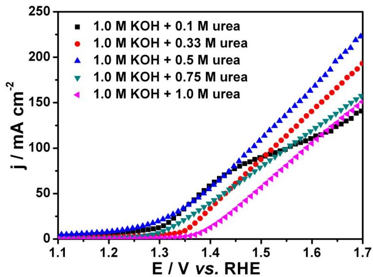
**Fig. S8** Polarization curves of the a-MoS<sub>2</sub>/CoS/Co<sub>0.85</sub>Se HNTs in 1.0 M KOH with different urea concentration.
