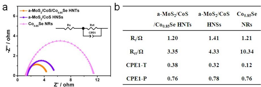
**Fig. S11** (a) Nyquist plots of the a-MoS<sub>2</sub>/CoS/Co<sub>0.85</sub>Se HNTs, a-MoS<sub>2</sub>/CoS HNSs and Co<sub>0.85</sub>Se NRs and (b) the corresponding EIS data for UOR.
