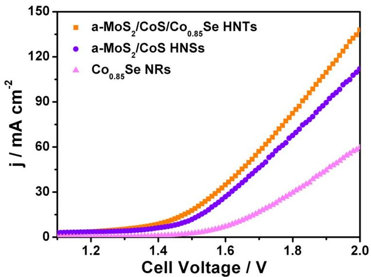
**Fig. S21** Polarization curves for the as-prepared a-MoS<sub>2</sub>/CoS/Co<sub>0.85</sub>Se HNTs, a-MoS<sub>2</sub>/CoS HNSs and Co<sub>0.85</sub>Se NRs electrodes in 1.0 M KOH with 0.5 M urea.
