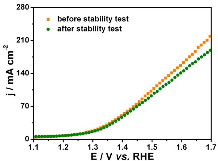
**Fig. S16** Polarization curves of the as-prepared a-MoS<sub>2</sub>/CoS/Co<sub>0.85</sub>Se HNTs electrode before and after long-term stability test.
