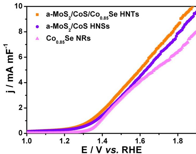
**Fig. S13** UOR polarization curves of the different samples normalized by ECSA.
