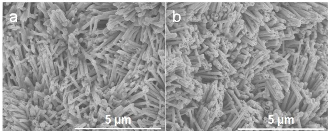
**Fig. S22** SEM images of the as-prepared a-MoS<sub>2</sub>/CoS/Co<sub>0.85</sub>Se HNTs electrode after (a) UOR and (b)HER.
