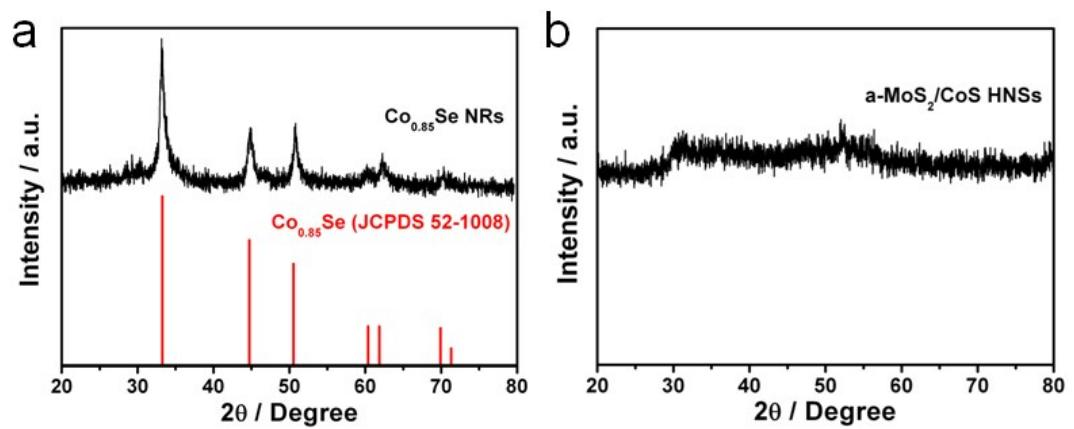
**Fig. S5** XRD patterns of the as-prepared (a)  $\text{Co}_{0.85}\text{Se NRs}$  and (b)  $\text{a-MoS}_2/\text{CoS HNSs}$ .
