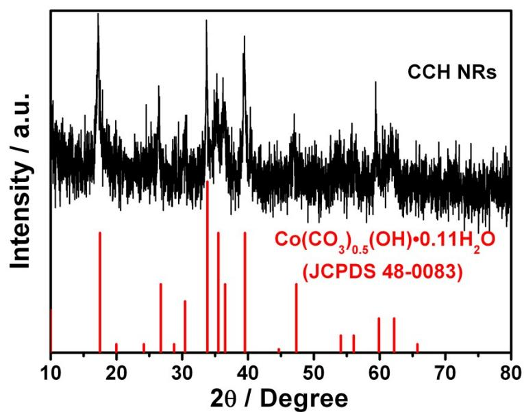
**Fig. S2** XRD pattern of the as-prepared CCH NRs.
