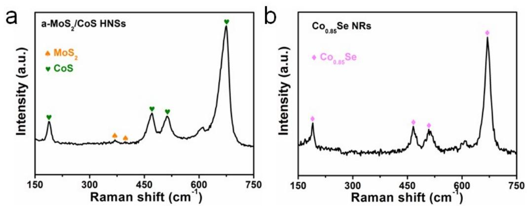
**Fig. S6** Raman spectra of the as-prepared (a) a-MoS<sub>2</sub>/CoS HNSs and (b) Co<sub>0.85</sub>Se NRs.
