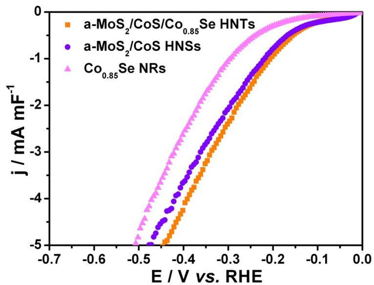
**Fig. S19** HER polarization curves of the different samples normalized by ECSA.
