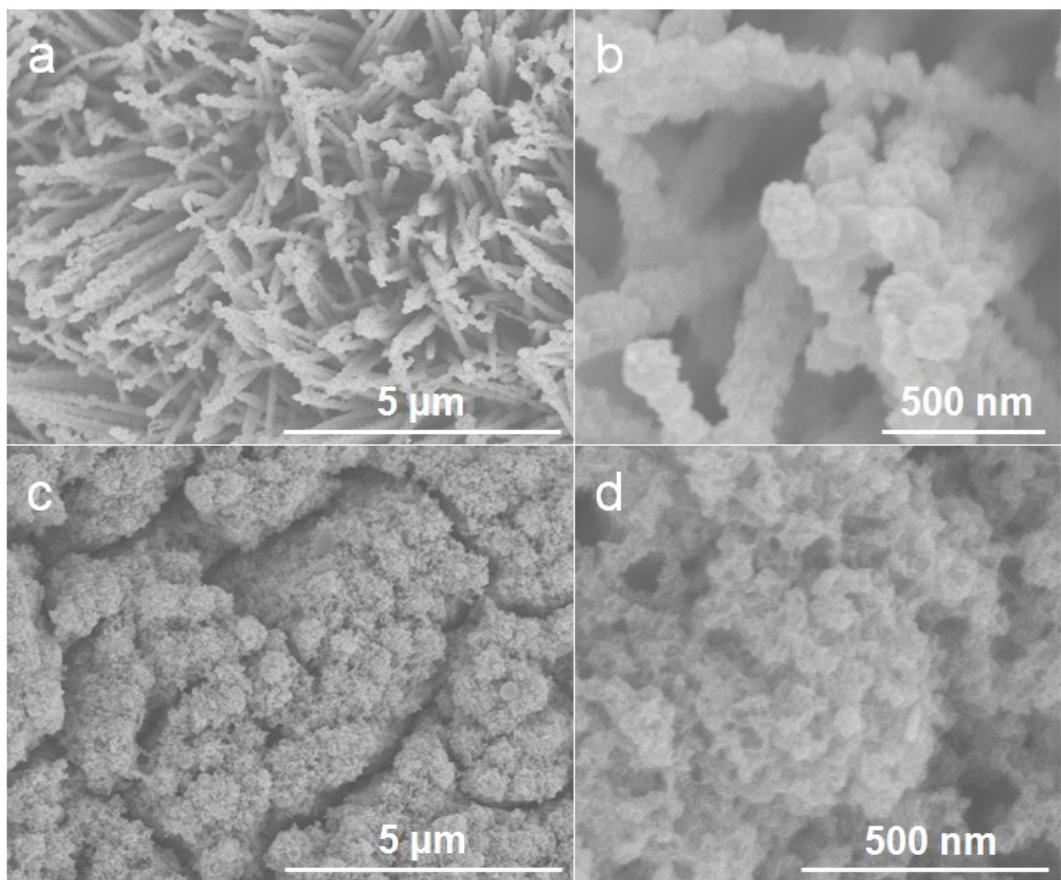
**Fig. S3** SEM images of the as-prepared (a, b)  $\text{Co}_{0.85}\text{Se}$  NRs and (c, d) a- $\text{MoS}_2/\text{CoS}$  HNSs.
