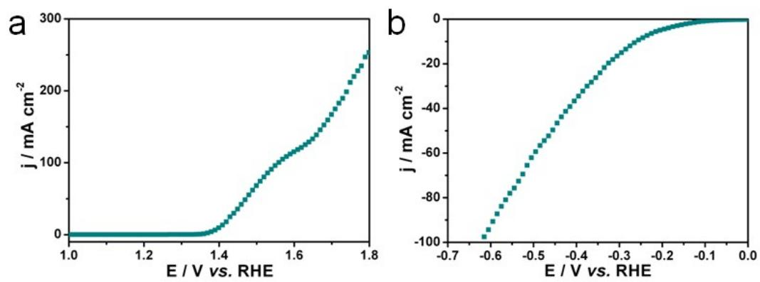
**Fig. S10** Polarization curves of NF towards (a) UOR and (b) HER in 1.0 M KOH with 0.5 M urea.
