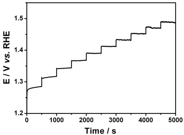
**Fig. S15** Multi-current process of a-MoS<sub>2</sub>/CoS/Co<sub>0.85</sub>Se HNTs electrode. The current density started at 10 mA cm<sup>-2</sup> and ended at 110 mA cm<sup>-2</sup> with an increment of 10 mA cm<sup>-2</sup> per 500 s.
