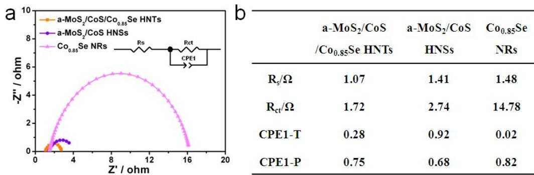
**Fig. S18** (a) Nyquist plots of the a-MoS<sub>2</sub>/CoS/Co<sub>0.85</sub>Se HNTs, a-MoS<sub>2</sub>/CoS HNSs and Co<sub>0.85</sub>Se NRs electrodes and (b) the corresponding EIS data for HER.
