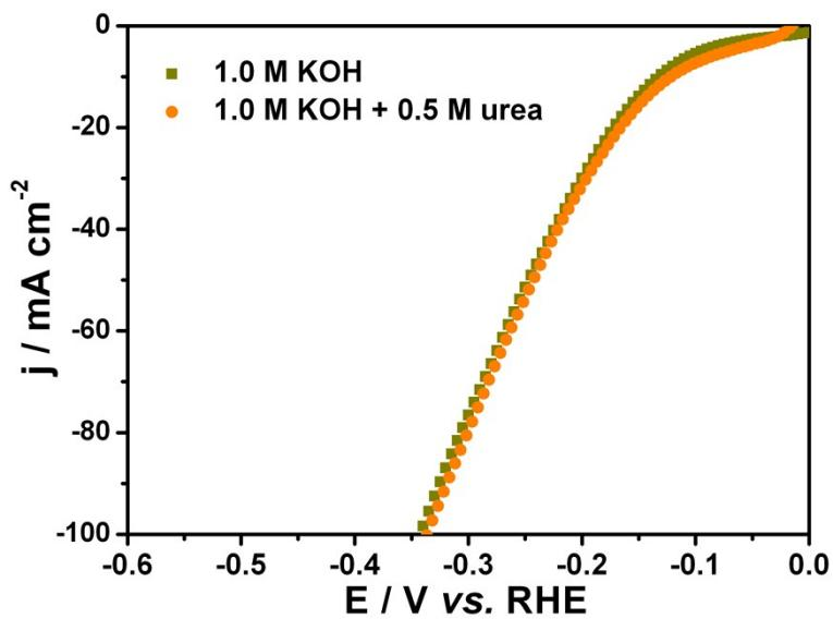
**Fig. S20** Polarization curves of the as-prepared a-MoS<sub>2</sub>/CoS/Co<sub>0.85</sub>Se HNTs in 1.0 M KOH with and without 0.5 M urea.
