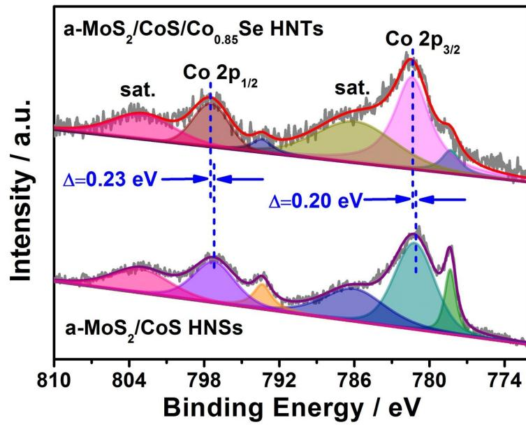
**Fig. S7** High-resolution XPS spectra of Co 2p for the  $\text{a-MoS}_2/\text{CoS}/\text{Co}_{0.85}\text{Se}$  HNTs and  $\text{a-MoS}_2/\text{CoS}$  HNSs.
