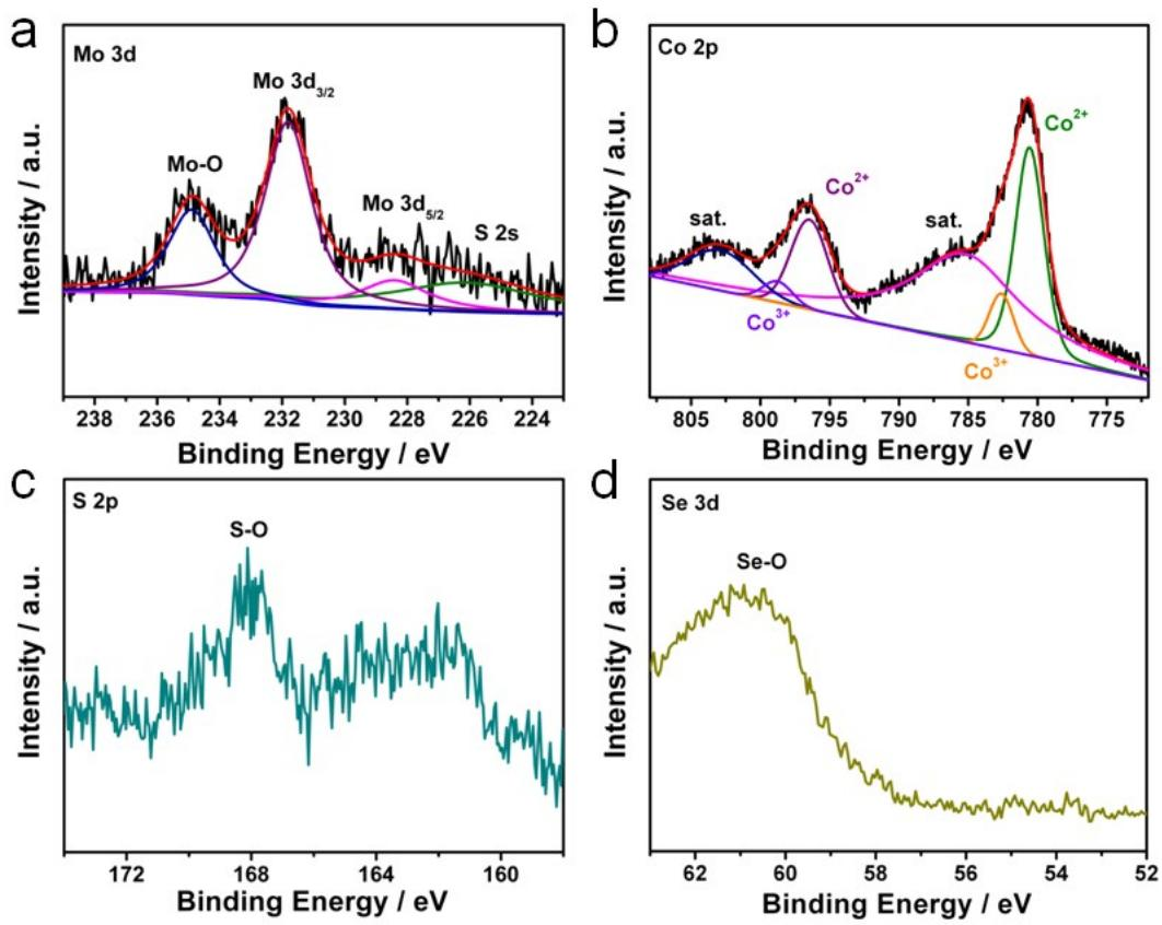
**Fig. S23** High-resolution XPS spectra of a) Mo 3d, b) Co 2s, c) S 2p and e) Se 3d for the as-prepared a-
