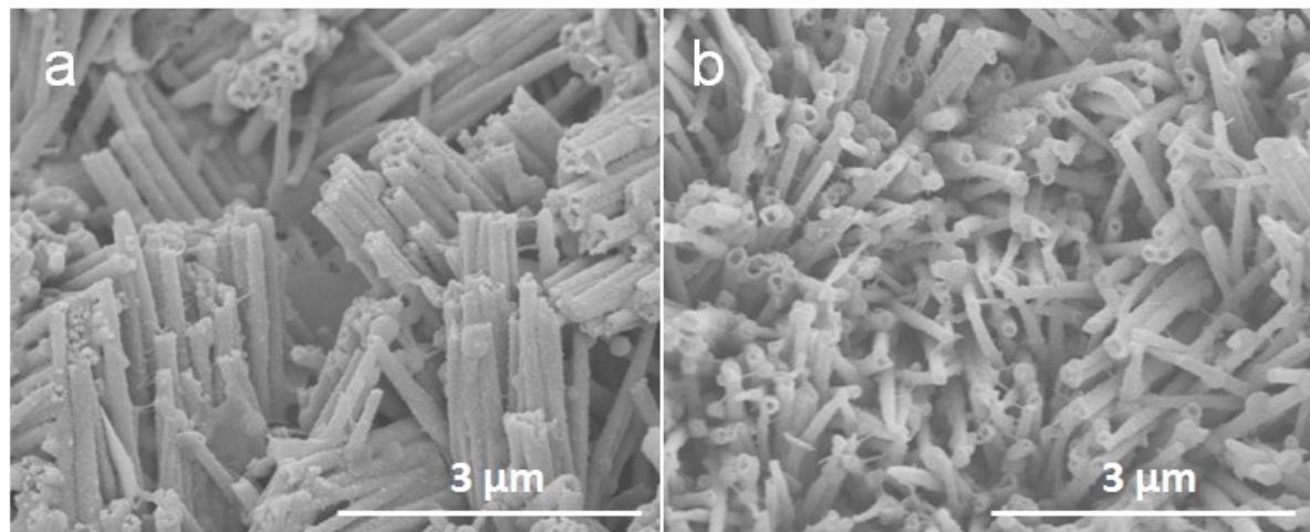
**Fig. S17** SEM images of the a-MoS<sub>2</sub>/CoS/Co<sub>0.85</sub>Se HNTs electrode after long-term stability test for (a) UOR and (b) HER.
