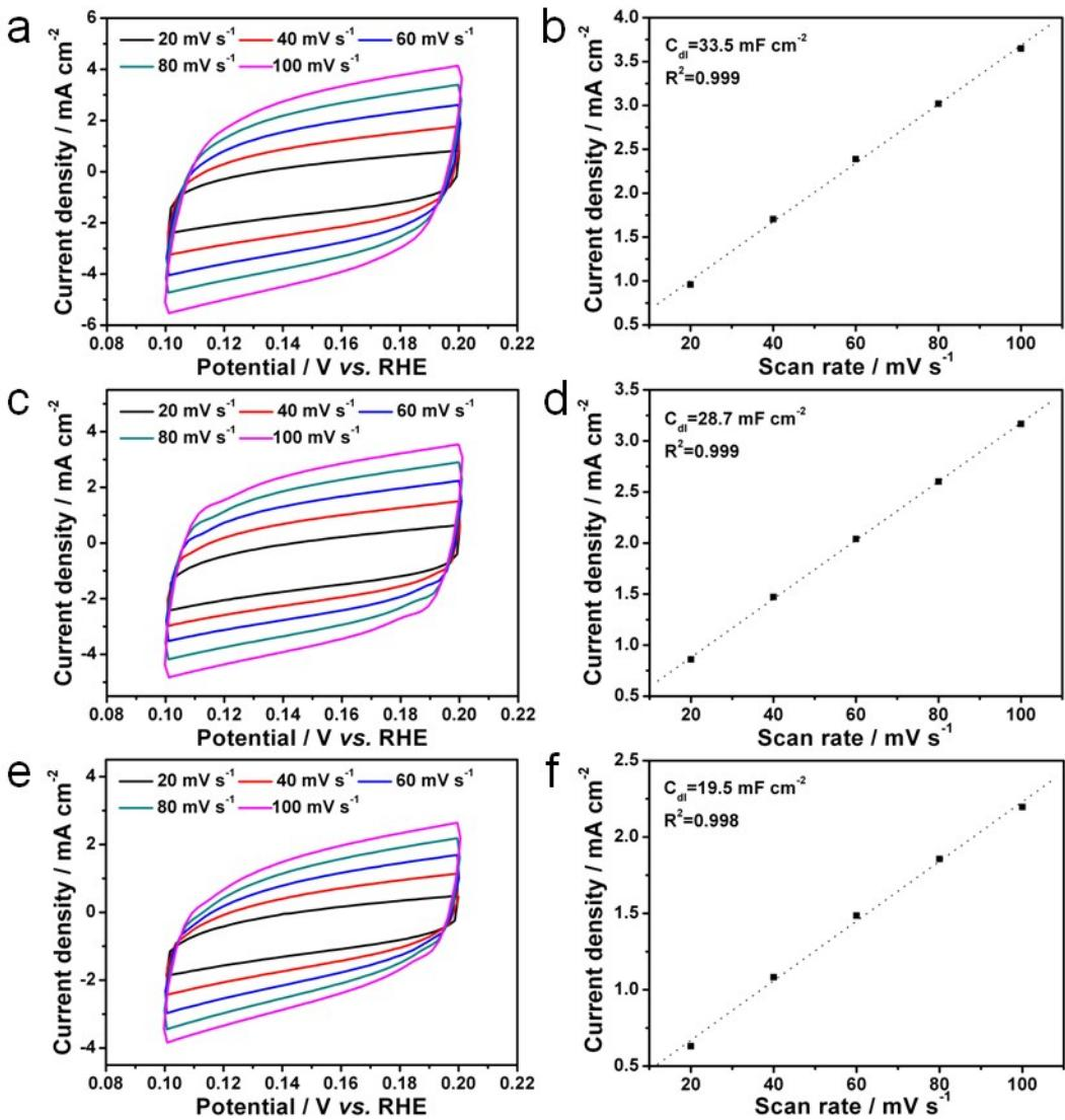
**Fig. S12** CV curves and the plots of current density as a function of scan rate: (a, b) a-MoS<sub>2</sub>/CoS/Co<sub>0.85</sub>Se HNTs, (c, d) a-MoS<sub>2</sub>/CoS HNSs and (e, f) Co<sub>0.85</sub>Se NRs electrodes in the double layer region at scan rates of 20, 40, 60, 80 and 100 mV s<sup>-1</sup> in 1.0 M KOH with 0.5 M urea.
