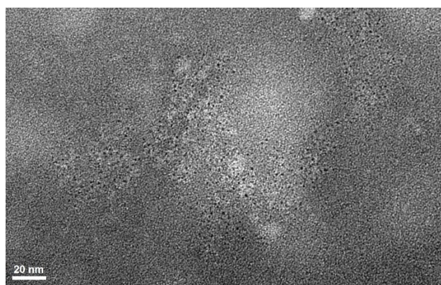
Fig. S13 TEM image of the negative stained HSA in the presence of four equivalents of the DHLA-AuNCs. White components represent HSA while black dots represent AuNCs.
