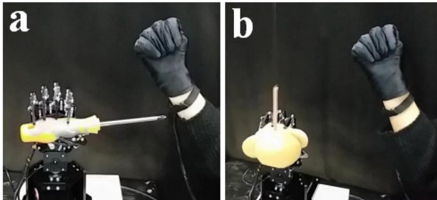
**Fig. S7** Photographs showing the smart glove control a hand robot to (a) hold still object and (b) grasp a moving toy.
