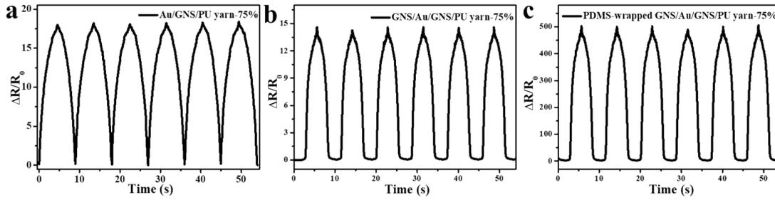
**Fig. S4** Resistance-time relationships under six stretching/releasing cycles with an applied strain of 75%: (a) Au/GNS/PU yarn (GF: 23.96), (b) GNS/Au/GNS/PU yarn (GF: 19.55), (c) PDMS-wrapped GNS/Au/GNS/PU yarn (GF: 668.33).
