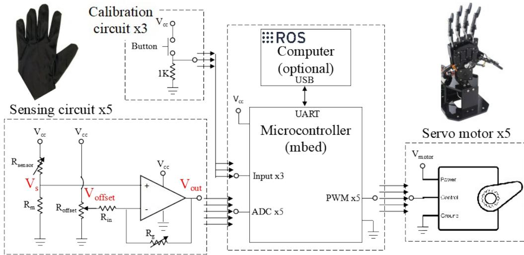
**Fig. S6** Schematic diagram of the wearable sensor platform for human-machine interface. Each strain sensor in the glove was connected to a sensing circuit and microcontroller to map the normalized signal voltage value into rotation angle of the servo motor on the corresponding finger of the robotic hand. A separate calibration circuit provides personalized tuning for the voltage mapping of the fingers. Optionally, the signals can be displayed on computer that runs Robot Operating System.
