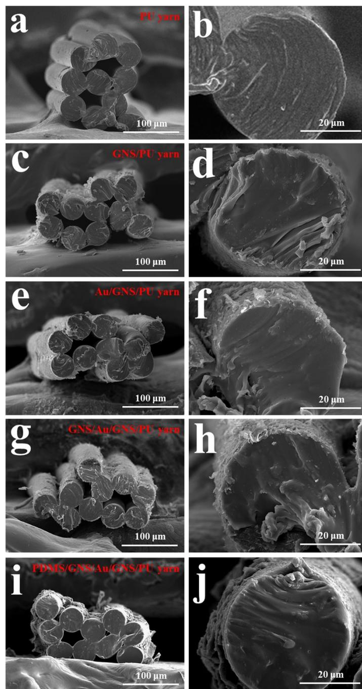
**Fig. S3** The cross-sectional FESEM images of (a, b) PU yarn, (c, d) GNS/PU yarn, (e, f) Au/GNS/PU yarn, (g, h) GNS/Au/GNS/PU yarn, and (i, j) PDMS-wrapped GNS/Au/GNS/PU yarn. The PU yarn is consisted of a group of monofilaments with average diameters of approximately 40  $\mu\text{m}$ .
