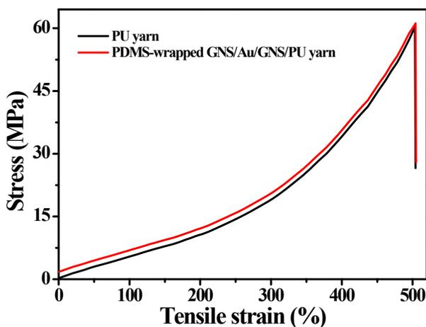
**Fig. S2** Tensile properties of PU yarn and the resultant PDMS-wrapped GNS/Au/GNS/PU yarn. It compares the stress-strain curves of the PU yarn and the resultant strain sensor. The PU yarn and the resultant strain sensor can be stretched to approximately 500% until breakage, which indicates that the multilayer sheath and PDMS wrapping layer had no apparent influence on the inherent outstanding mechanical property.
