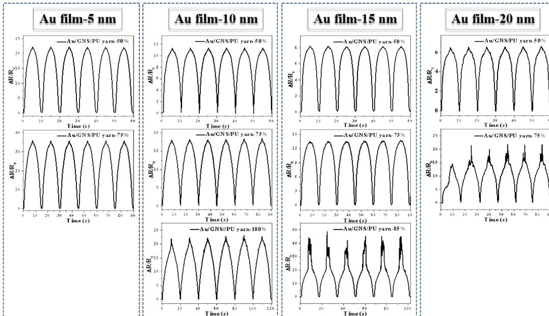
**Fig. S5** Electro-mechanical properties of Au/GNS/PU yarn with different thicknesses of Au films. Comparing with the GNS/PU yarns coated with 5 nm, 15 nm, and 20 nm Au films, the GNS/PU yarn coated with 10 nm Au film possesses a wider and more stable working (strain-sensing) range (up to 100%), therefore, in this manuscript, we chose the 10 nm Au film as the inter layer.
