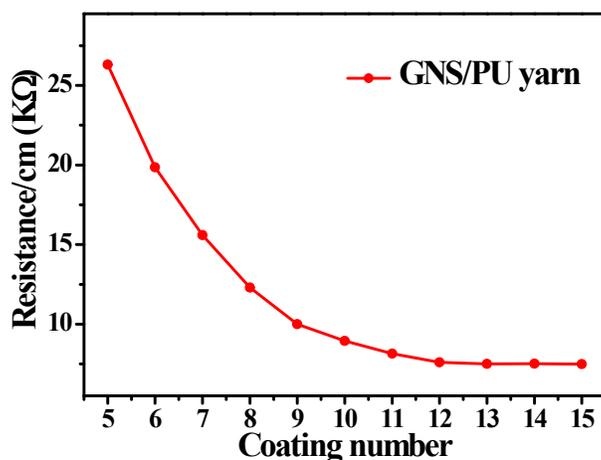
**Fig. S1** Resistance changes of GNS/ PU yarn with different number of GNS coating. The electrical resistance of GNS/PU yarn decreases with the increase of number of GNS coating (from 5 to 12) until it reaches to a stable condition (from 12 to 15). That is say, when the number of GNS coating increased to 12, the GNS layer has been achieved to a highly conductive and stable state, and thereby enabling the electro-mechanical properties reach to a stable state.
