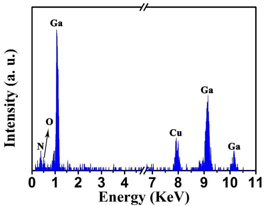
**Figure S9.** EDS spectrum of a randomly selected individual GaN nanowire grown at 1050 °C.
