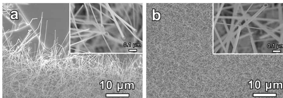
**Figure S3.** SEM images of GaN nanowires grown at 980 °C and GaCl<sub>3</sub> flow rate of 10 sccm under different NH<sub>3</sub> flow rate: (a) 30 sccm and (b) 15 sccm.
