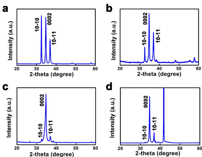
**Figure S1.** XRD patterns of GaN nanowires grown at 980 °C under GaCl<sub>3</sub> flux rate of (a) 40 sccm, (b) 30 sccm, (c) 15 sccm and (d) 10sccm, respectively.
