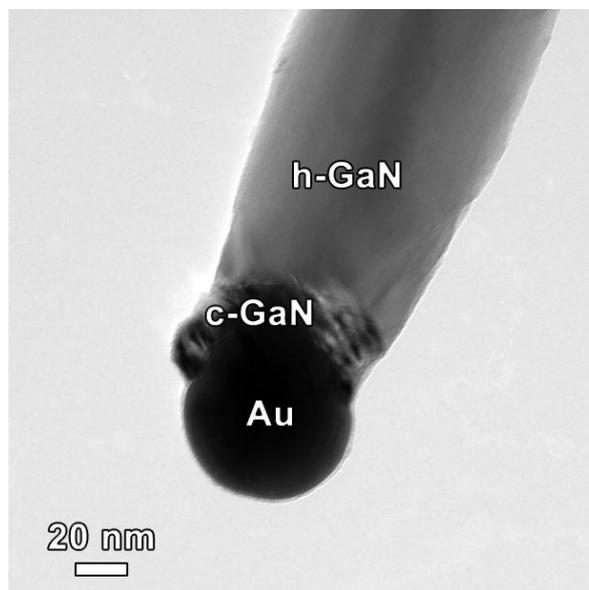
**Figure S7.** Low-magnification TEM image of an individual GaN nanowire grown at 980 °C
