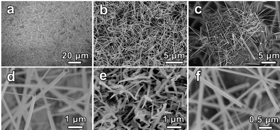
**Figure S4.** SEM images of GaN nanowires grown under fixed GaCl<sub>3</sub> flow rate of 10 sccm under (a, d) 980 °C, NH<sub>3</sub> flow rate of 15 sccm; (b, e) 900 °C, NH<sub>3</sub> flow rate of 15 sccm; (c, f) 900 °C, NH<sub>3</sub> flow rate of 30 sccm.
