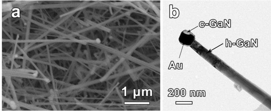
**Figure S6.** SEM and low-magnification TEM images of nonpolar GaN nanowires grown at 1050 °C.
