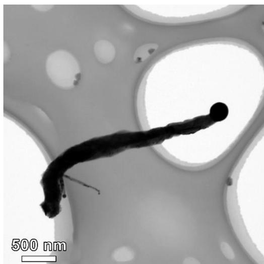
**Figure S2.** Low magnification TEM image of an individual GaN nanowire corresponding to **Figure 2b.**
