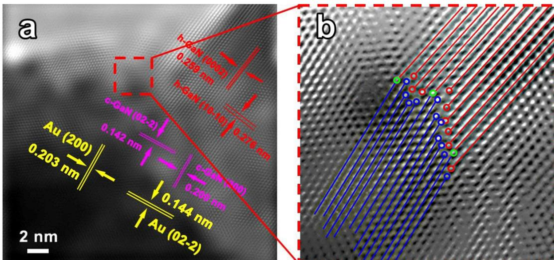
**Figure S5.** (a) IFFT pattern of Au/GaN interface corresponding to 900 °C grown GaN nanowire; (b) enlarged IFFT pattern showing lattice mismatching between cubic GaN and hexagonal GaN.
