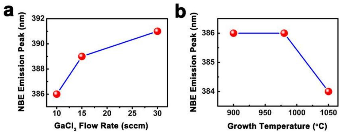
**Figure S8.** Effect of (a) GaCl<sub>3</sub> flow rate and (b) growth temperature on the near-band emission
