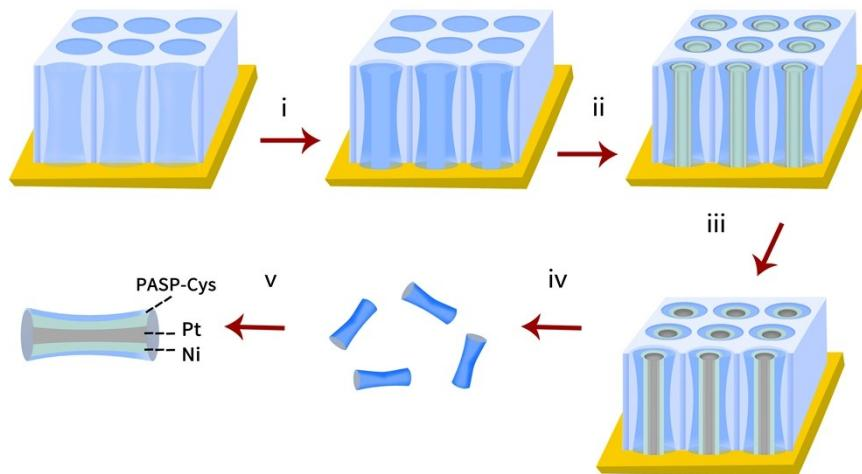
**Fig. 1S.** Preparation process of PAsp-Cys/Ni/Pt micromotors.
