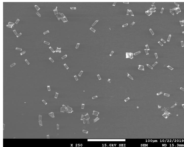
**Fig. 2S** SEM image of PAsp-Cys/Ni/Pt micromotors
