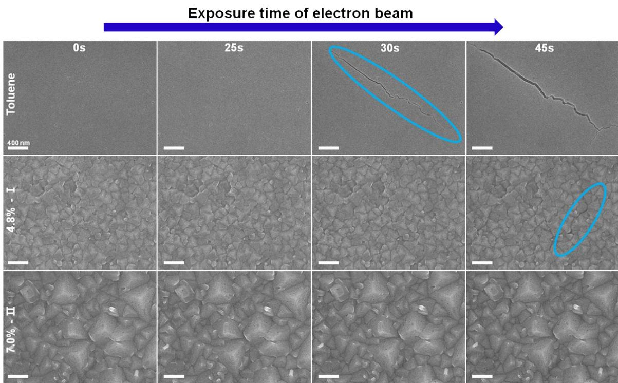
**Supplementary Figure S8.** Time-dependent SEM images of MAPbBr<sub>3</sub> films formed by toluene and with seed concentrations of 4.8% and 7.0% under irradiation by an electron beam.
