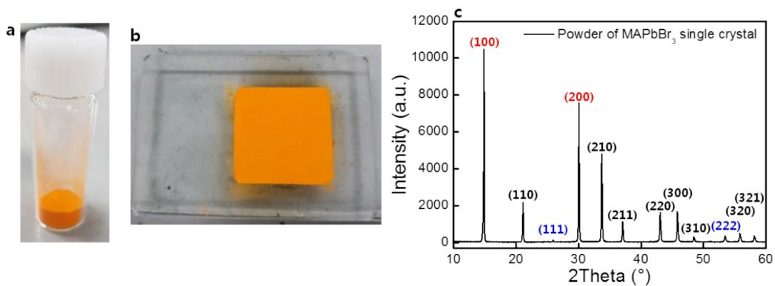
**Supplementary Figure S4.** Photographs of a) the powder of the MAPbBr<sub>3</sub> single crystal and b) the uniform setting of the powder. c) XRD pattern of the powder of the MAPbBr<sub>3</sub> single crystal for the calculation of the texture coefficient.
