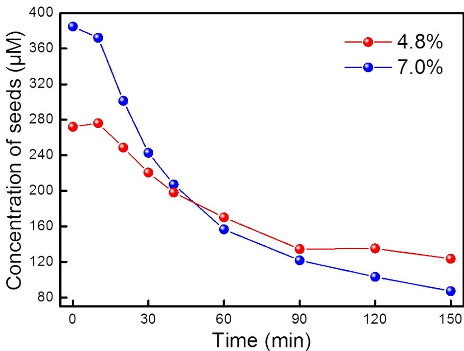
**Supplementary Figure S5.** Calculated concentration of seeds with respect to the aggregation time (4.8% and 7.0% seeds). It was calculated using the reported molar extinction coefficient [*ACS Energy Letters* **2017**, 2, 88] and lattice constant [*Nano Letters* **2015**, 15, 5191] of MAPbBr<sub>3</sub> QDs.
