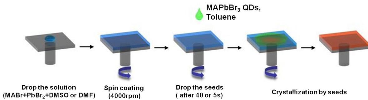
**Supplementary Figure S1.** Crystallization process with perovskite seeds.
