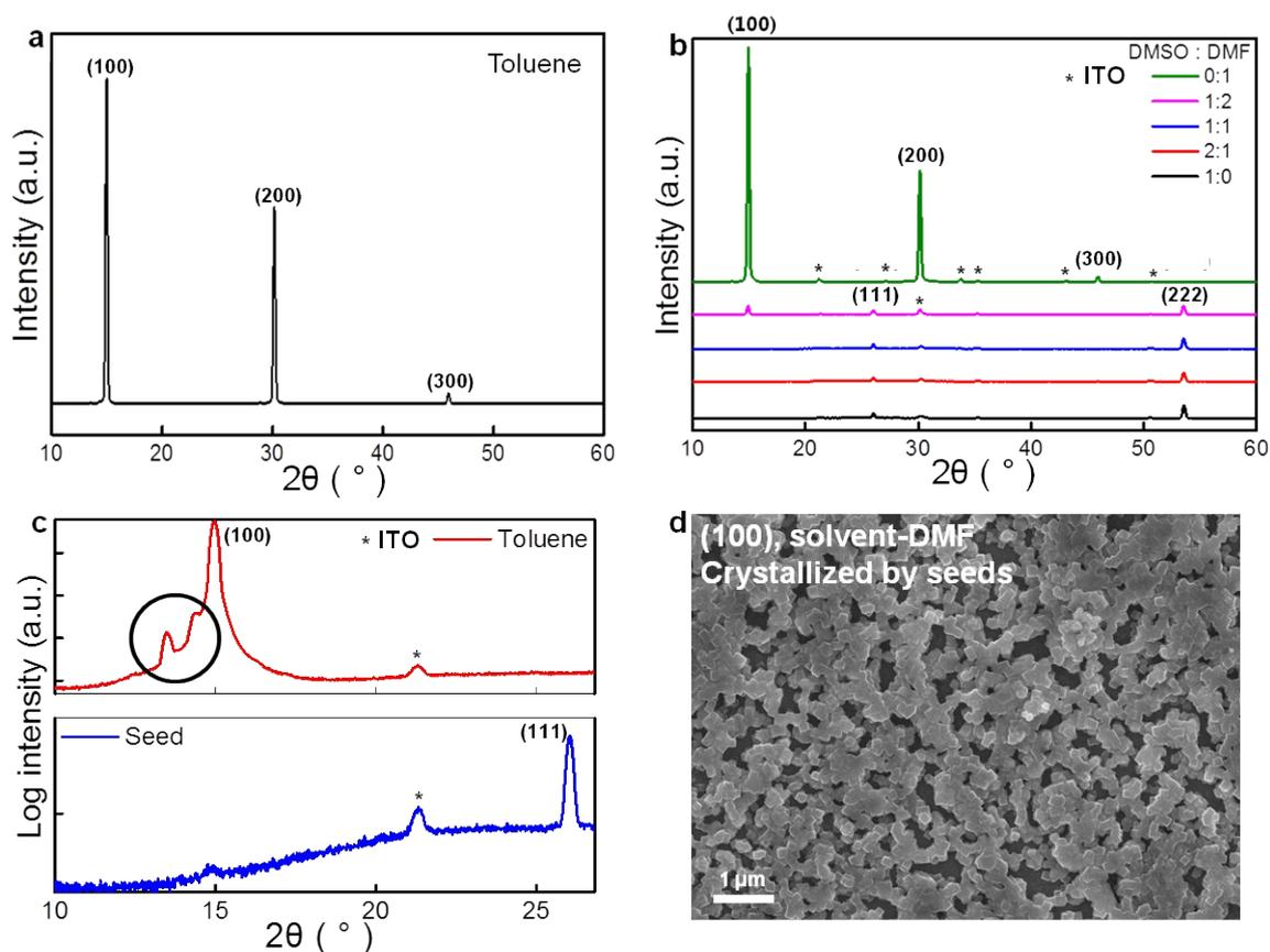
**Supplementary Figure S2.** XRD pattern of a) the film formed by toluene and b) the films formed by seeds with different ratios of DMSO to DMF in the perovskite solution. c) Log-scale XRD pattern of the (100) plane for the film formed by toluene and the (111) plane for the film formed by seeds. d) SEM image of the film formed by seeds. The solvent of the perovskite solution was DMF. Owing to the rapid evaporation of DMF, it was difficult to produce full-coverage films.
