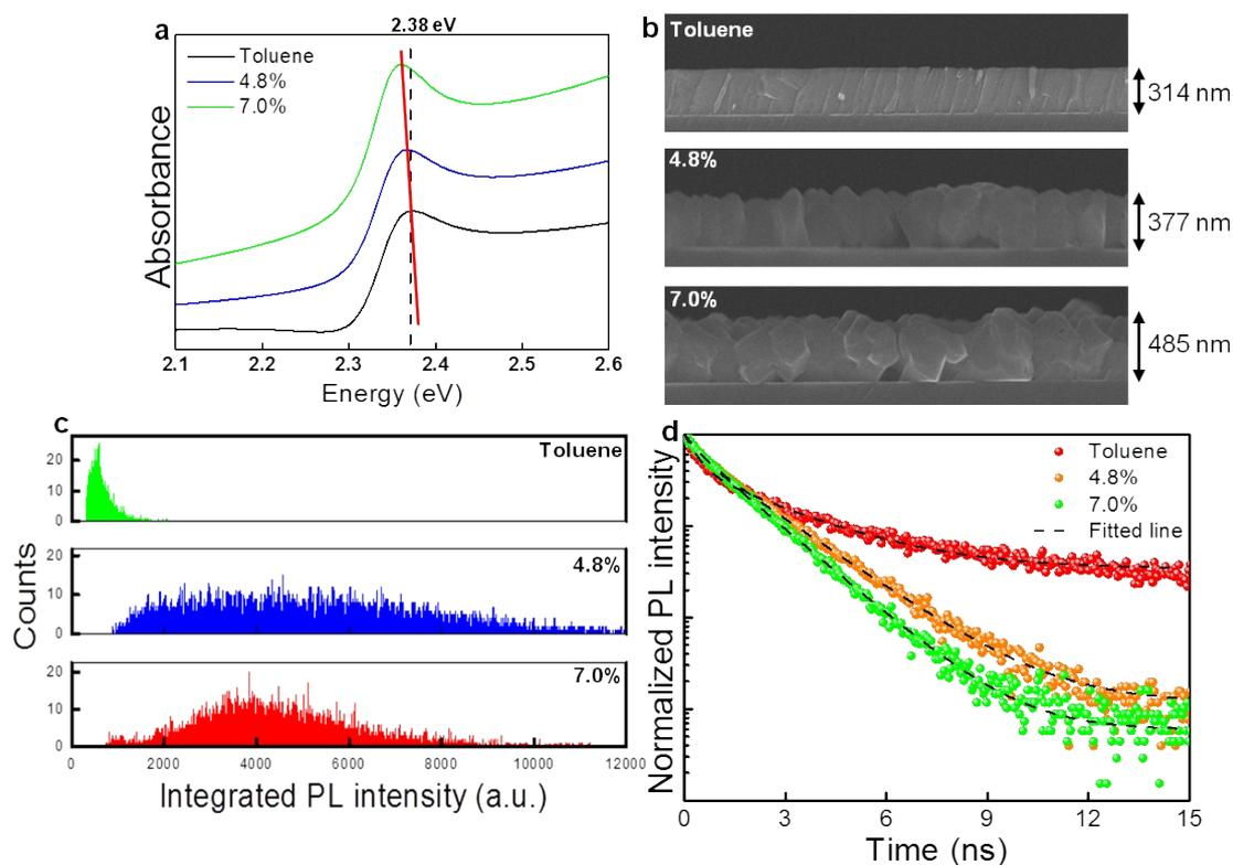
**Supplementary Figure S6.** a) Absorption spectra of MAPbBr<sub>3</sub> films formed by toluene and with seed concentrations of 4.8% and 7.0%. The dashed line indicates the exciton peak position for the film formed by toluene. The red line corresponds to the exciton peak position. b) Cross-sectional SEM images, c) integrated PL intensity histograms and d) TRPL spectra of the MAPbBr<sub>3</sub> films formed by toluene and with seed concentrations of 4.8% and 7.0%.
