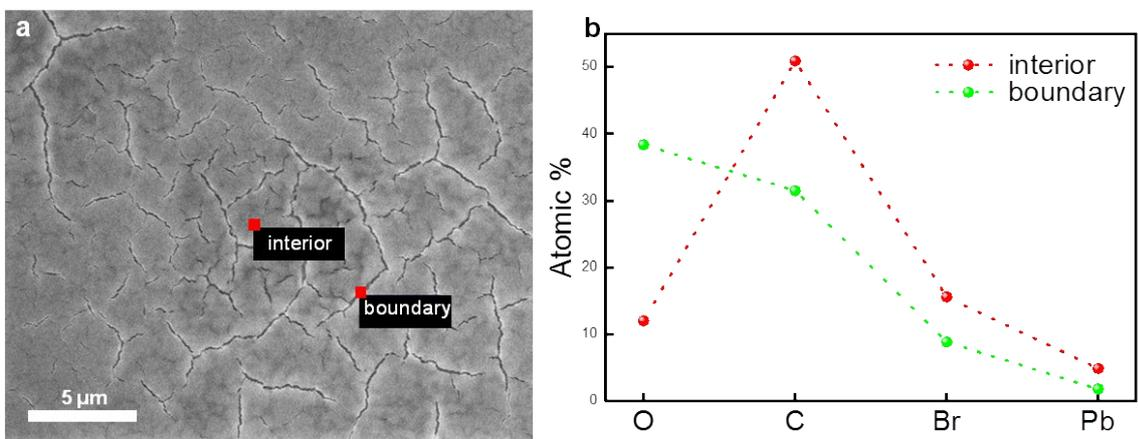
**Supplementary Figure S9.** a) SEM image of the film formed by toluene exposed to an electron beam for 2 min. b) Atomic percentage of O, C, Br, Pb in the interior and at the boundary (crack).
