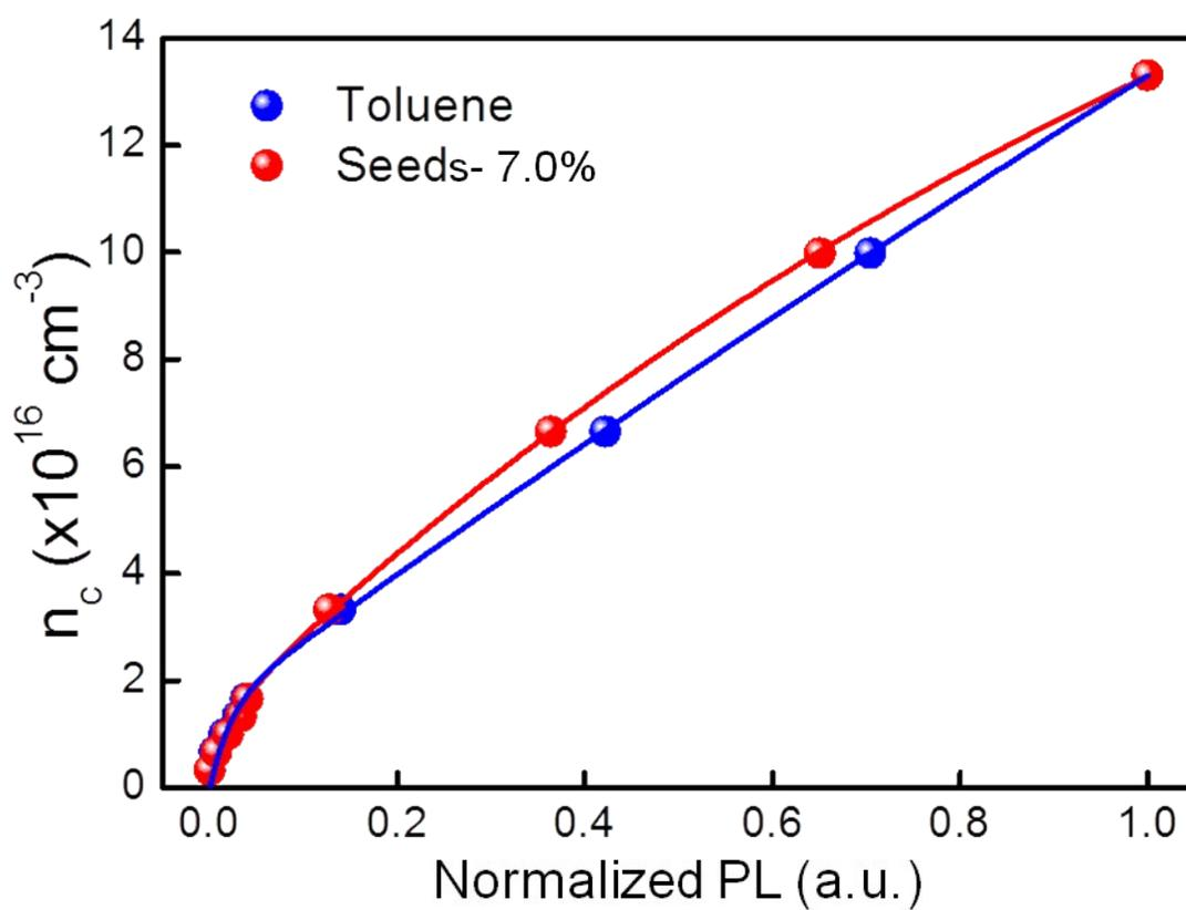
**Supplementary Figure S7.** Initial generated charge carrier density with respect to the normalized PL intensity measured via excitation-power-dependent PL.
