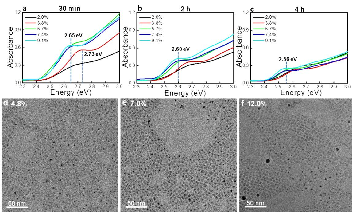
**Supplementary Figure S3.** UV–visible absorption spectra of the MAPbBr<sub>3</sub> QDs with the increasing concentration of the precursor solution after a) 30 min, b) 2 h, and c) 4 h. TEM image of the MAPbBr<sub>3</sub> QDs with a concentration of d) 4.8%, e) 7.0% and f) 12.0%.
