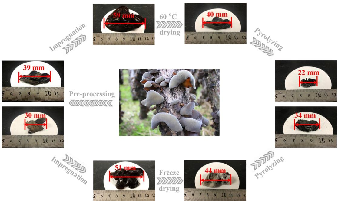
**Figure S1** The comparative digital photographs at different stages of the synthesis process of Mo<sub>2</sub>C@N-CANs electrocatalysts from natural agaric.
