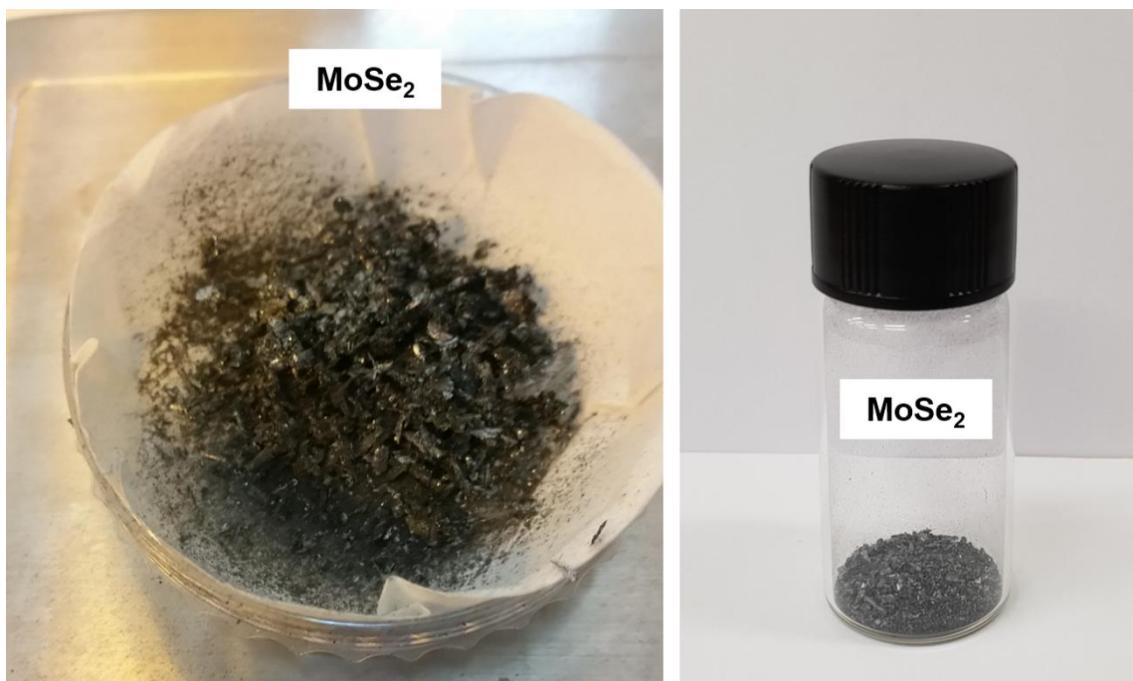
Fig. S13. Pictures of collected as-grown MoSe<sub>2</sub> nanosheets.
