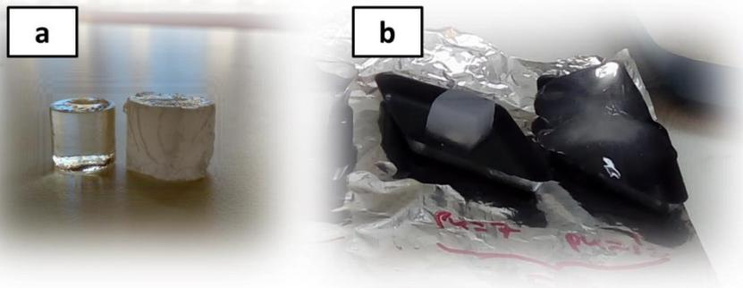
**Figure S6.** a) DAT hydrogel in the presence (left) and absence (right) of OEGMA and b) AM-free DAT hydrogel swollen in water (left) and SGF media (right)
