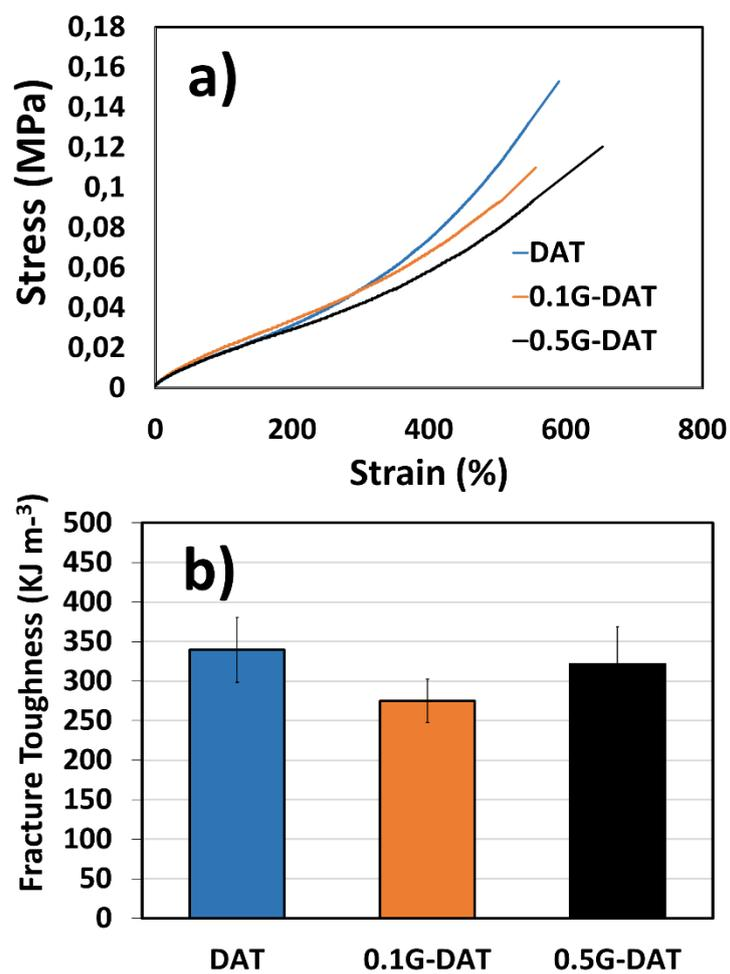
**Figure S7.** Tensile studies on (G)-DAT hydrogels: a) Stress-strain curve, b) Fracture toughness
