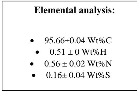
**Figure S3.** Characterization of graphene: Thermogravimetric Analysis, average Raman spectrum, TEM and lateral flake size images and elemental analysis.
