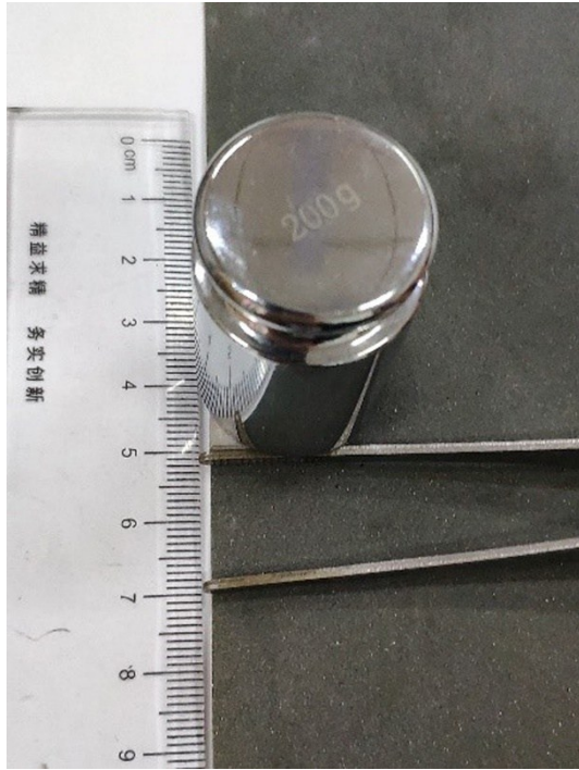
Figure S3. Scratched diagram of SHS and SLIPS for testing the thermally assisted healing property.
