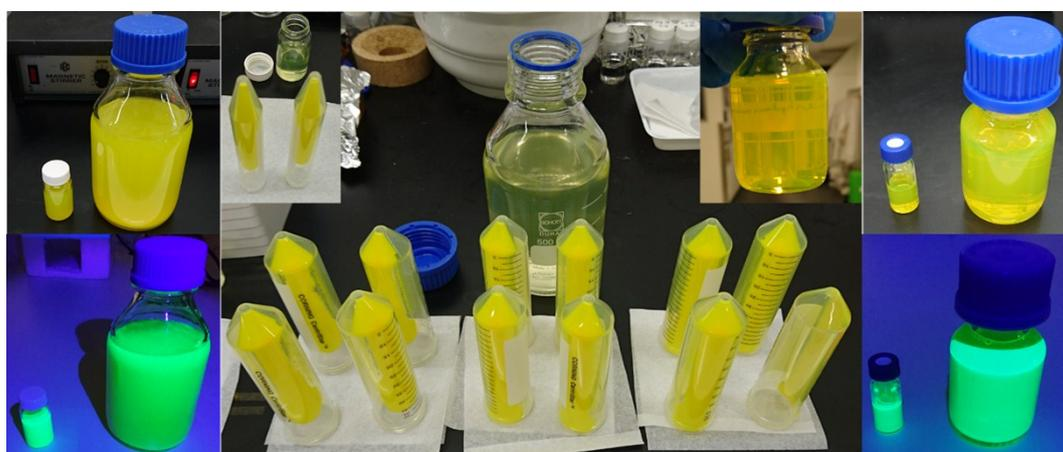
**Figure S25.** Small scale (left) and upscaled crude solutions under (a) ambient light and (b)  $\lambda = 365$  nm UV-light. Pellets and waste solvent after first centrifugation of (c) small scale and (d) upscaled reactions. (e) Purified CsPbBr<sub>3</sub> nanocrystal solution of upscaled reaction. Purified nanocrystal solutions of small scale (left) and upscaled (right) reactions under (f) ambient light and (g)  $\lambda = 365$  nm UV-light.
