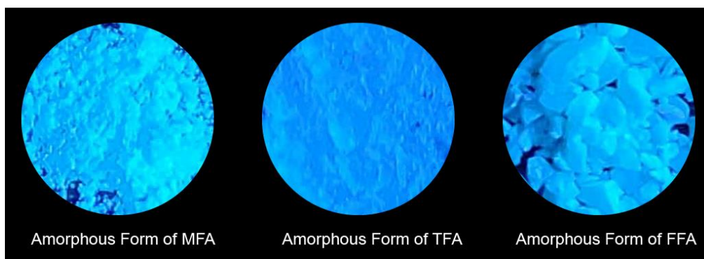
Figure S26 Fluorescent image of amorphous form of MFA , TFA and FFA under 365 nm UV illumination.
