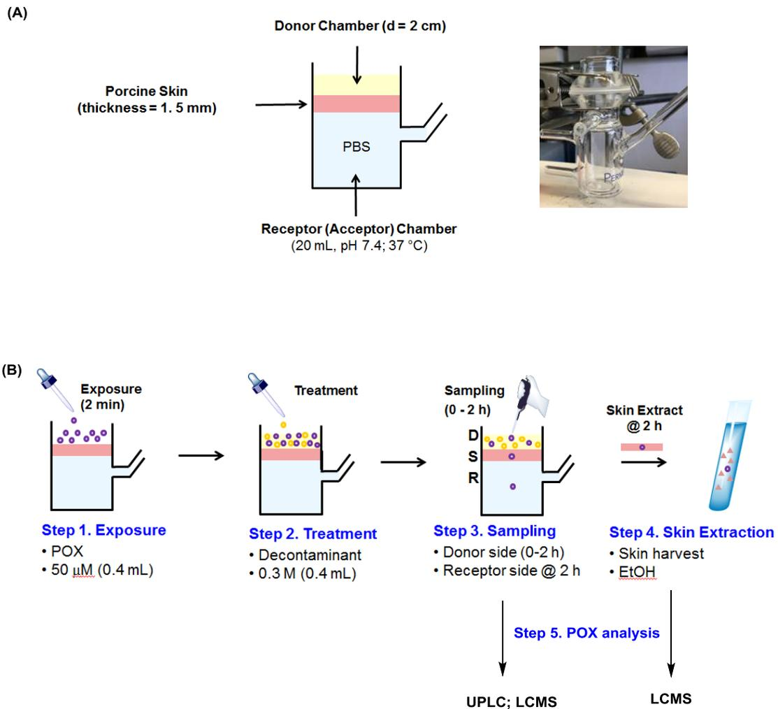
**Figure S7.** Schematic for POX decontamination using porcine skin in a Franz cell. (A) A photograph of a Franz cell, and (B) Process of POX decontamination and sample analysis. D = donor chamber; S = skin; R = receptor chamber
