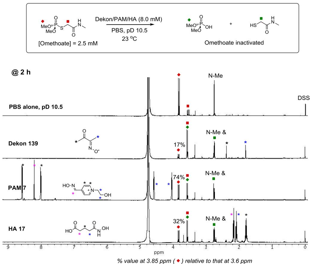
**Figure S3 (Continued).** <sup>1</sup>H NMR spectral traces of the hydrolysis of omethoate (2.5 mM) in a deuterated phosphate buffered saline (dPBS, pD 10.5) alone, or catalyzed by Dekon 139 (8.0 mM), **7** (8.0 mM), and **17** (8.0 mM), each in pD 10.5 at 23 °C after 2 h (E). The fraction (%) of omethoate intact was estimated by the integration of its signals for OMe groups.
