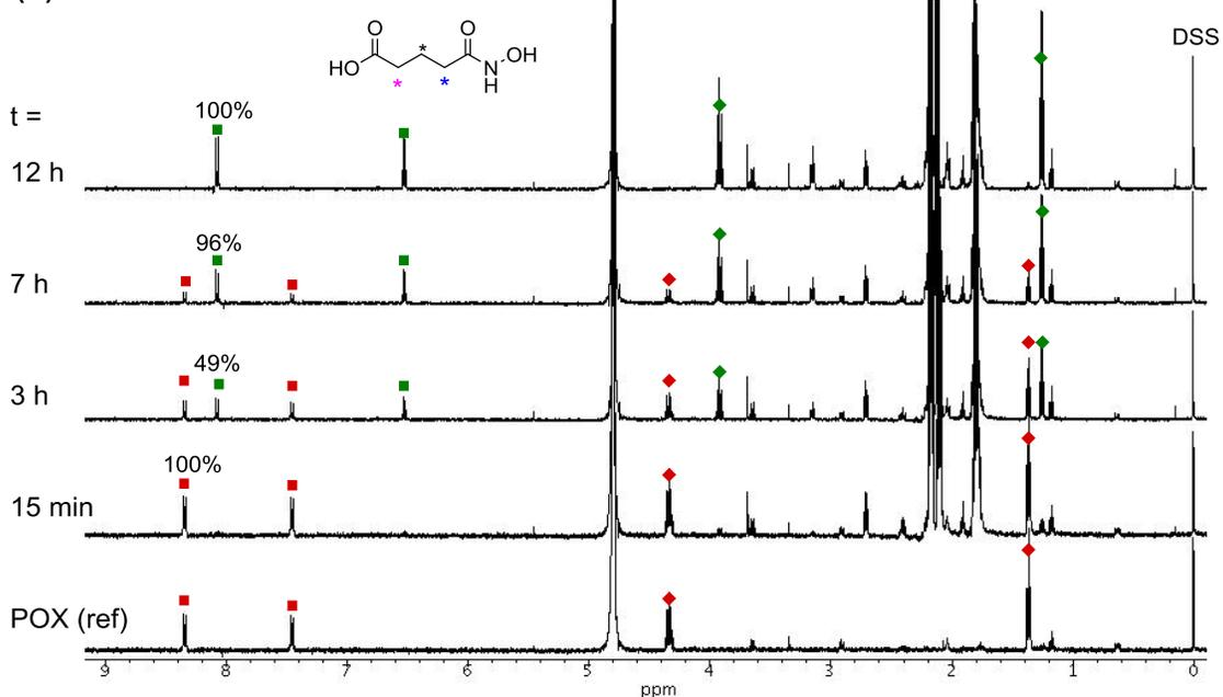
**Figure S3 (continued).** <sup>1</sup>H NMR spectral traces of the hydrolysis of POX (2.5 mM) in a deuterated phosphate buffered saline (dPBS, pD 10.5) catalyzed by **7** (8.0 mM; C), and **17** (8.0 mM; D), each in pD 10.5 at 23 °C. The fraction of POX hydrolysis is noted as the percentage value (%) as a function of incubation time.
