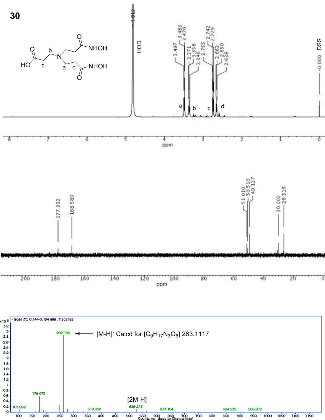
**Figure S1.** <sup>1</sup>H NMR (D<sub>2</sub>O, 500 MHz; top), <sup>13</sup>C NMR (100 MHz; middle) and HRMS spectra (bottom; negative ion mode) of **30**.
