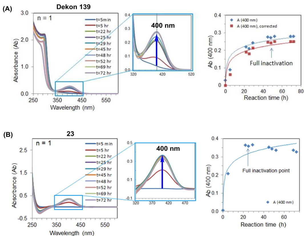
**Figure S4.** UV/vis spectral traces of POX inactivation. Paraoxon (POX; 30  $\mu\text{M}$ ) was incubated with Dekon 139 (4.0 mM; A) and **23** (4.0 mM; B) in PBS, pH 10.5 at 37  $^\circ\text{C}$ .
