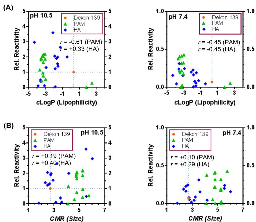
**Figure S5.** Plots of compound reactivity versus its lipophilicity ( $c\log P$ ) (A) and calculated molar refractivity (CMR) (B). Relative reactivity refers to the ratio of  $k_1(\text{test compound})/k_1(\text{Dekon 139, pH 10.5})$ .  $r$  = correlation coefficient (Pearson)
