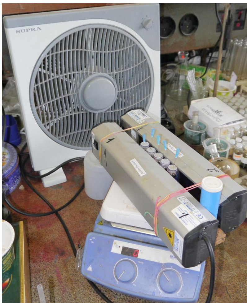
Figure S2. Photochemical reactors, used in our work.
