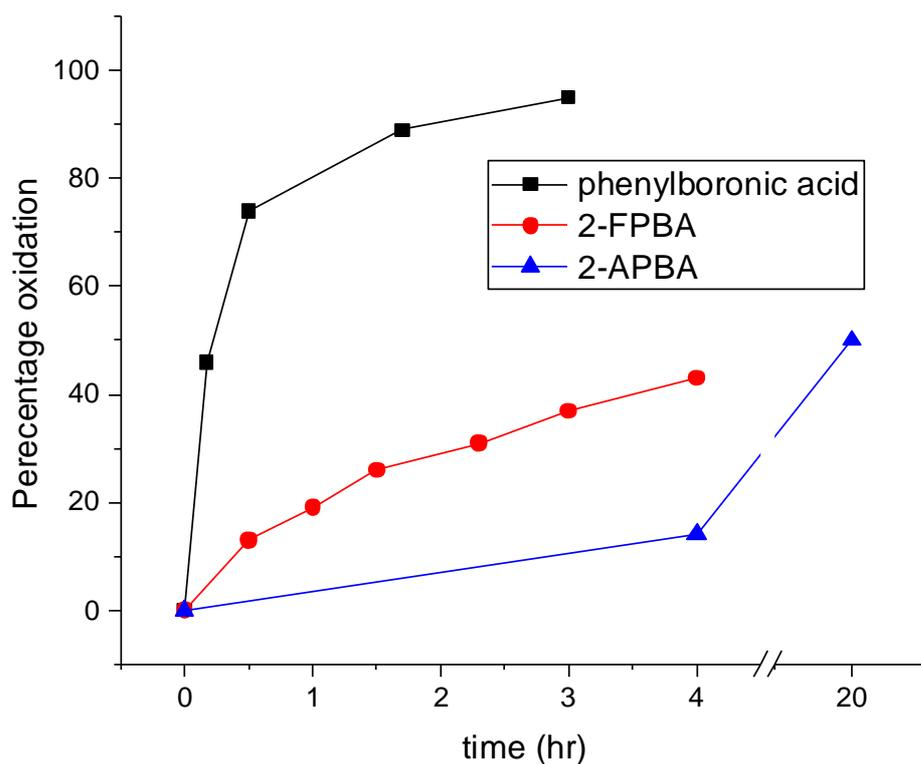
**Figure S5.** Oxidation kinetics of 2-APBA/FPBA in comparison to that of phenylboronic acid. Based on these results, the apparent half-lives of phenylboronic acid, 2-FPBA, and 2-APBA are estimated to be 0.5 hr, 4 hrs and 20 hrs respectively.
