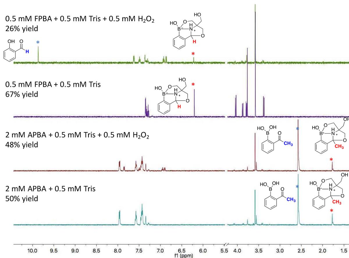
**Figure S6.** Tris conjugation with 2-APBA or 2-FPBA in the presence of H<sub>2</sub>O<sub>2</sub>. All reactions were allowed to incubate in a phosphate buffer (pH 7.4) for 20 hrs before the <sup>1</sup>H-NMR spectra were recorded.
