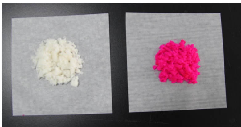
Fig. S1. The prepared supported catalyst: (1) the benzyltriethylammonium chloride functionalized Merrifield resin (left); (2) The supported Rose Bengal ammonium salt (right).
