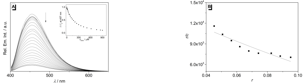
Figure S1. A: Fluorimetric titration of 2c with ct DNA ( c = 1.0 mM in base pairs) in K-phosphate buffer (pH = 7.0, 5% v/v DMSO), T = 20 °C; \lambda_{\text{ex}} = 342 nm. The arrows indicate the development of the emission bands during the titration. Inset: Plot of relative emission intensity I / I_0 versus c_{\text{DNA}} . B: Corresponding Scatchard plot of r / c versus r and fit of the experimental data to the theoretical model (eq. S3).
