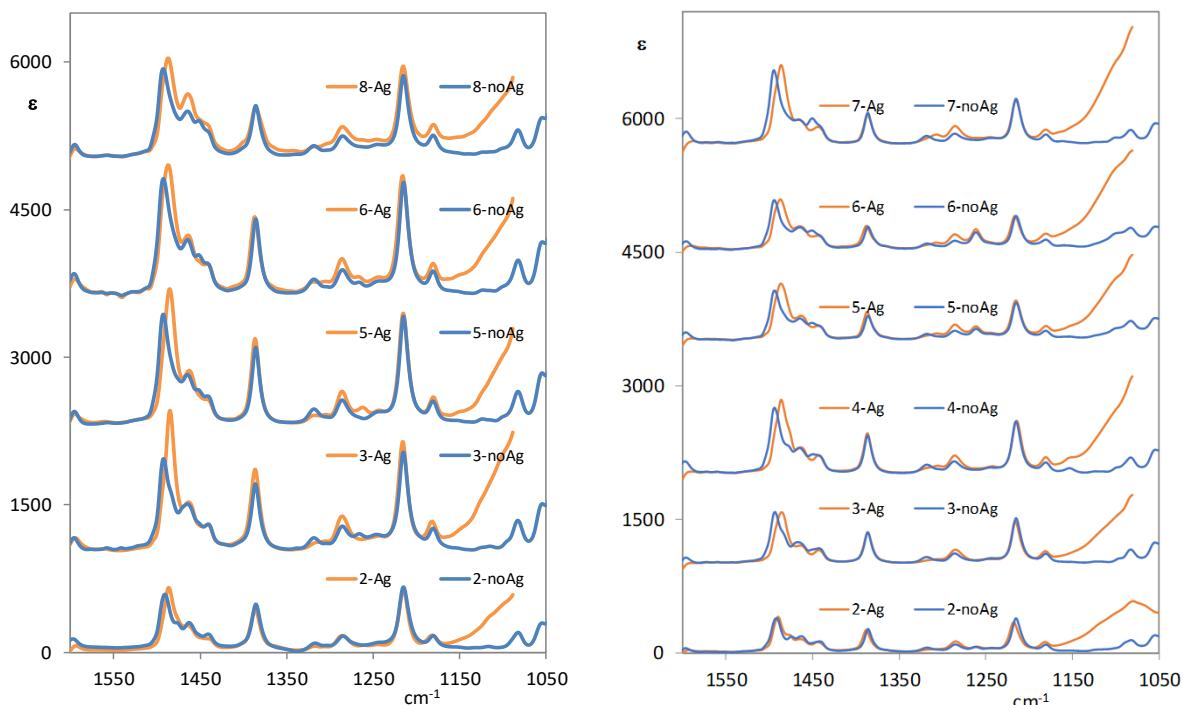
**Figure S63.** Superposition of VCD spectra of monosulfoxide (*S*)-**2**(two CC triple bonds) and disulfoxide (*S,S*)-**3**(three CC triple bonds)<sup>52</sup> after normalization of the corresponding absorption spectra
