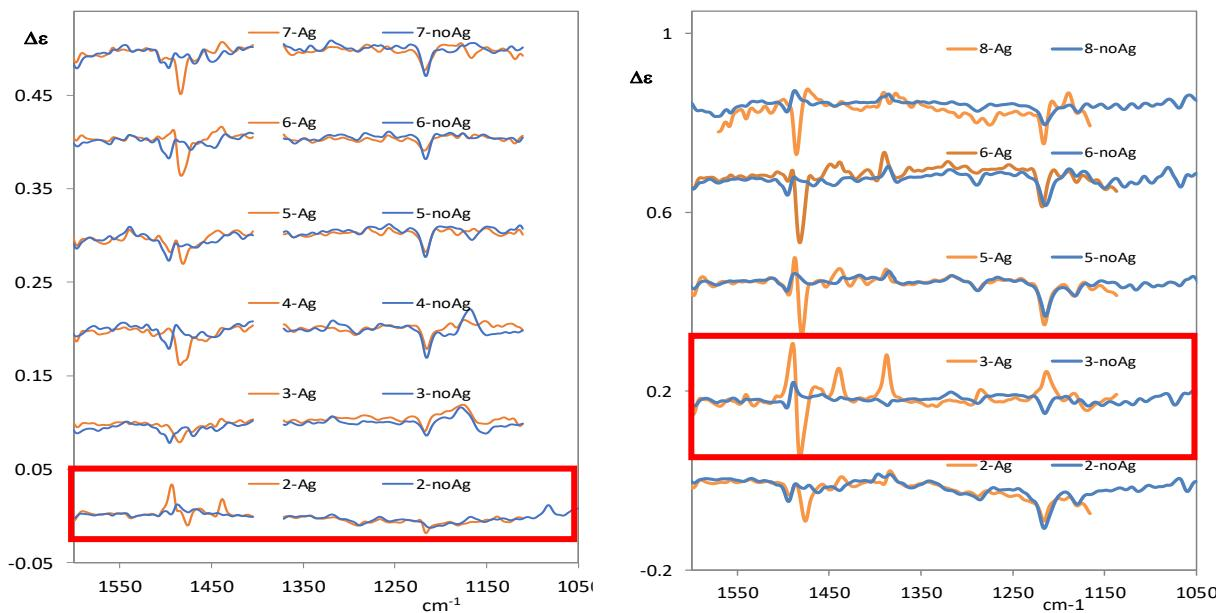
**Figure S62.** IR spectra of monosulfoxides of the present work (left), and disulfoxides of previous work<sup>S2</sup> (right). The number of the compounds indicates also the number of triple bonds.
