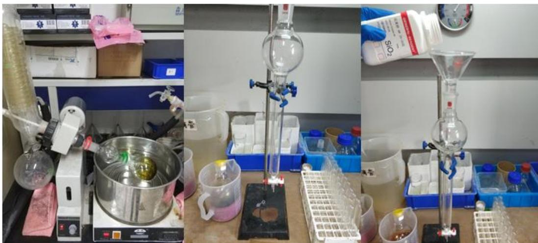
(Left) Concentration of the solvent; (Center) Addition of cotton to the bottom of the glass column; (Right) addition of a small amount of quartz sand.
