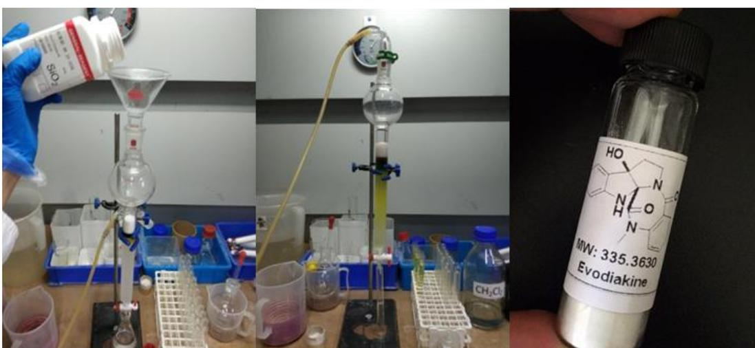
(Left) Addition of quartz sand; (Center) Purified by chromatography on silica gel ( $\text{CH}_2\text{Cl}_2/\text{MeOH} = 100:1$ ); (Right) Evodiakine obtained after column chromatography.
