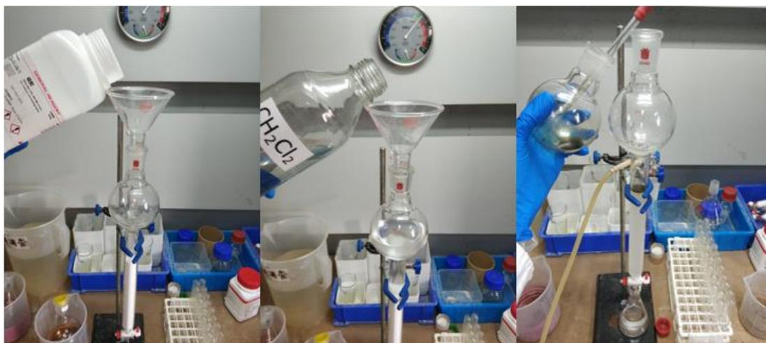
(Left) Addition of silica gel; (Center)  $\text{CH}_2\text{Cl}_2$  was pouring into the column; (Right) Addition of the crude mixture.
