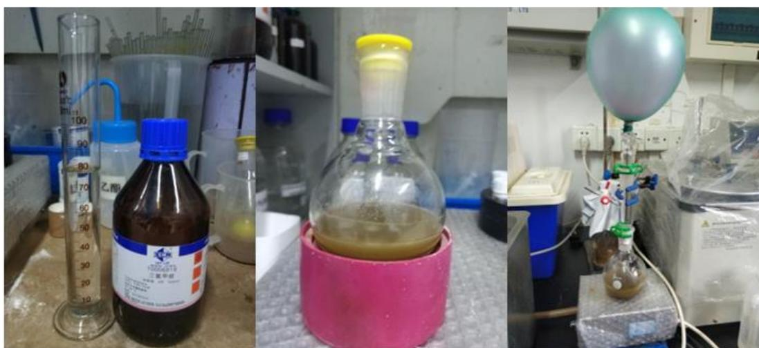
(Left)  $\text{CHCl}_3$  (150 mL); (Center) Dissolved in solvent; (Right) Oxygen replace air.
