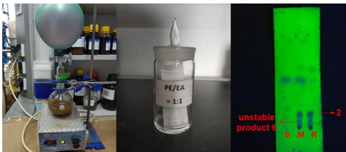
(Left) Stirred at r.t. for 2 h; (Center) Reaction progress was monitored by TLC; (Right) TLC under UV (PE/EtOAc = 1 : 1).
