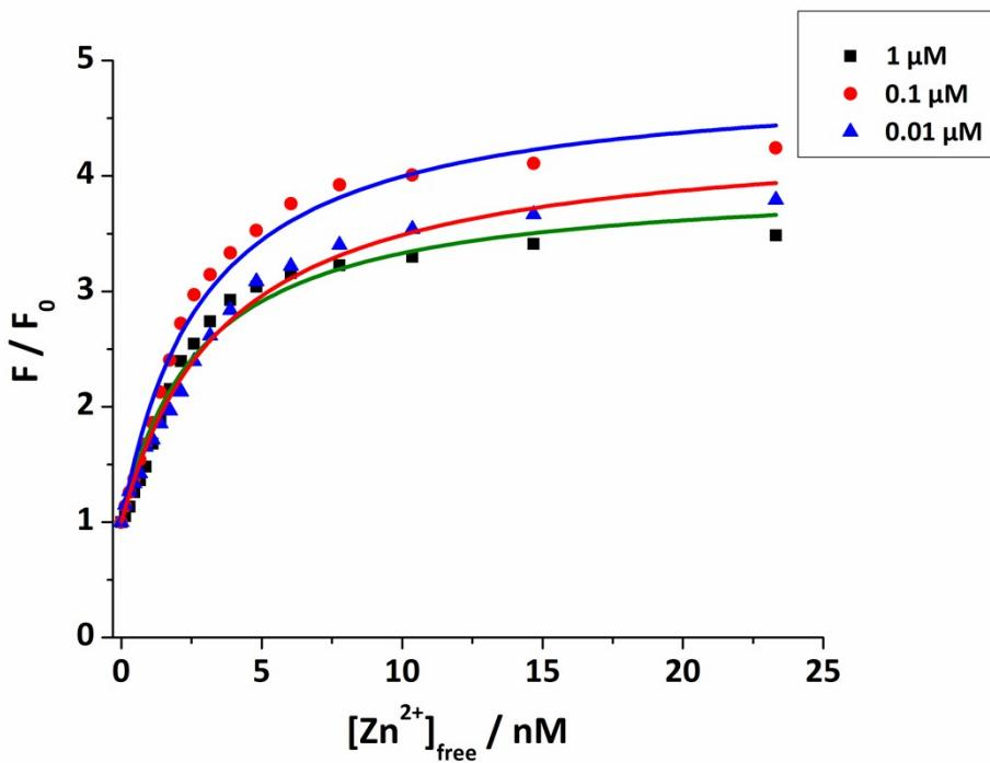
Fig. S14 The non-linear curve fitting of the fluorescence intensity of **9** at different concentrations against  $[Zn^{2+}]_{\text{free}}$  applying Equation S1. ( $\lambda_{\text{ex}} = 346 \text{ nm}$ ,  $\lambda_{\text{em}} = 414 \text{ nm}$ )
