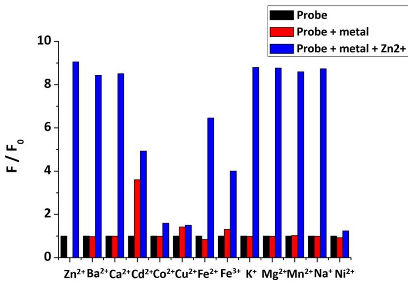
Fig. S31 Metal ion selectivity of **8**. Average normalized fluorescence intensities for **8** (50  $\mu\text{M}$ ) (black bars), after addition of 5 equivalents of various cations (red bars), followed by addition of 1 equivalent of  $\text{ZnCl}_2$  (blue bars).
