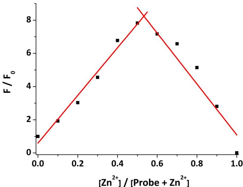
Fig. S10 The Job's plot to determine the stoichiometry of the complex formed between **9** and Zn<sup>2+</sup>. The total amount of [Probe + Zn<sup>2+</sup>] was 100 μM, ( $\lambda_{\text{ex}} = 346$  nm,  $\lambda_{\text{em}} = 414$  nm, slit width: 5/2.5 nm)
