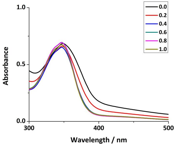
Fig. S1 The UV-Vis spectra of **7** (50  $\mu\text{M}$ ) and its complex with different equivalents of  $\text{Zn}^{2+}$ .
