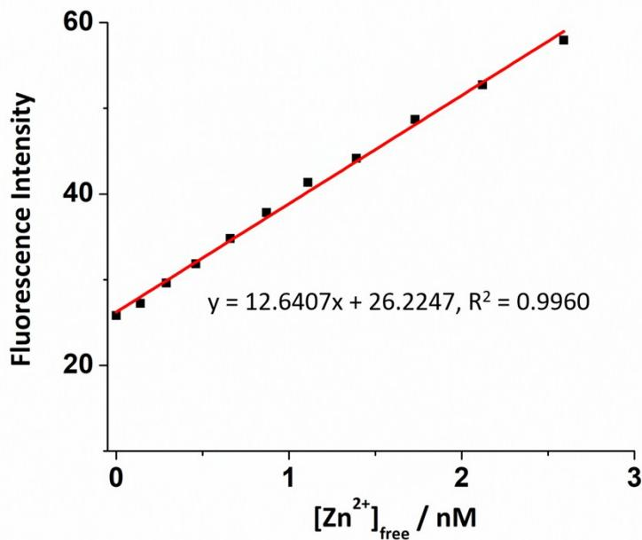
Fig. S17 Fluorescence response of **8** (1  $\mu\text{M}$ ) against  $[\text{Zn}^{2+}]_{\text{free}}$ . ( $\lambda_{\text{ex}} = 346 \text{ nm}$ ,  $\lambda_{\text{em}} = 414 \text{ nm}$ , slit width: 5/5 nm)
