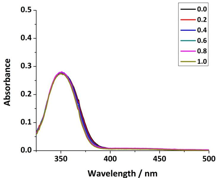
Fig. S2 The UV-Vis spectra of **8** (50  $\mu\text{M}$ ) and its complex with different equivalents of  $\text{Zn}^{2+}$ .
