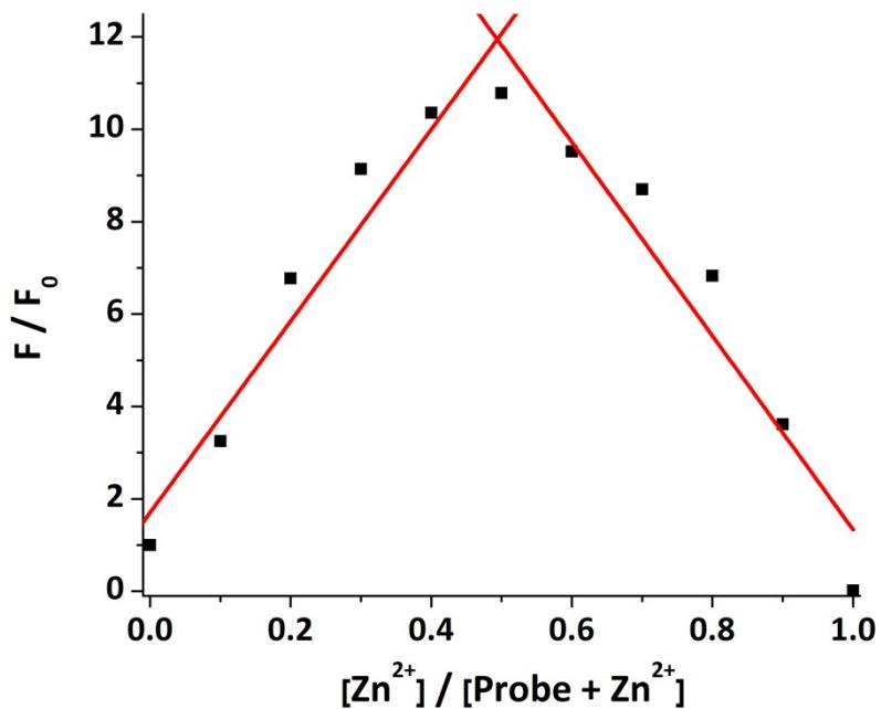
Fig. S8 The Job's plot to determine the stoichiometry of the complex formed between **7** and  $\text{Zn}^{2+}$ . The total amount of  $[\text{Probe} + \text{Zn}^{2+}]$  was 100  $\mu\text{M}$ , ( $\lambda_{\text{ex}} = 346 \text{ nm}$ ,  $\lambda_{\text{em}} = 414 \text{ nm}$ , slit width: 5/2.5 nm)
