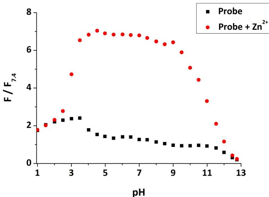
Fig. S24 The pH profile of **8** (50 μM, black dots) and its complex with 1 equivalent of Zn<sup>2+</sup> (red dots). ( $\lambda_{\text{ex}} = 346$  nm, slit width: 5/2.5 nm)
