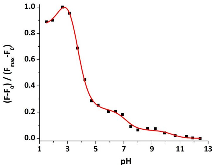
Fig. S27 Normalized integrated fluorescence emission of **7** (50 μM) vs pH, the nonlinear curve fitting used to determine the apparent pK<sub>a</sub> values applying Equation S3. The determined pK<sub>a</sub> values are: pK<sub>a1</sub> = 2.65 ± 0.26, pK<sub>a2</sub> = 3.62 ± 0.09, pK<sub>a3</sub> = 7.13 ± 0.17, pK<sub>a4</sub> = 10.42 ± 0.41, R<sup>2</sup> = 99.83%.
