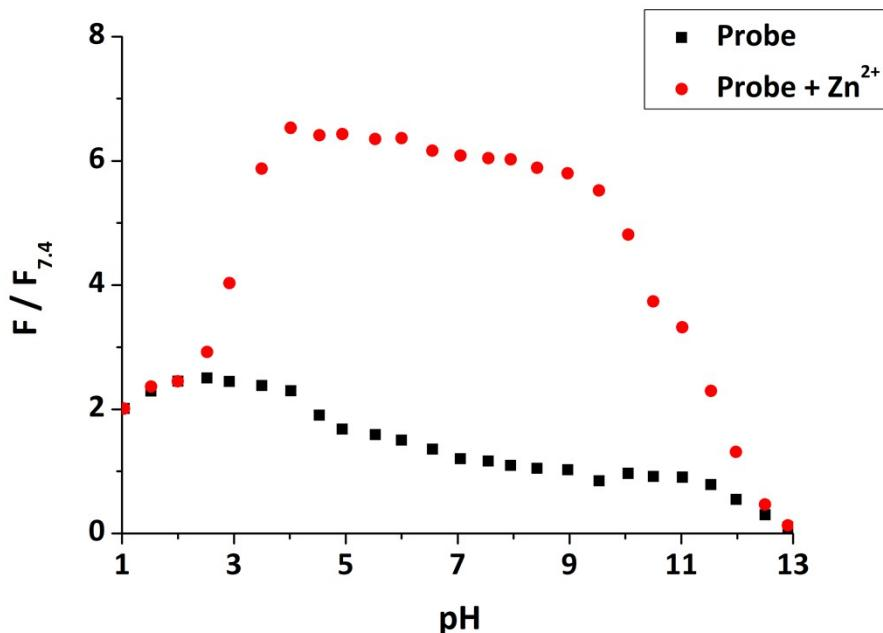
Fig. S25 The pH profile of **9** (50  $\mu\text{M}$ , black dots) and its complex with 1 equivalent of Zn<sup>2+</sup> (red dots). ( $\lambda_{\text{ex}} = 346 \text{ nm}$ , slit width: 5/2.5 nm)
