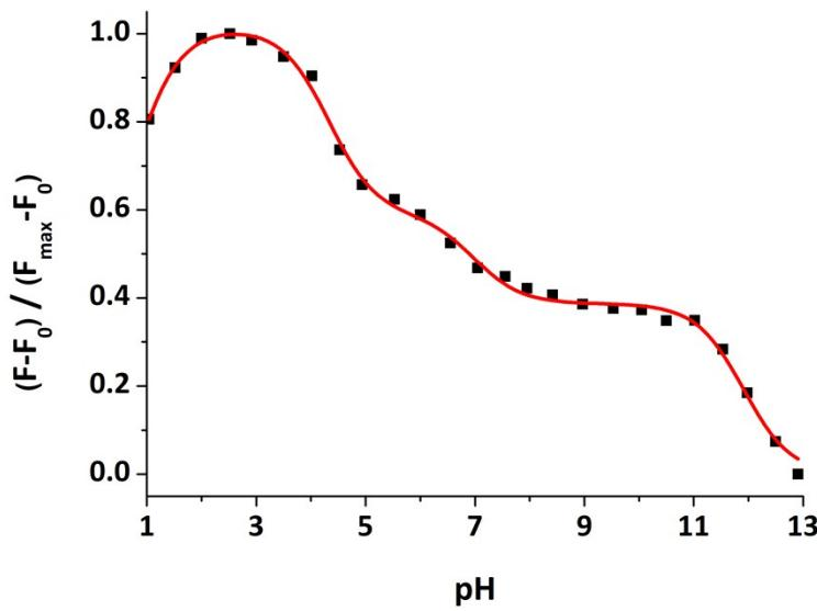
Fig. S29 Normalized integrated fluorescence emission of **9** (50  $\mu\text{M}$ ) vs pH, the nonlinear curve fitting used to determine the apparent  $\text{p}K_a$  values applying Equation S3. The determined  $\text{p}K_a$  values are:  $\text{p}K_{a1} = 0.70 \pm 0.38$ ,  $\text{p}K_{a2} = 4.33 \pm 0.08$ ,  $\text{p}K_{a3} = 6.99 \pm 0.15$ ,  $\text{p}K_{a4} = 11.91 \pm 0.06$ ,  $R^2 = 99.64\%$ .
