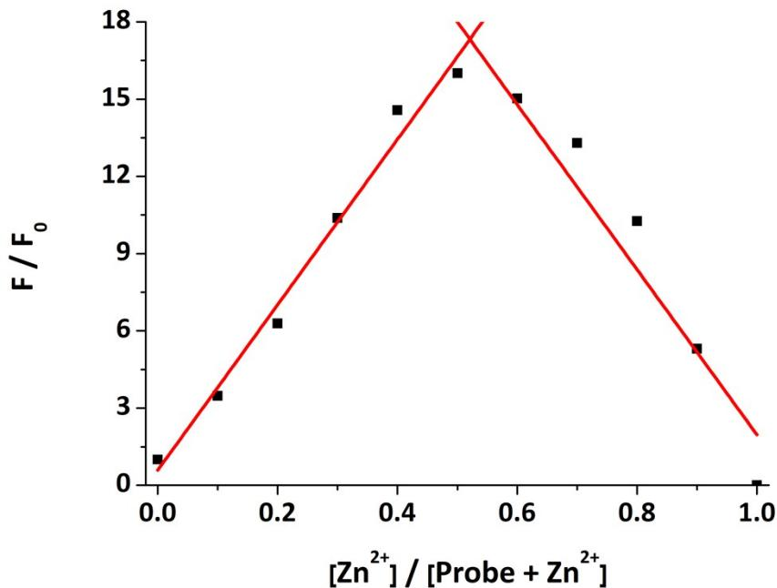
Fig. S11 The Job's plot to determine the stoichiometry of the complex formed between **10** and  $Zn^{2+}$ . The total amount of  $[\text{Probe} + Zn^{2+}]$  was 100  $\mu\text{M}$ , ( $\lambda_{\text{ex}} = 346 \text{ nm}$ ,  $\lambda_{\text{em}} = 414 \text{ nm}$ , slit width: 5/2.5 nm)
