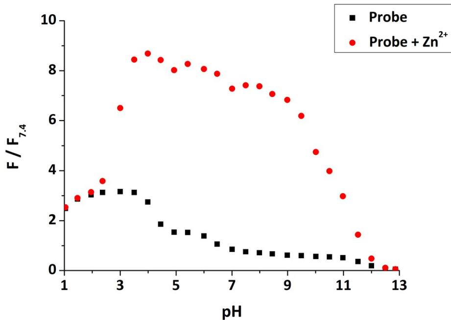
Fig. S26 The pH profile of **10** (50  $\mu\text{M}$ , black dots) and its complex with 1 equivalent of Zn<sup>2+</sup> (red dots). ( $\lambda_{\text{ex}} = 346 \text{ nm}$ , slit width: 5/2.5 nm)
