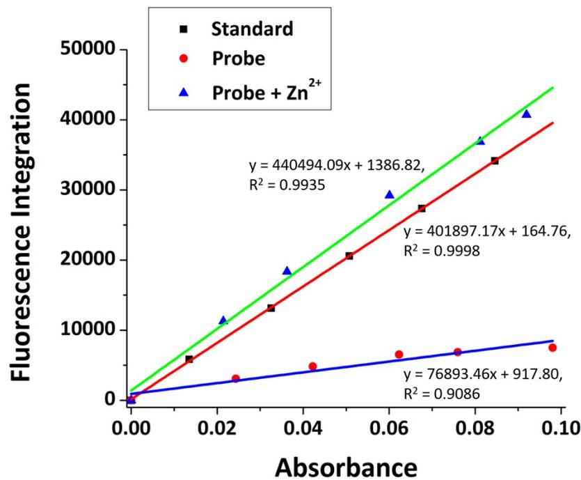
Fig. S20 Linear plots for standard sample, 7, and 7 + Zn<sup>2+</sup> to obtain quantum yields. ( $\lambda_{\text{ex}} = 346 \text{ nm}$ , slit width: 5/2.5 nm)
