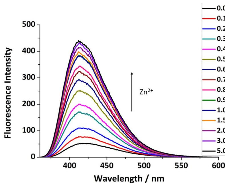
Fig. S6 The fluorescence response of **9** (50  $\mu\text{M}$ ) to different equivalents of  $\text{Zn}^{2+}$ . ( $\lambda_{\text{ex}} = 346 \text{ nm}$ , slit width: 5/2.5 nm)
