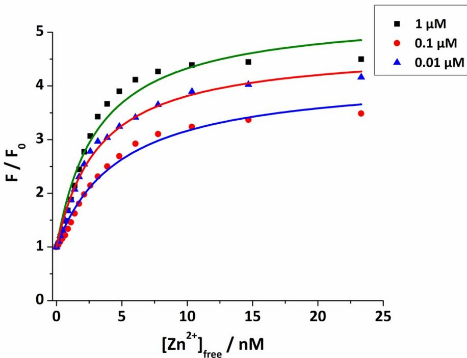
Fig. S15 The non-linear curve fitting of the fluorescence intensity of **10** at different concentrations against  $[Zn^{2+}]_{\text{free}}$  applying Equation S1. ( $\lambda_{\text{ex}} = 346 \text{ nm}$ ,  $\lambda_{\text{em}} = 414 \text{ nm}$ )
