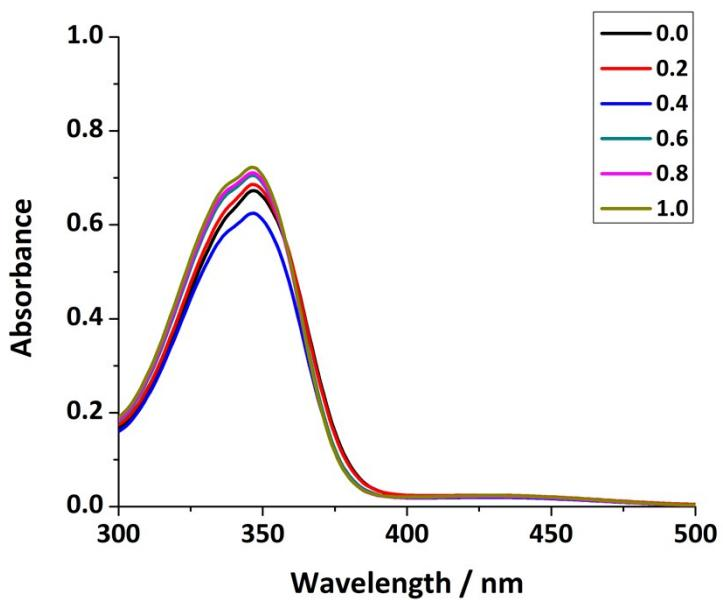
Fig. S3 The UV-Vis spectra of **9** (50  $\mu\text{M}$ ) and its complex with different equivalents of  $\text{Zn}^{2+}$ .
