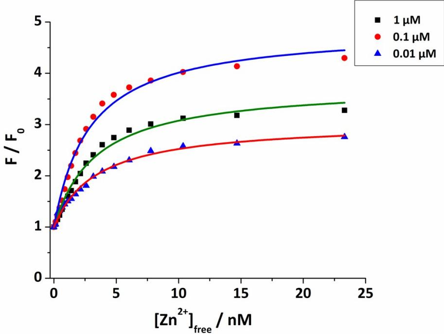
Fig. S13 The non-linear curve fitting of the fluorescence intensity of **8** at different concentrations against  $[Zn^{2+}]_{\text{free}}$  applying Equation S1. ( $\lambda_{\text{ex}} = 346 \text{ nm}$ ,  $\lambda_{\text{em}} = 414 \text{ nm}$ )
