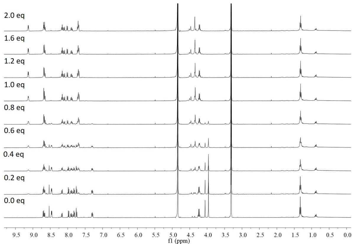
Fig. S34 <sup>1</sup>H NMR titration spectra (whole range) of probe **10** (5 mM) with different equivalents ZnCl<sub>2</sub> in CD<sub>3</sub>OD.
