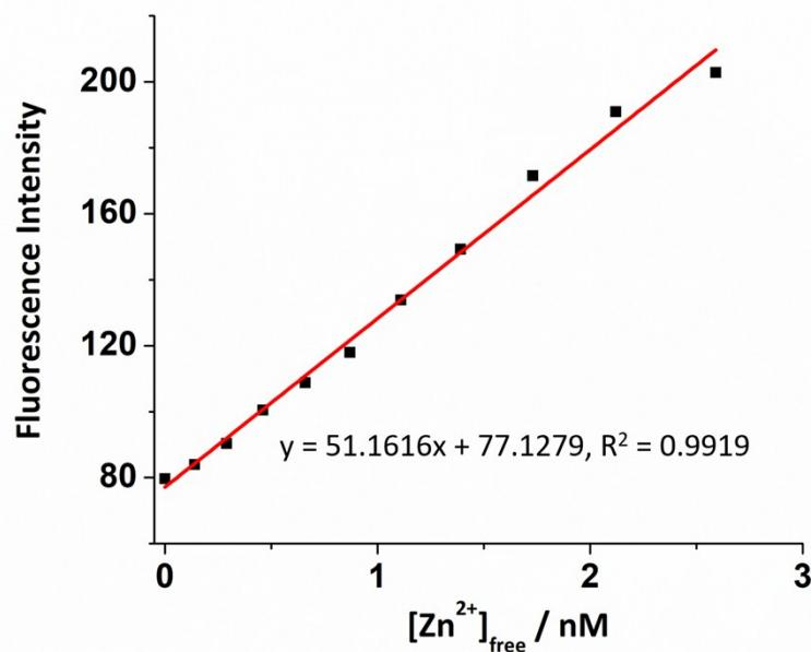
Fig. S18 Fluorescence response of **9** (1  $\mu\text{M}$ ) against  $[\text{Zn}^{2+}]_{\text{free}}$ . ( $\lambda_{\text{ex}} = 346 \text{ nm}$ ,  $\lambda_{\text{em}} = 414 \text{ nm}$ , slit width: 5/5 nm)
