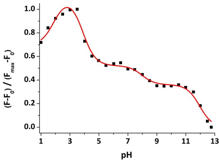
Fig. S28 Normalized integrated fluorescence emission of **8** (50  $\mu\text{M}$ ) vs pH, the nonlinear curve fitting used to determine the apparent  $\text{p}K_a$  values applying Equation S3. The determined  $\text{p}K_a$  values are:  $\text{p}K_{a1} = 1.91 \pm 0.27$ ,  $\text{p}K_{a2} = 3.88 \pm 0.13$ ,  $\text{p}K_{a3} = 7.97 \pm 0.32$ ,  $\text{p}K_{a4} = 11.95 \pm 0.12$ ,  $R^2 = 98.57\%$ .
