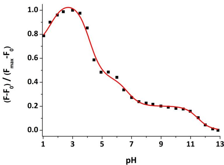
Fig. S30 Normalized integrated fluorescence emission of **10** (50  $\mu\text{M}$ ) vs pH, the nonlinear curve fitting used to determine the apparent  $\text{p}K_a$  values applying Equation S3. The determined  $\text{p}K_a$  values are:  $\text{p}K_{a1} = 1.53 \pm 0.29$ ,  $\text{p}K_{a2} = 6.73 \pm 0.21$ ,  $\text{p}K_{a3} = 4.14 \pm 0.10$ ,  $\text{p}K_{a4} = 11.50 \pm 0.17$ ,  $R^2 = 99.39\%$ .
