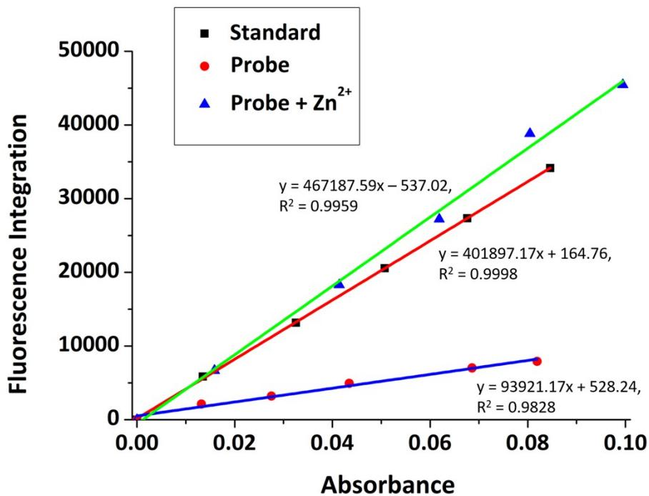
Fig. S21 Linear plots for standard sample, 8, and 8 + Zn<sup>2+</sup> to obtain quantum yields. ( $\lambda_{\text{ex}} = 346 \text{ nm}$ , slit width: 5/2.5 nm)
