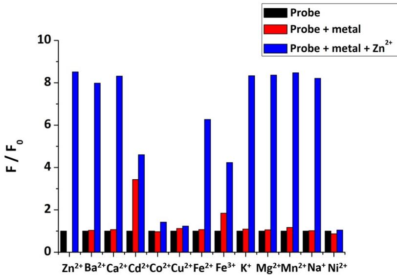
Fig. S32 Metal ion selectivity of **9**. Average normalized fluorescence intensities for **9** (50  $\mu$ M) (black bars), after addition of 5 equivalents of various cations (red bars), followed by addition of 1 equivalent of  $ZnCl_2$  (blue bars).
