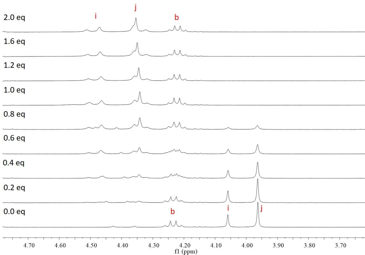
Fig. S35 <sup>1</sup>H NMR titration spectra (range 3.70 - 4.70 ppm) of probe **10** (5 mM) with different equivalents  $\text{ZnCl}_2$  in  $\text{CD}_3\text{OD}$ .
