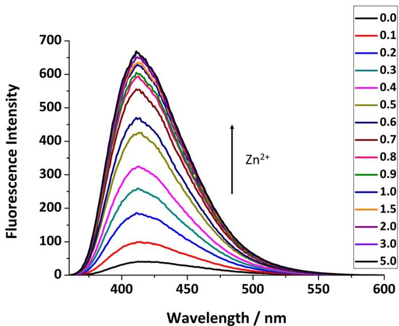
Fig. S7 The fluorescence response of **10** (50  $\mu\text{M}$ ) to different equivalents of  $\text{Zn}^{2+}$ . ( $\lambda_{\text{ex}} = 346 \text{ nm}$ , slit width: 5/2.5 nm)
