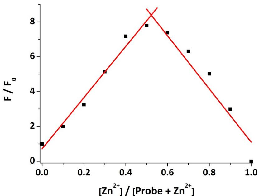
Fig. S9 The Job's plot to determine the stoichiometry of the complex formed between **8** and Zn<sup>2+</sup>. The total amount of [Probe + Zn<sup>2+</sup>] was 100 μM, ( $\lambda_{\text{ex}} = 346$  nm,  $\lambda_{\text{em}} = 414$  nm, slit width: 5/2.5 nm)
