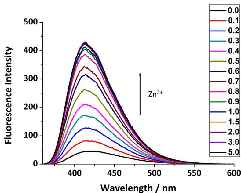
Fig. S5 The fluorescence response of **8** (50  $\mu\text{M}$ ) to different equivalents of  $\text{Zn}^{2+}$ . ( $\lambda_{\text{ex}} = 346 \text{ nm}$ , slit width: 5/2.5 nm)
