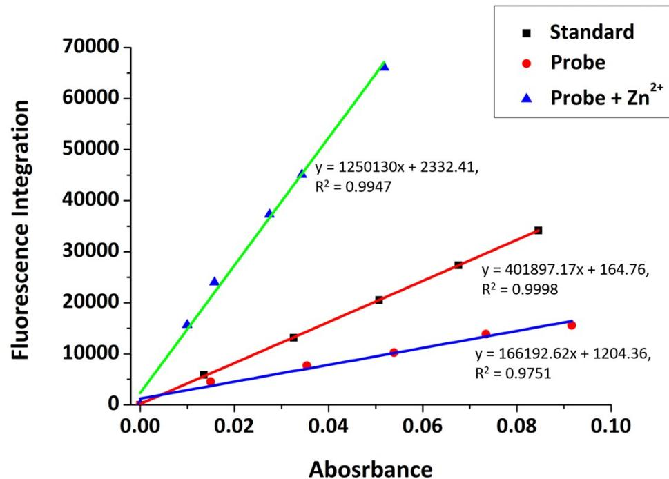
Fig. S23 Linear plots for standard sample, **10**, and **10** + Zn<sup>2+</sup> to obtain quantum yields. ( $\lambda_{\text{ex}} = 346$  nm, slit width: 5/2.5 nm)
